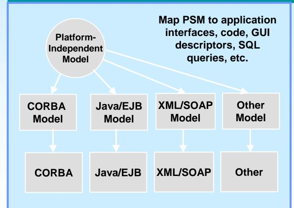
MDA Tool generates all or most of the implementation code for deployment technology selected by the developer.
