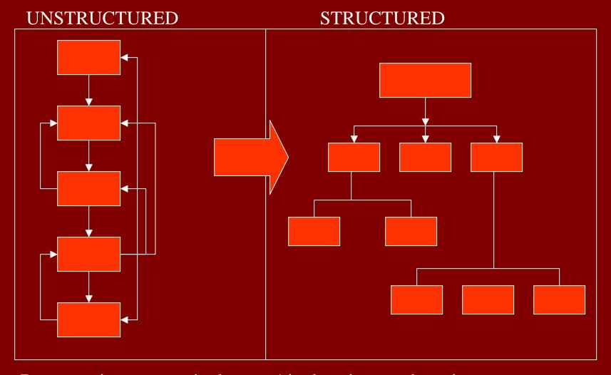
Restructuring creates single entry/single exit procedures in a program, isolates I/O logic and generally prepares a system for modularization.
