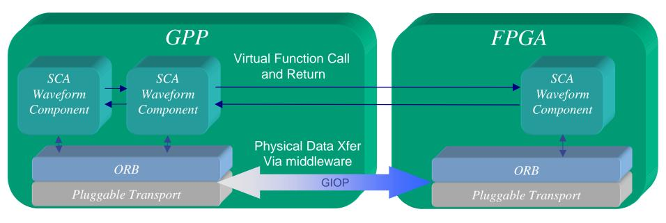
For System on a Chip (SoC) solutions, both the embedded processor and off-board processors can communicate, via an ORB with waveform components implemented in hardware; thus, SCA compliance is maintained.
