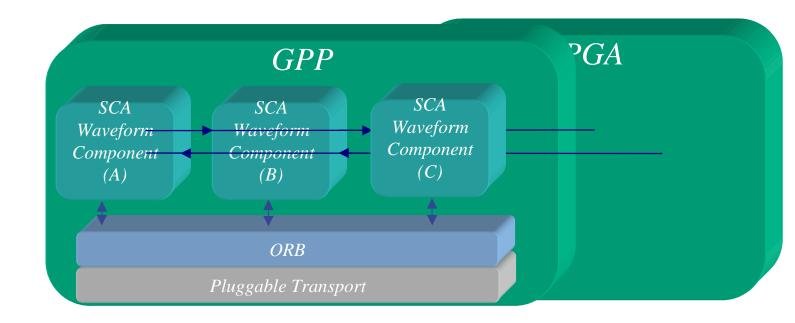
Attempts to implement this resulted in non-SCA compliant components in the FPGA and added complexity for the radio developer
