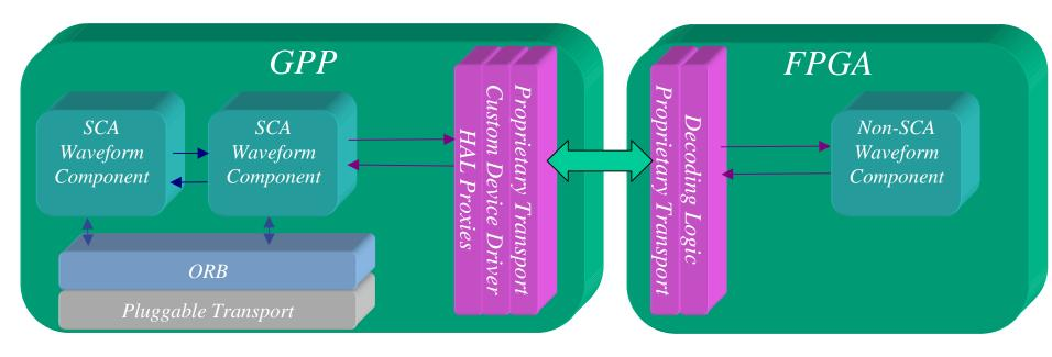
Other attempts to implement this have only moved the problem internal to the FPGA. The result is still non-SCA compliant components in the FPGA and a likley increase in added transport overhead
