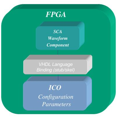
The embedded waveform logic is then connected to the ICO Wrapper which contains the VHDL SCA waveform component
