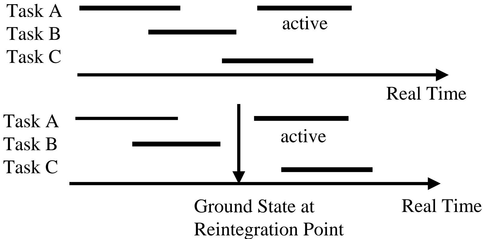
**g-state:** Minimal h-state of a subsystem (node) where all tasks are inactive and all channels are flushed. Needed for reintegration of nodes.
