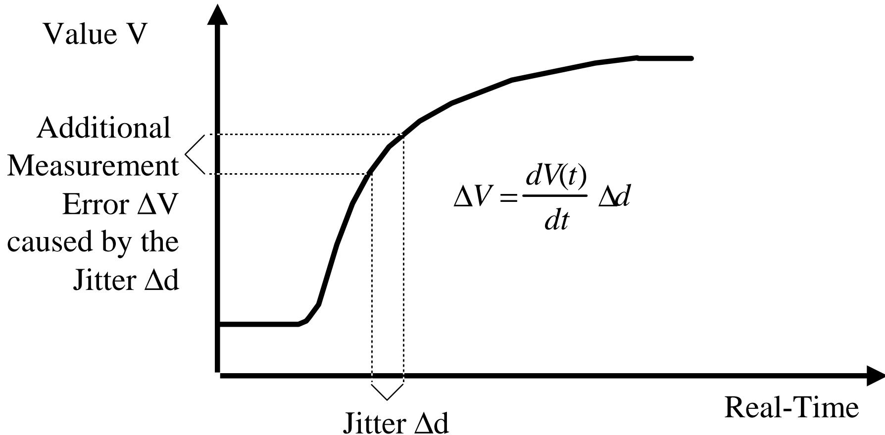
**Jitter in Control Loops causes a degradation of control quality.**
