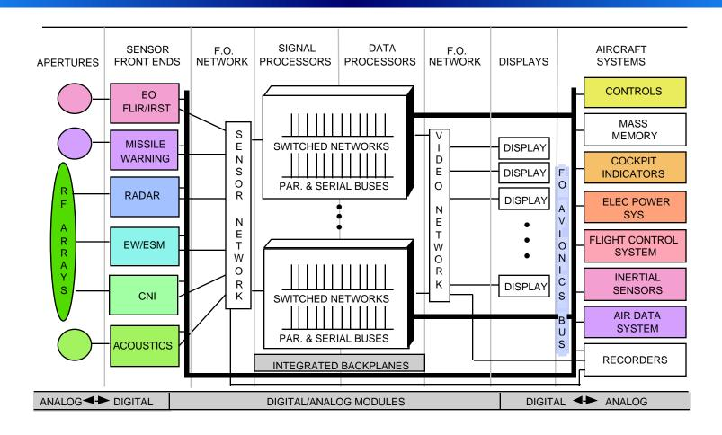
This architecture is taken from the Joint Advanced Strike Technology Program Avionics Architecture Definition, Version 1.0 dated 9 August 1994
