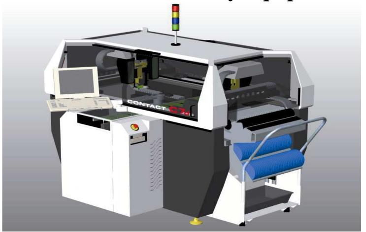
Machines that combine high speed and precise positioning and placement of devices onto printed circuit boards
