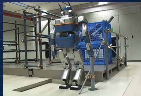
walk up stairs holding on to the railing
