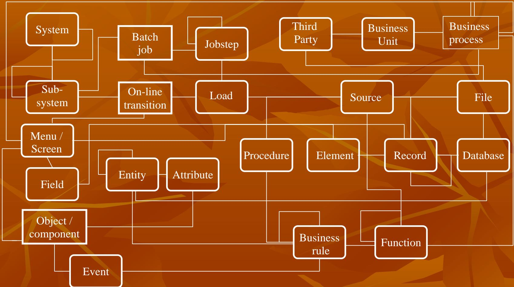
Project-level repository facilitates tracking of business data and rules back to physical system components and target requirements.
