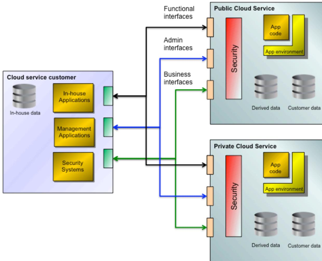
**Figure 3: Components and connections for Hybrid Cloud Computing**
