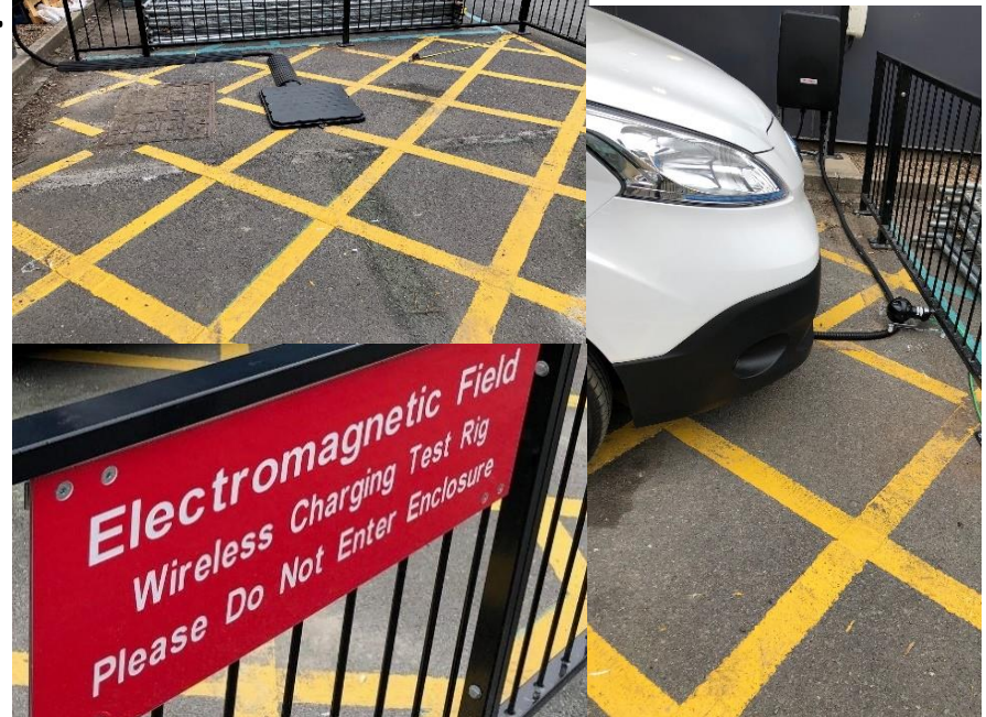
EV retrofitted with VA, VIU and HMI for WPT
