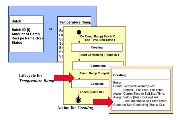
Figure 1: The primary projections of Executable UML
