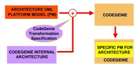
The UML Radar Platform Independent Models (PIMs) are mapped to this specialised CodeGenie Platform Model creating a Platform Specific Model (PSM). The software for the Radar Controller system is generated according to a number of archetype templates that specify the software generated for each PM entity (e.g. a *persistent* attribute).
