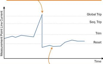
Measurement Point Line Current is below reset. Generators' circuit breakers are re-closed and generators released in priority order.
