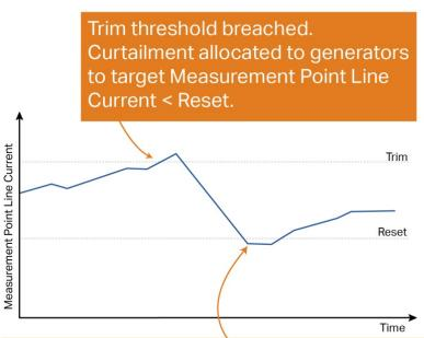
Measurement Point Line Current < Reset. **sgs power flow** enters releasing mode. Releases generation to bring Measurement Point Line Current between Trim and Reset.
