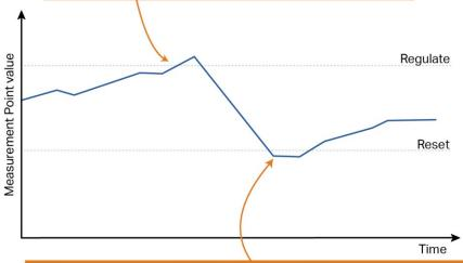
Measurement Point value < Reset. CONNECT+ enters releasing mode. Releases generation to bring Measurement Point value between regulate and reset.
