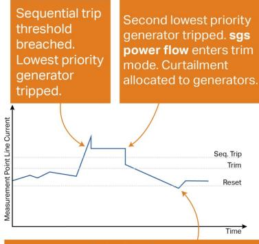
Measurement Point Line Current < Reset. sgs power flow enters releasing mode. Releases generation to bring Measurement Point Line Current between Trim and Reset.
