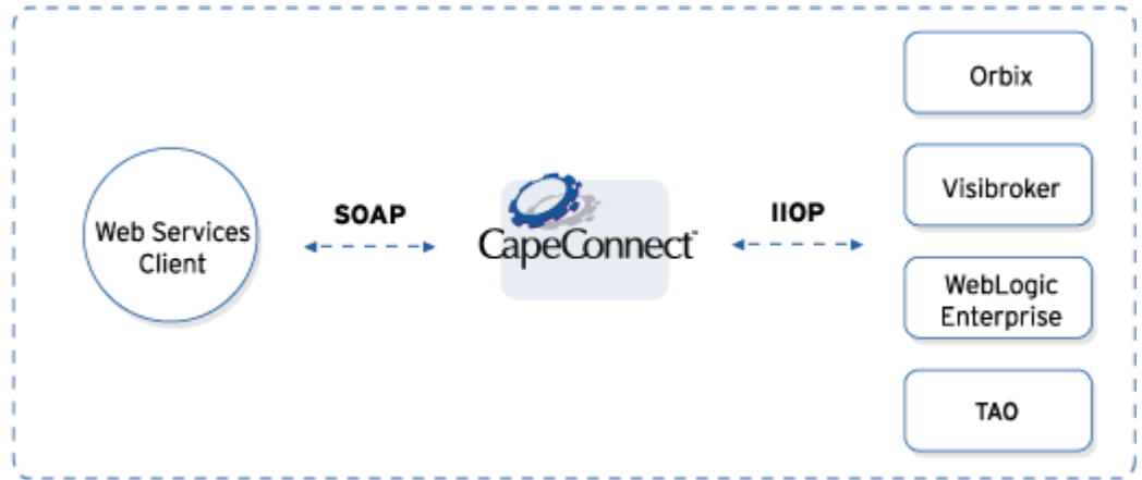
Figure 3: Exposing deployed CORBA ORB components as Web Services
