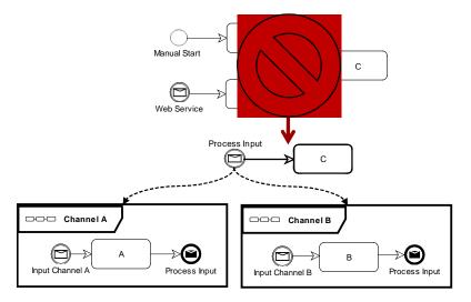
Good practice in process modeling is to separate the level of concerns: the communication channels should be separated from the work being done by the process. Thereby, it is possible to add new communication channels without having to change the process.
