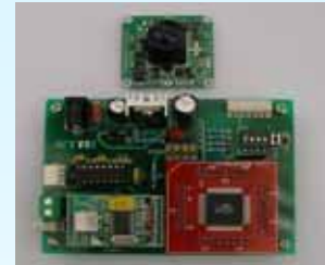
Prototype Detector (Camera + Transceiver)
