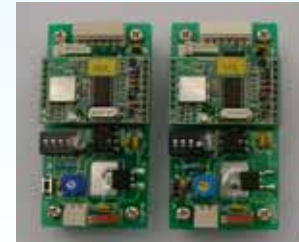
Prototype Tag with Infrared LED
