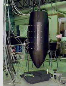
Distributed Active Control: Vibration Damping on Delta-4 Rocket Payload Fairing (1,000 nodes)
