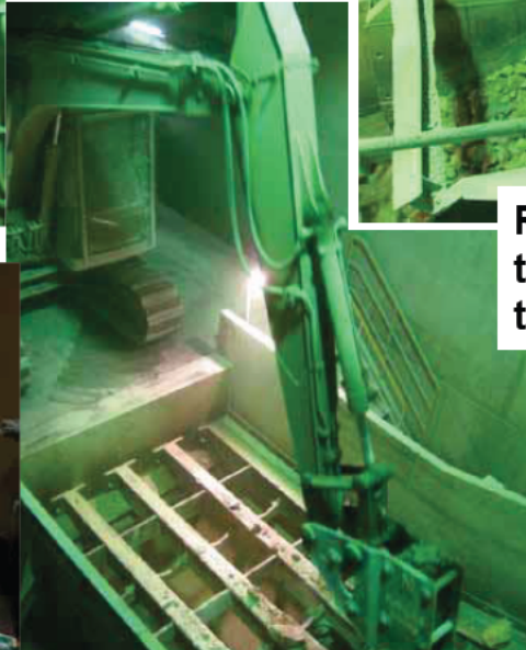
A hydraulic breaker and grizzly bars
