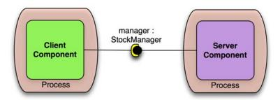
At deployment time this will lead to the following deployed components, connector fragment, and connections. The client component and fragment are required to be deployed within the same process.
