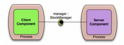
At deployment time this will lead to the following deployed components, connector fragment, and connections. The client component and fragment are required to be deployed within the same process.
