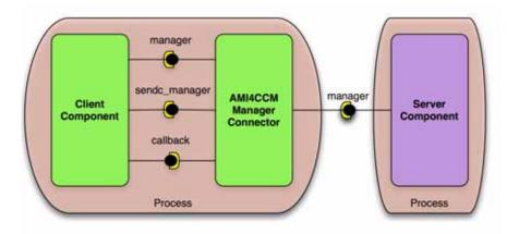
In case a multiplex receptacle has been enabled for AMI4CCM, for each server component a connector fragment will be deployed collocated to the client. Between the connector fragment and the server component only a simplex connection can be defined.
