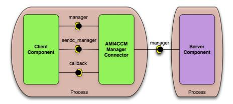
In case a multiplex receptacle has been enabled for AMI4CCM, for each server component a connector fragment will be deployed collocated to the client. Between the connector fragment and the server component only a simplex connection can be defined.
