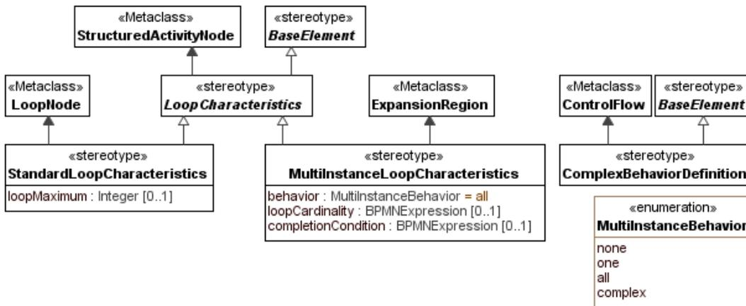
Figure 25: Loop Characteristics
