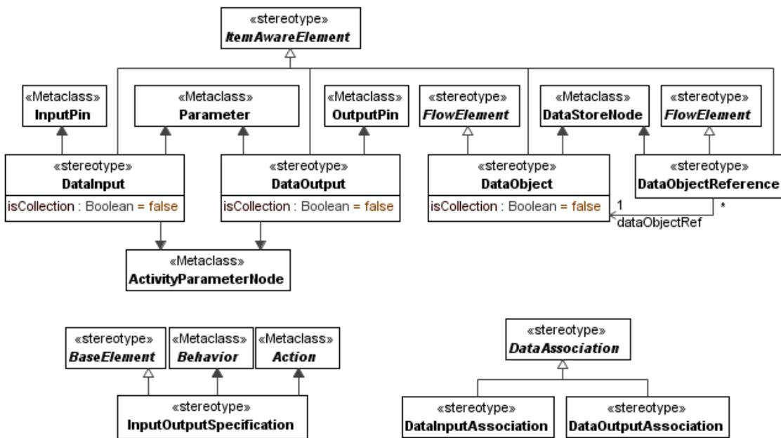
Figure 21: Input Output Specifications and Data Objects
