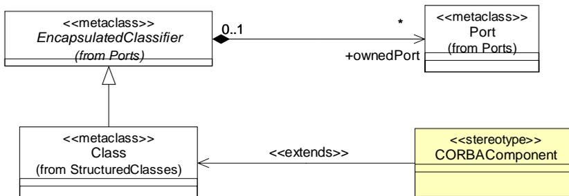
**Figure 8.21 - ComponentIDL Profile: Extended UML classes (I)**
