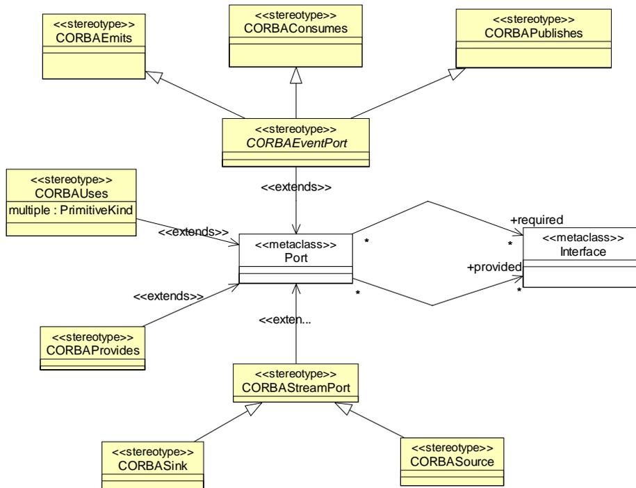
**Figure 8.22 ComponentIDL Profile: Extended UML classes (II)**
