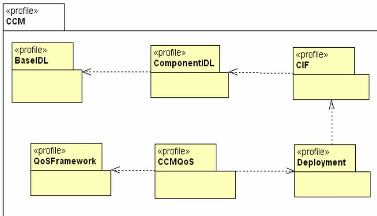
Figure 8.1 - CCM Profile package structure
