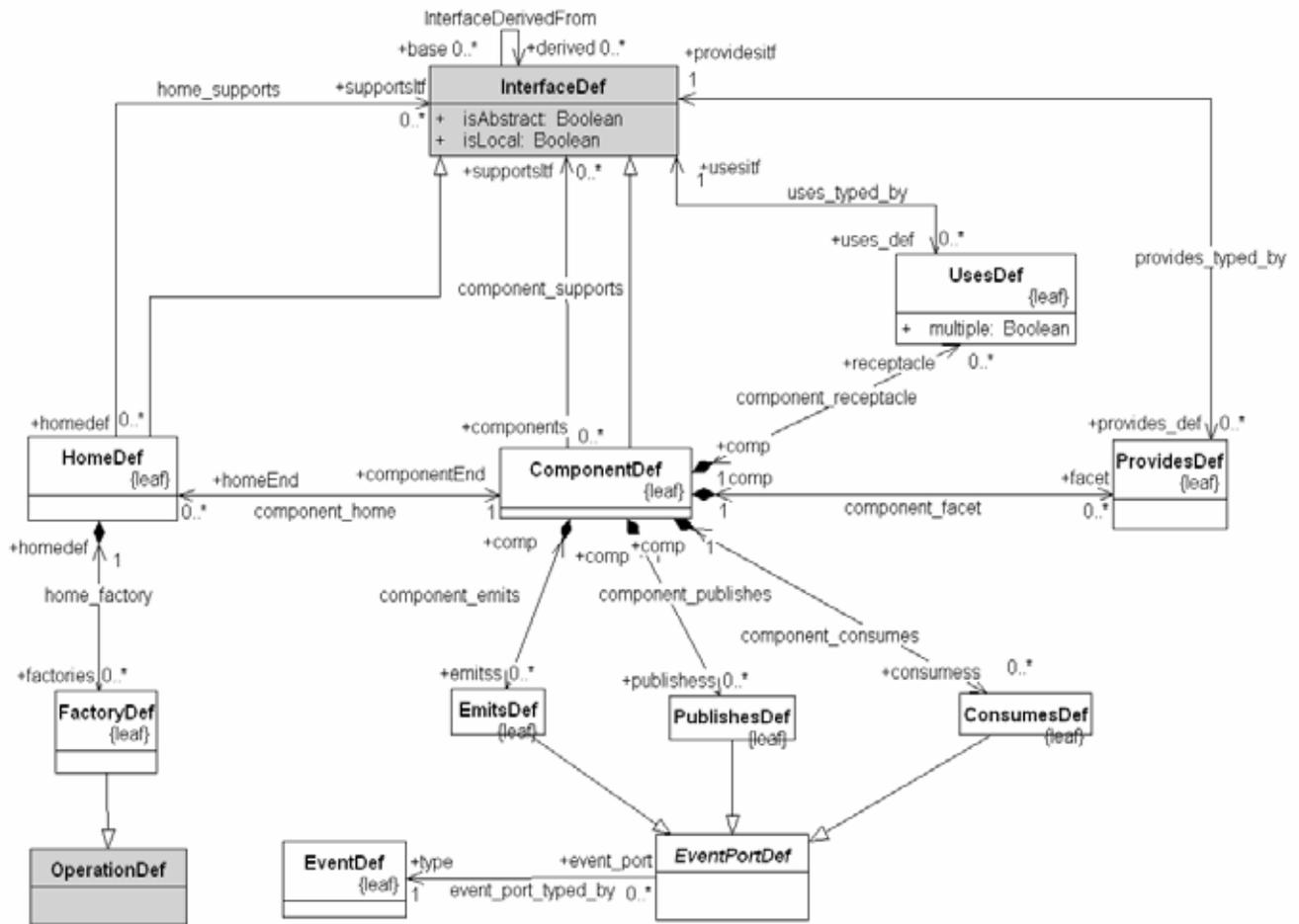
Figure 8.32 - ComponentIDL metamodel for the Lightweight CCM
