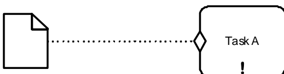
Figure 6.37 - Using the Sentry-based connector to visualize dependency between a Task and a CaseFileItem
