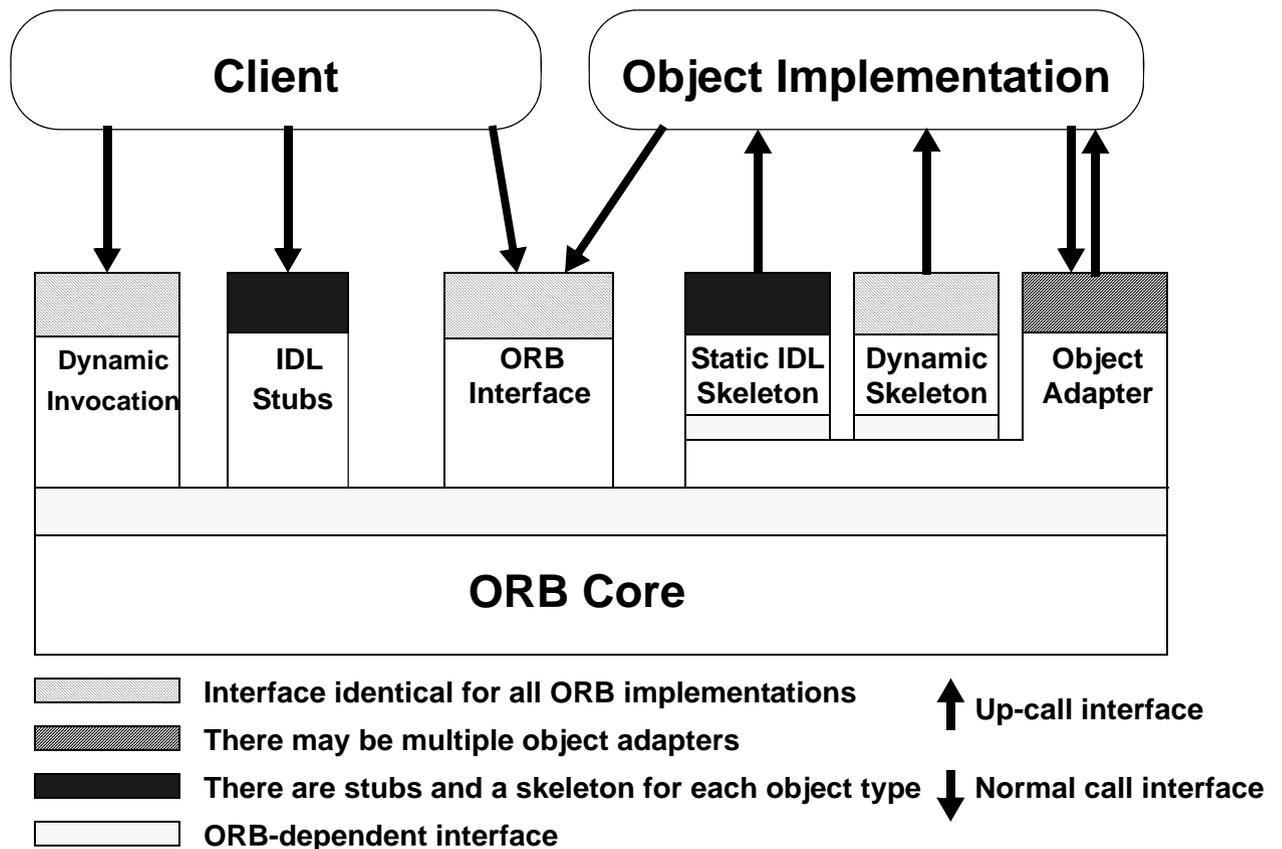
**Figure 4.2- The Structure of Object Request Interfaces**
