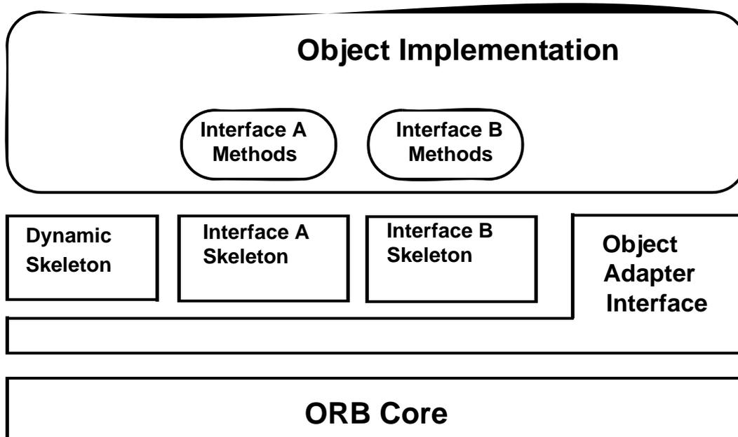
Figure 4.8- The Structure of a Typical Object Adapter
