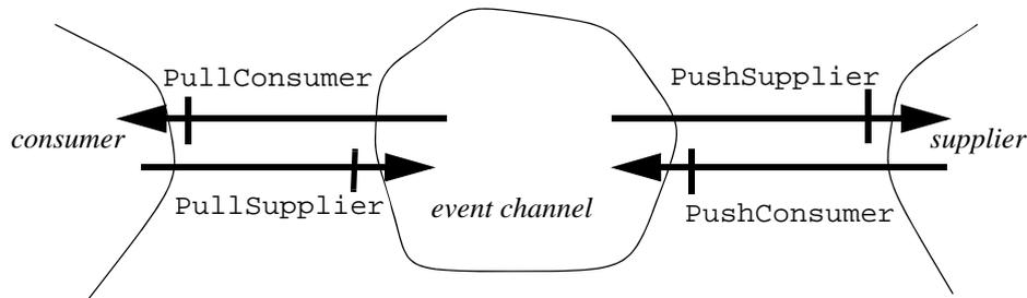
**Figure 14.5- Push-style Communication Between a Supplier and an Event Channel, and Pull-style Communication Between a Consumer and an Event Channel**
