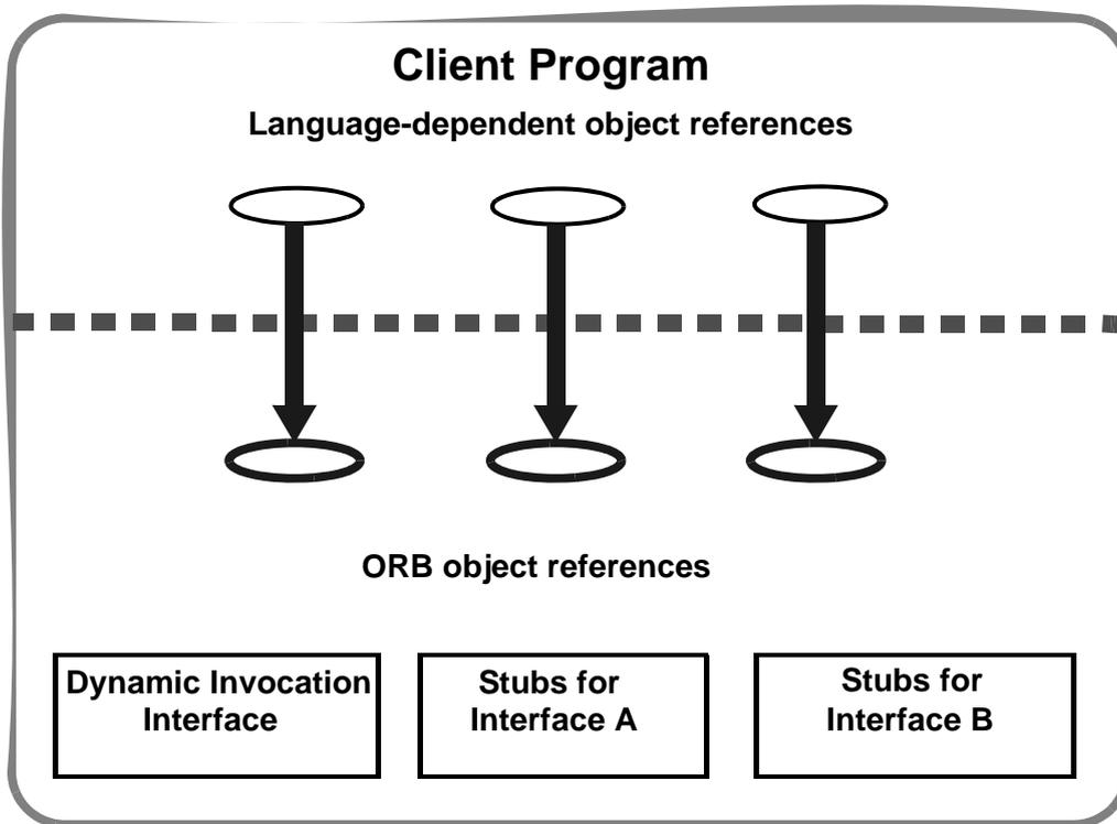
**Figure 4.6- The Structure of a Typical Client**
