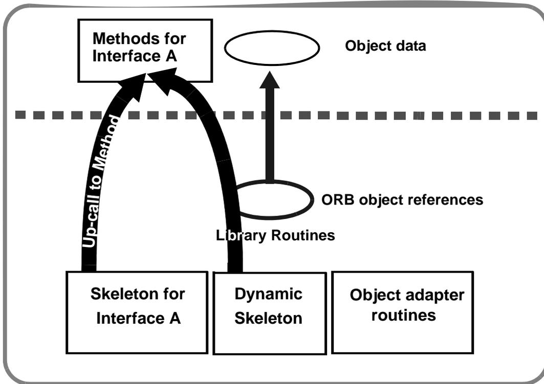
**Figure 4.7- The Structure of a Typical Object Implementation**
