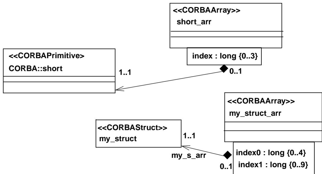
Figure 3-29 Typedefed Array Example
