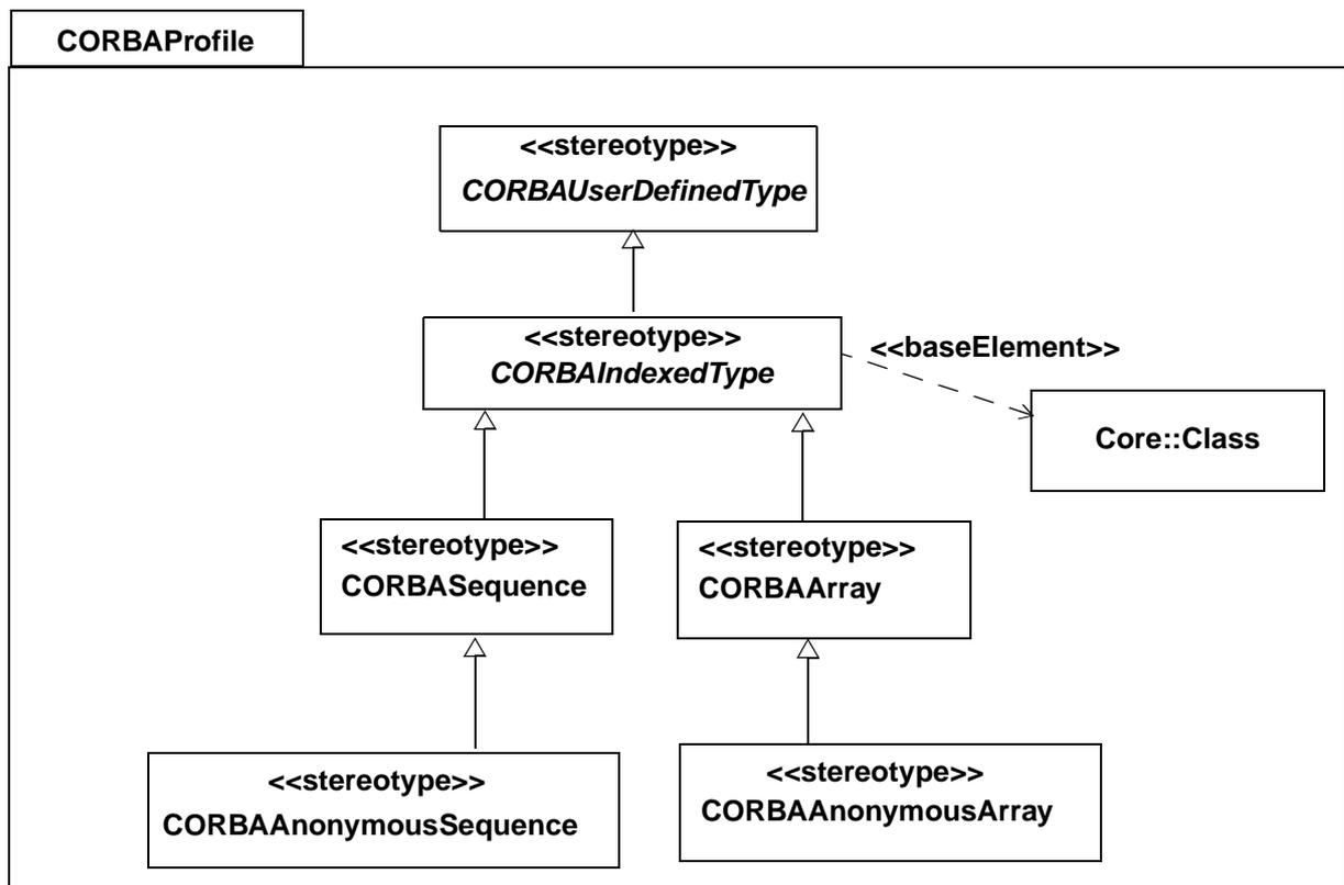
Figure 3-6 Virtual Metamodel for CORBA Indexed Types
