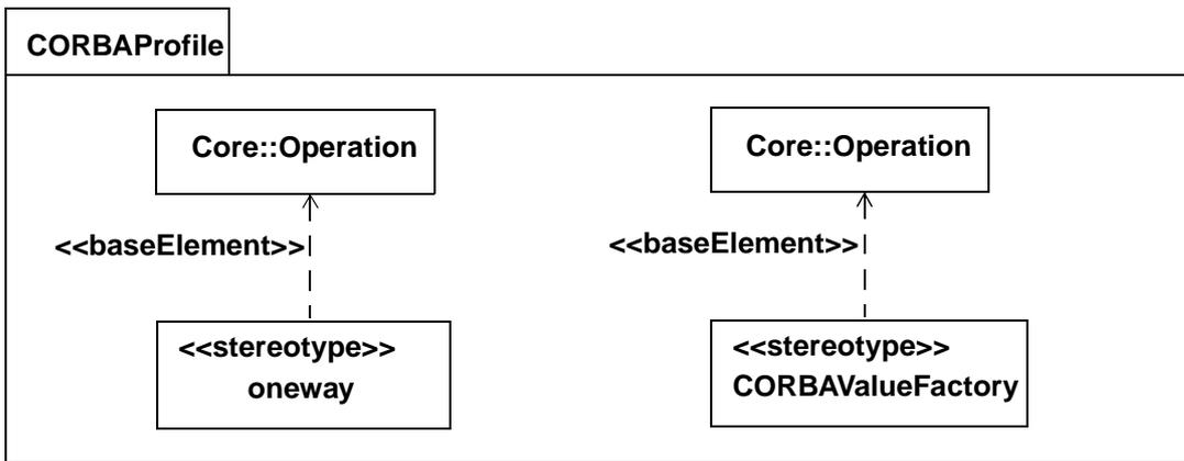
Figure 3-10 Virtual Metamodel for Stereotypes of Operation
