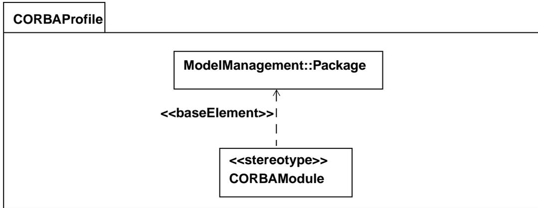
Figure 3-5 Virtual Metamodel for CORBA Module
