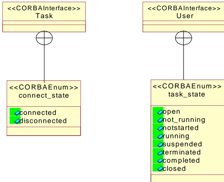
This diagram shows the the definitions of the enums and shows their namespace containment within specific interfaces.
