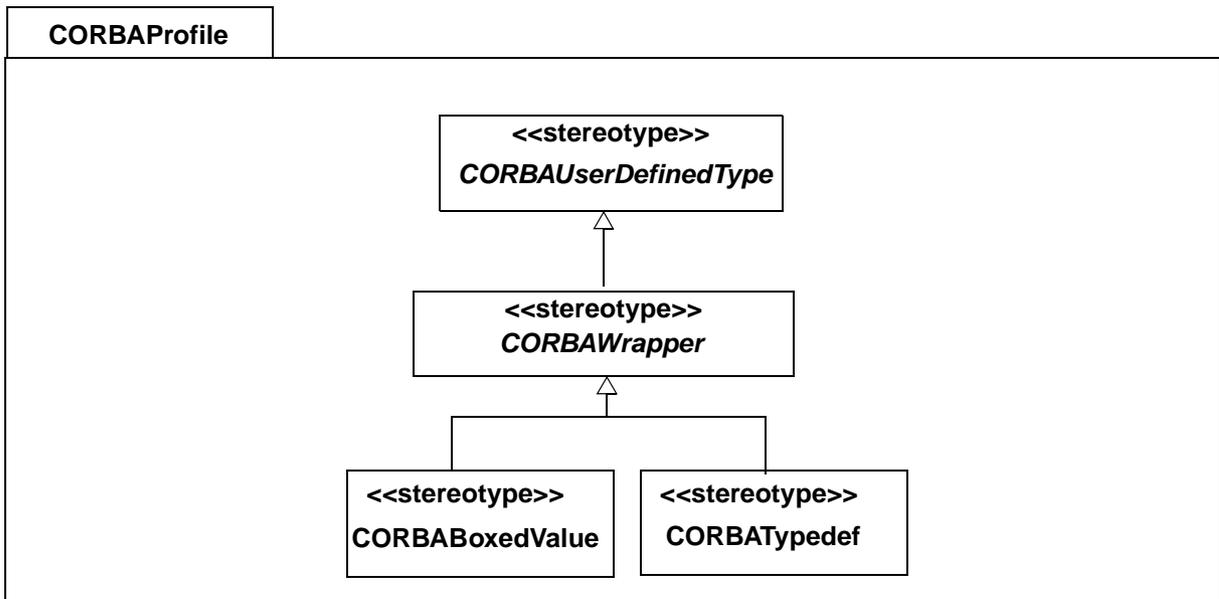
Figure 3-7 Virtual Metamodel for CORBA Wrapper Types
