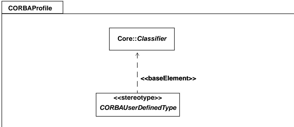
Figure 3-2 Virtual Metamodel for CORBA User-Defined Types
