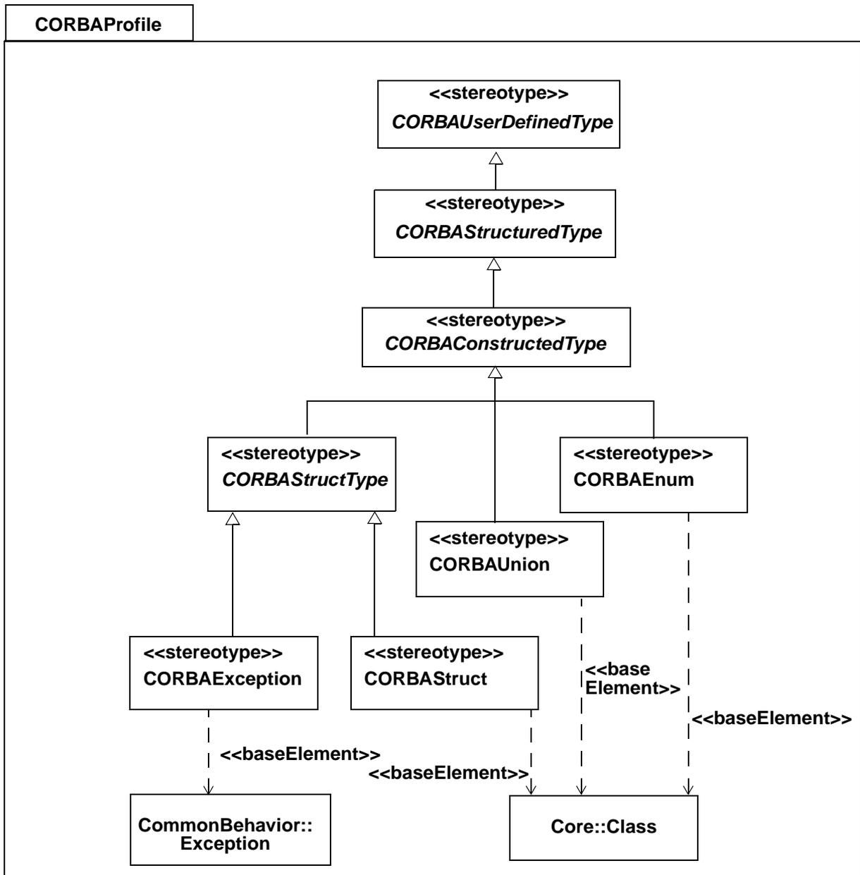
Figure 3-4 Virtual Metamodel for CORBAConstructed Types
