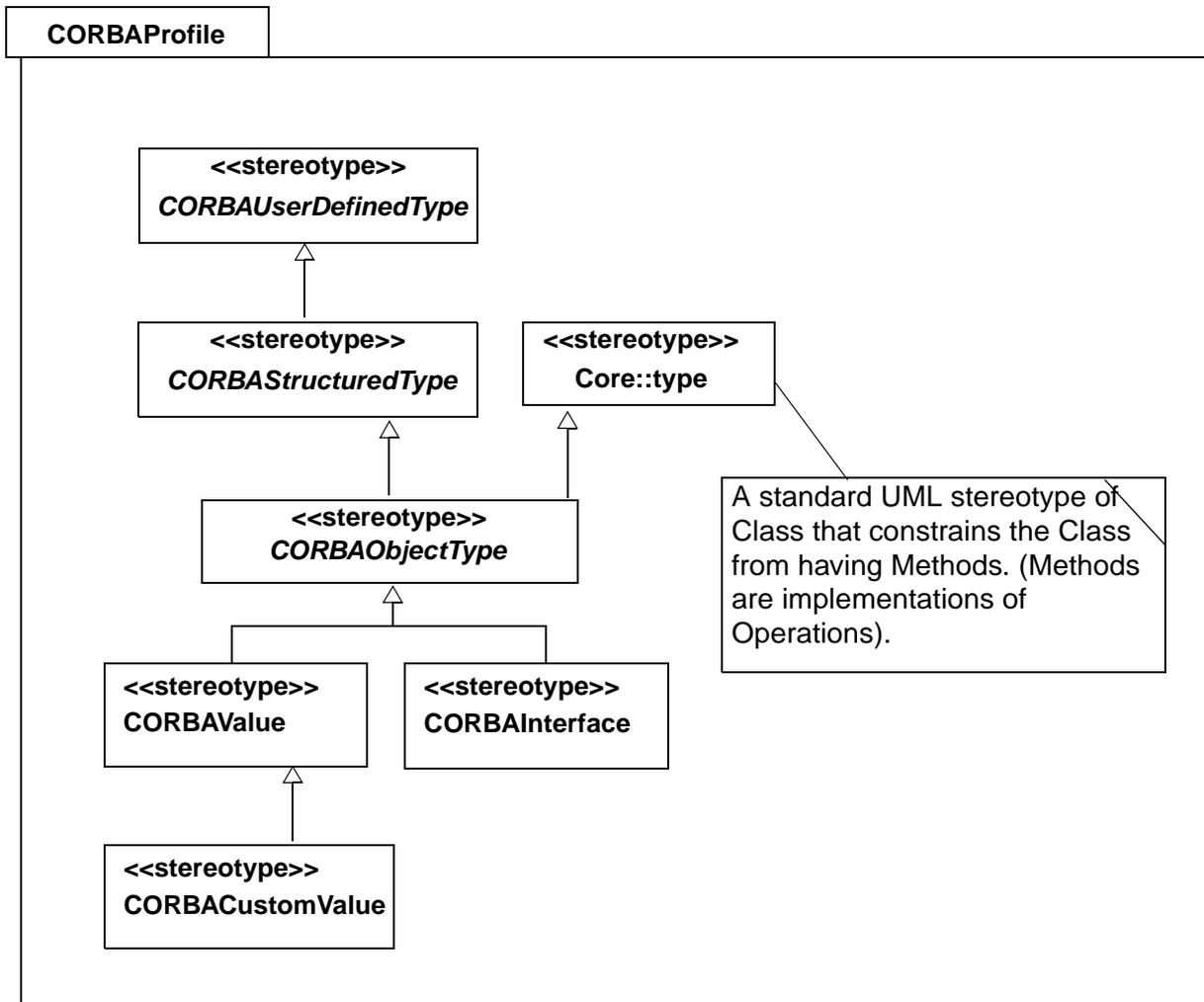
Figure 3-3 Virtual Metamodel for CORBA Object Types
