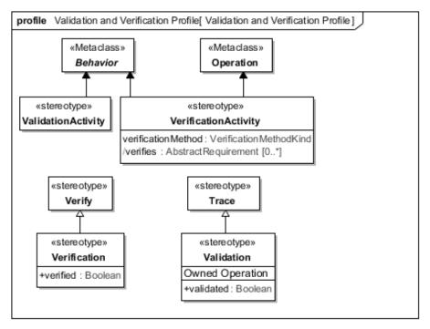
Figure 5 Validation and Verification Profile
