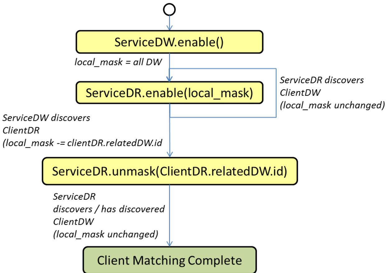
Figure 7.3 - The service-side client matching algorithm
