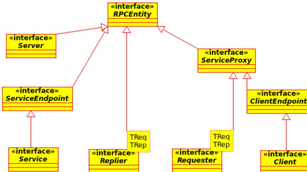
Figure 7.5 - Inheritance Hierarchy of RPC Entities (TReq, TRep are type parameters)
