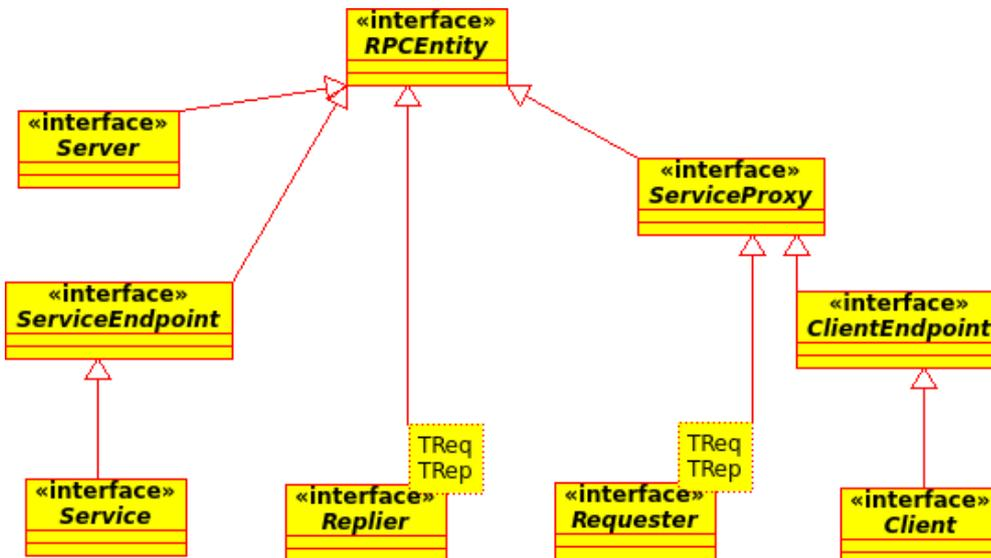
Figure 7.5 - Inheritance Hierarchy of RPC Entities (TReq, TRep are type parameters)
