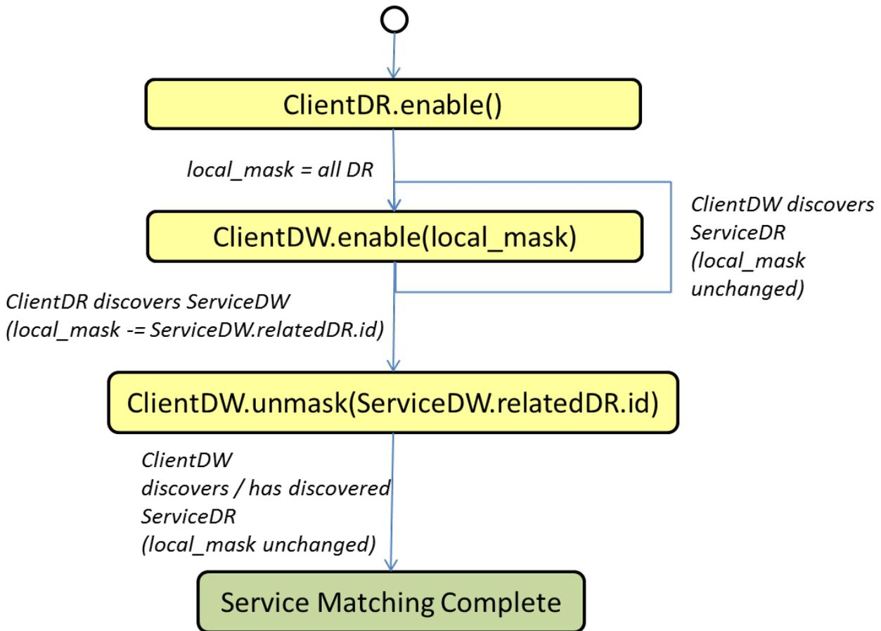
Figure 7.4 - The client-side service matching algorithm
