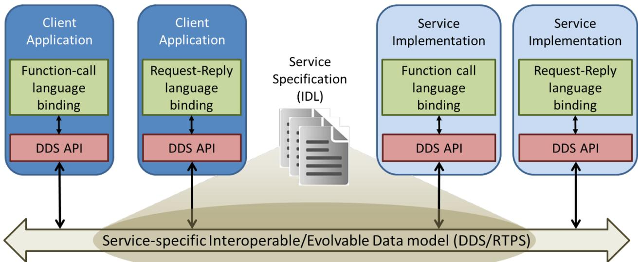
**Figure 7.2 - Strong decoupling of language binding (function-call and request /reply) from the service-specific data model**
