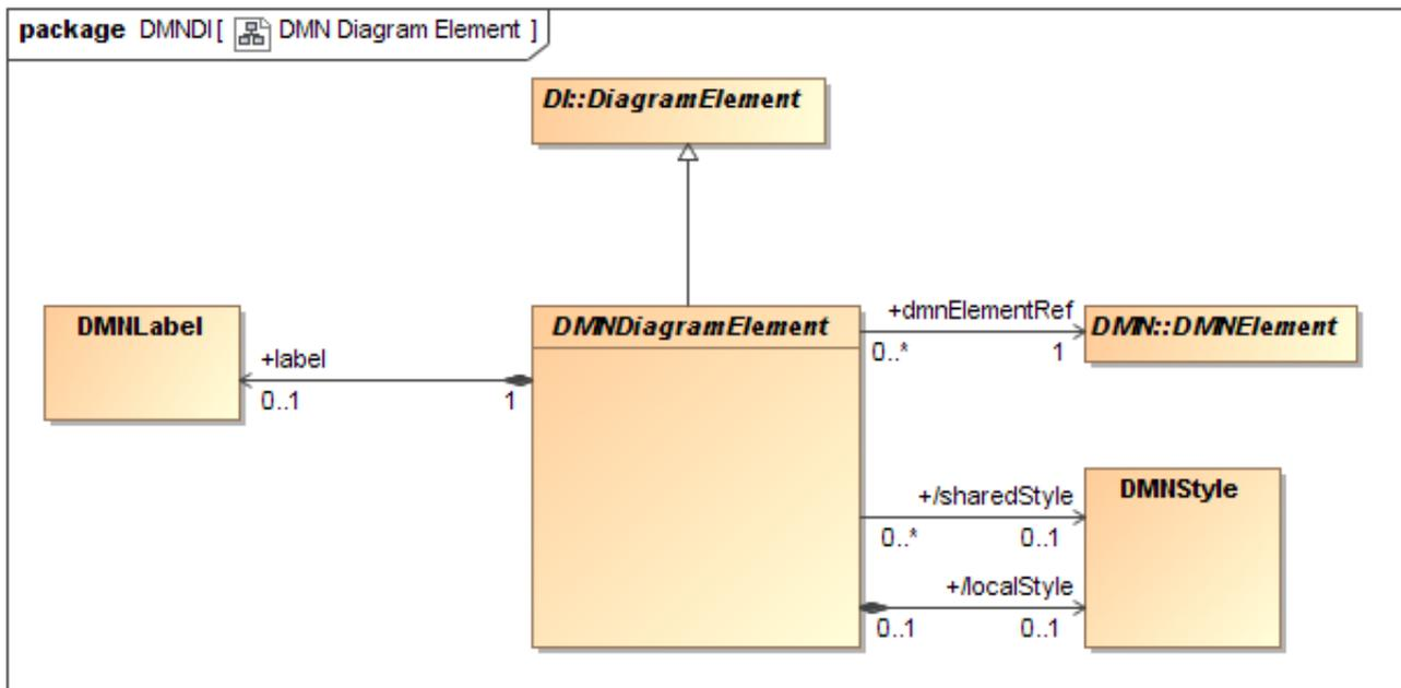
**Figure 13.3: DMNDiagramElement**
