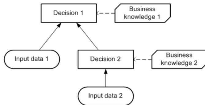
**Figure 5.5: A simple Decision Requirements Diagram (DRD)**
