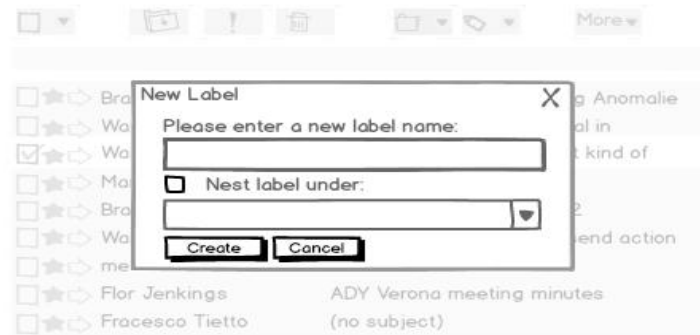
Figure A.16 - The Create New event causes a modal view container to be displayed, whereby the user can create a new tag and associate the selected messages with it.
