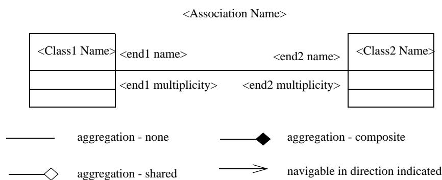
**Figure 8.6 - An M2-level Association in UML notation**
