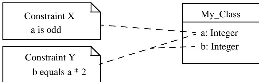
**Figure 6.5 - Examples of Constraints**
