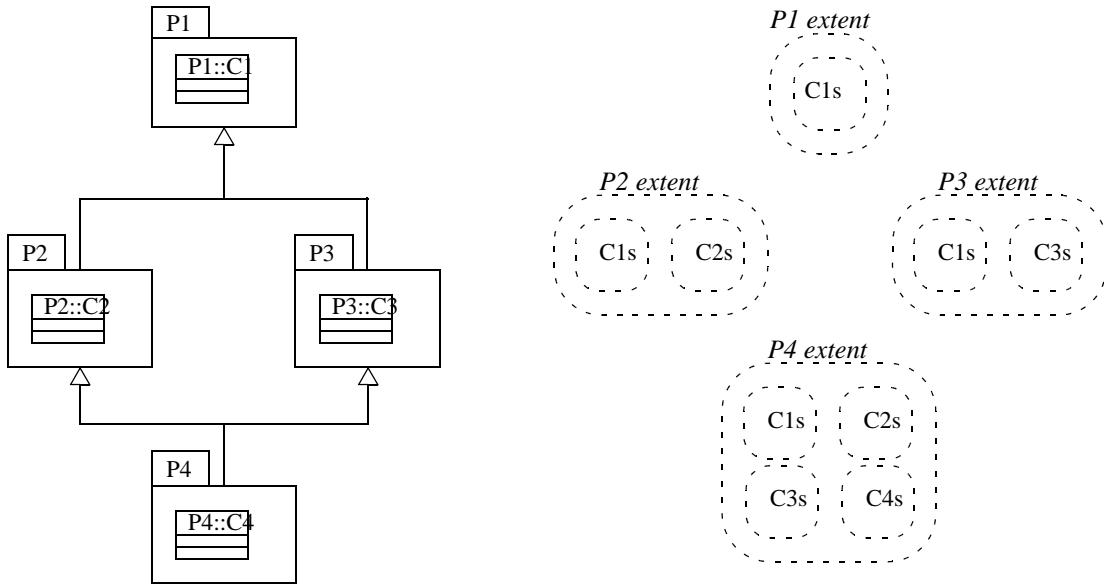
**Figure 8.4 - Extents for Multiply Inheriting Packages**
