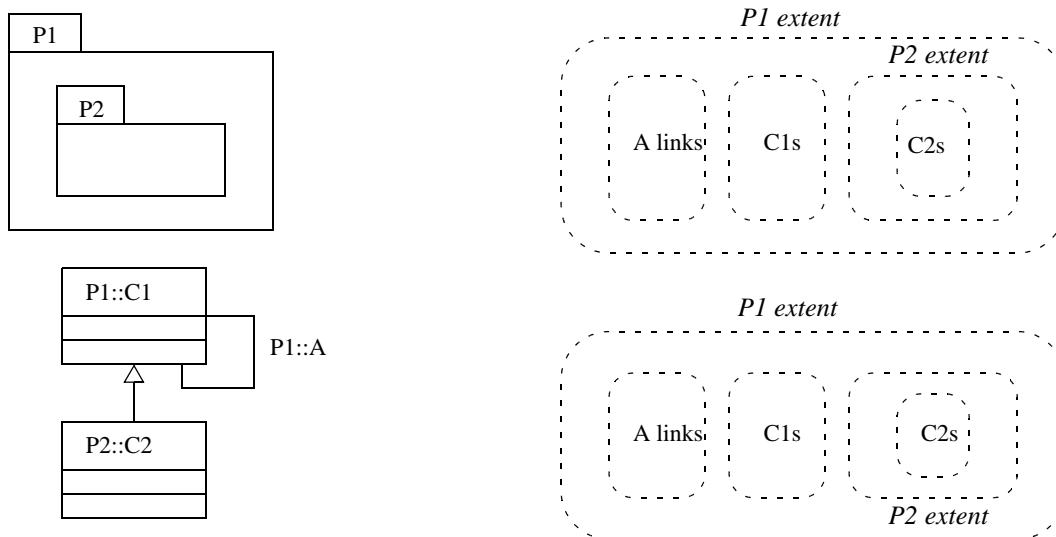
**Figure 8.3 - Extents for two meta-model instances**
