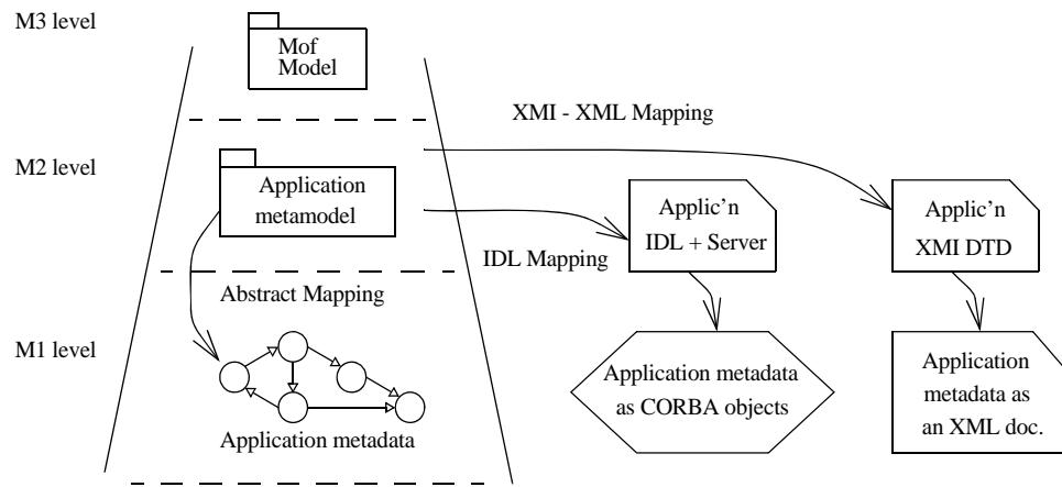
**Figure 6.6 - The function of MOF Technology Mappings**
