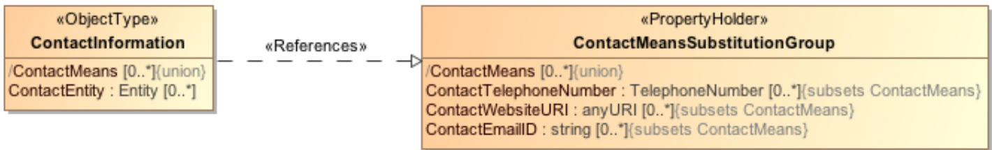
Figure 7-32 Representation of a substitution group using UML subsetted properties in a PIM
