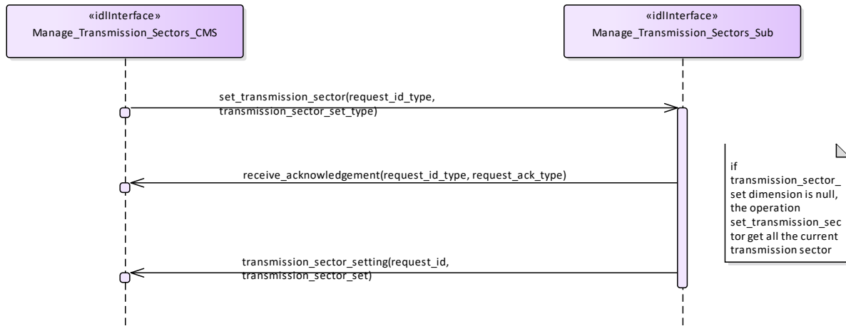
Figure 7- 151: Basic Flow - Manage Transmission Sectors - Enable/Disable (Interaction diagram)
