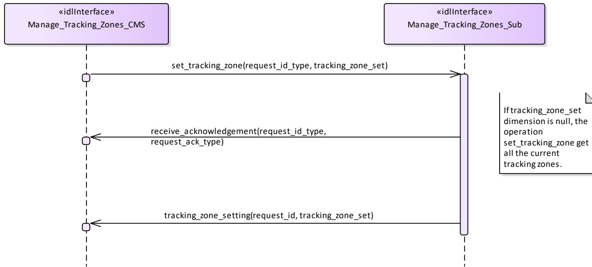
Figure 7- 178: Basic Flow - Manage Tracking Zone - Enable/Disable (Interaction diagram)
