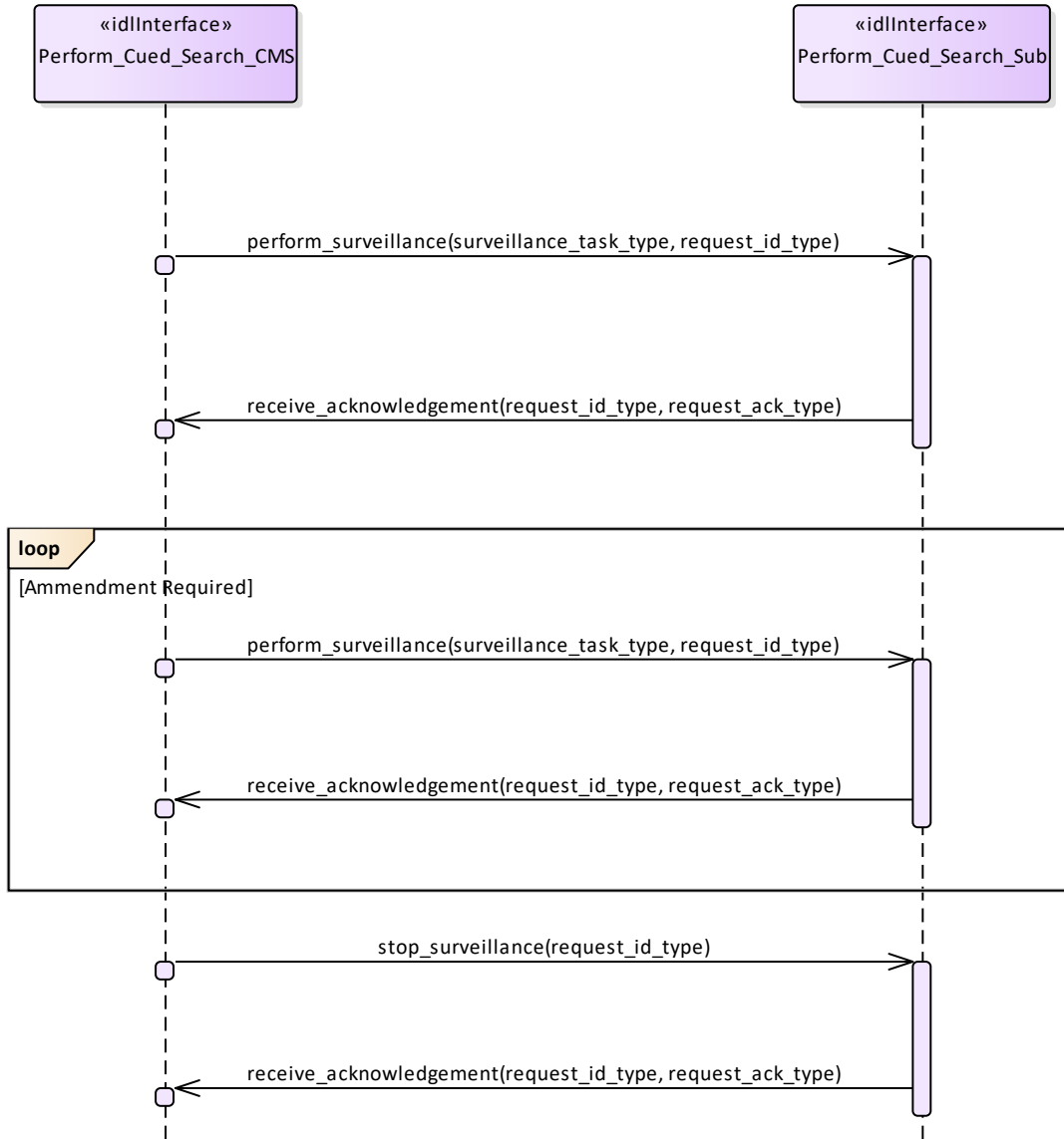
Figure 7- 122: Basic Flow - Perform Surveillance (Interaction diagram)
