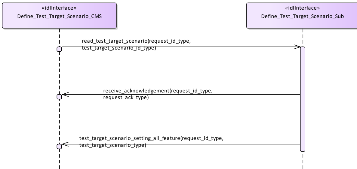
Figure 7- 157: Basic Flow - Inspect a Test Target Scenario (Interaction diagram)
