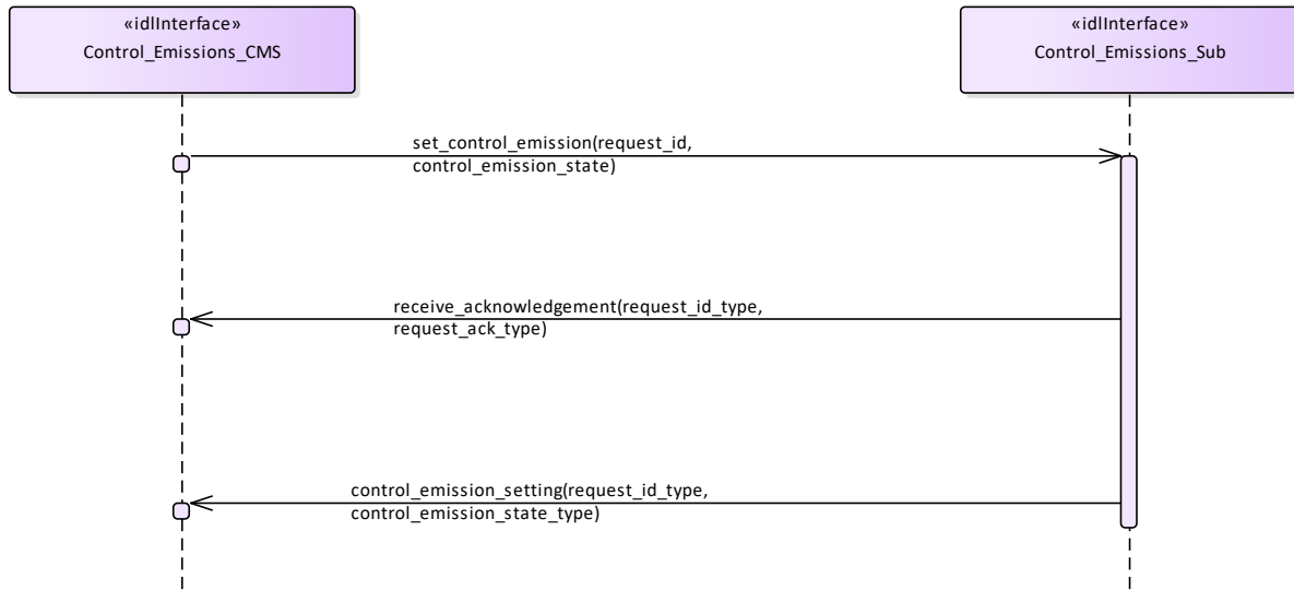
Figure 7- 153: Basic Flow - Control Emissions - On/Off (Interaction diagram)
