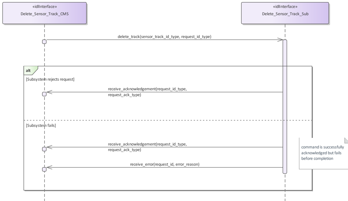
Figure 7.213 Alternative Flow - Delete Sensor Track (Interaction diagram)
