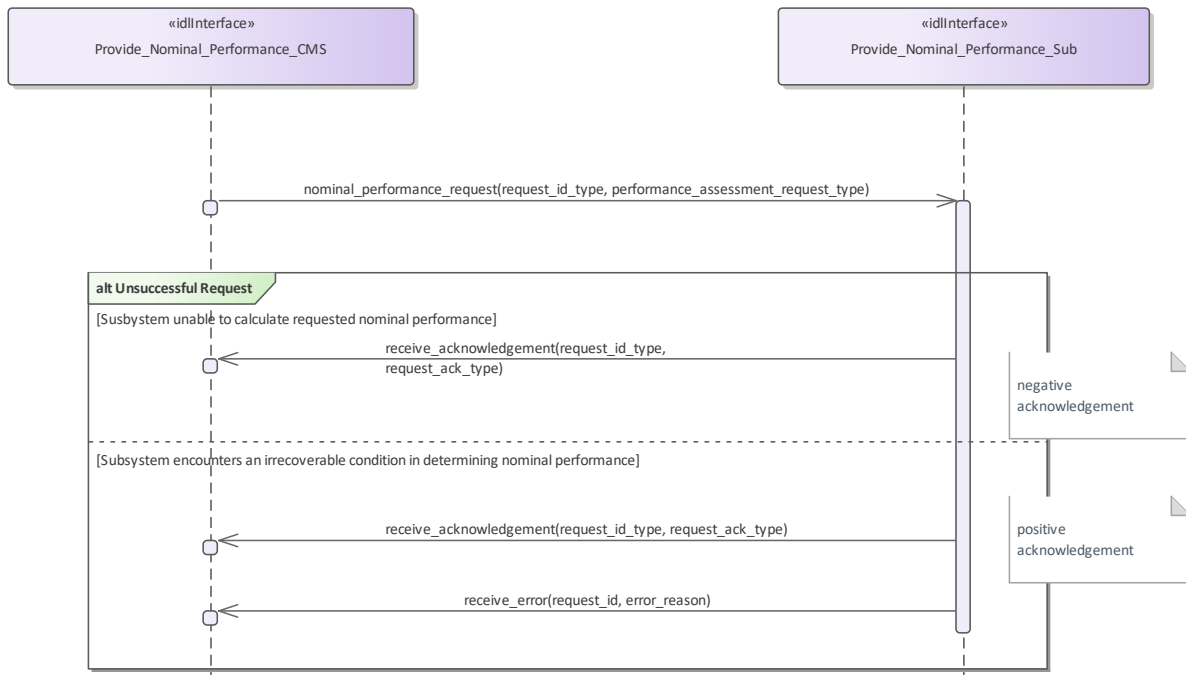
Figure 7.197 Alternative Flow - Provide Nominal Performance (Interaction diagram)
