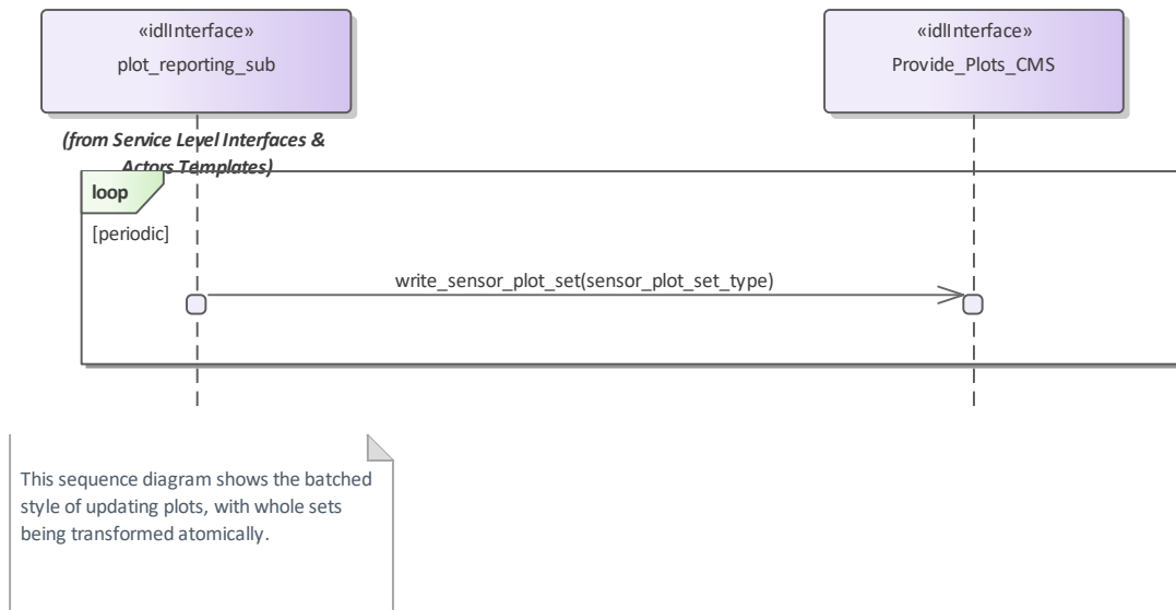
Figure 7.178 Basic Flow - Provide Plots (Sets) (Interaction diagram)
