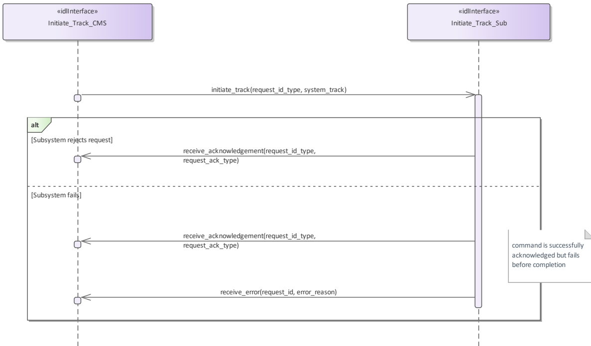
Figure 7.217 Alternative Flow - Initiate Track - loss of mastership (Interaction diagram)
