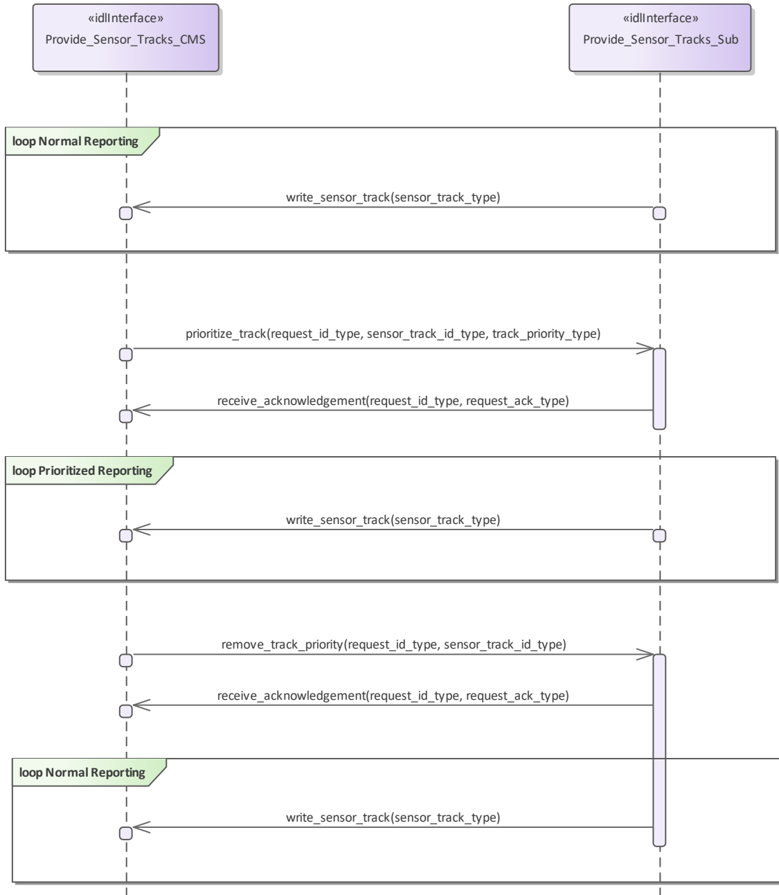
Figure 7.209 Basic Flow - Change Priority (Interaction diagram)
