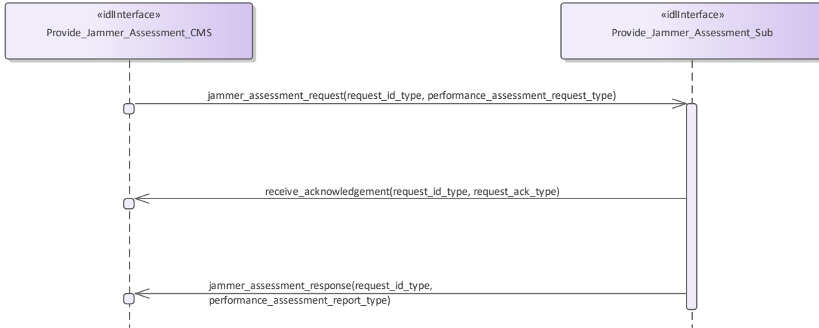
Figure 7.202 Basic Flow - Provide Jammer Assessment (Interaction diagram)
