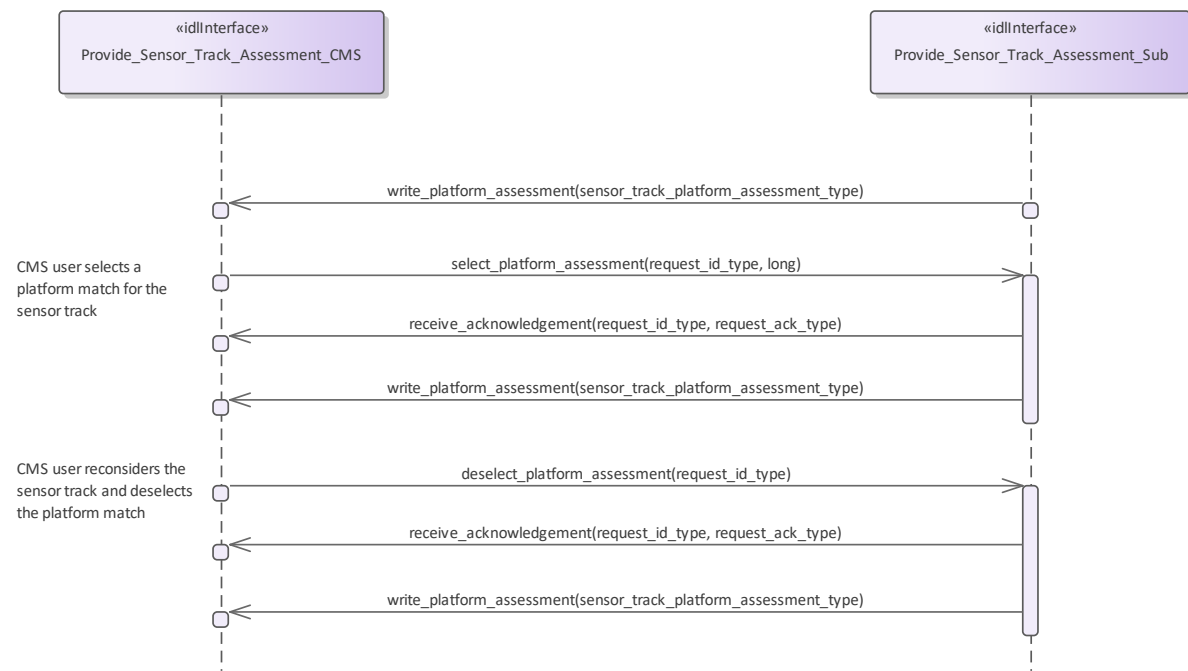
Figure 7.166 Assess_Sensor_Track - platform deselection (Interaction diagram)
