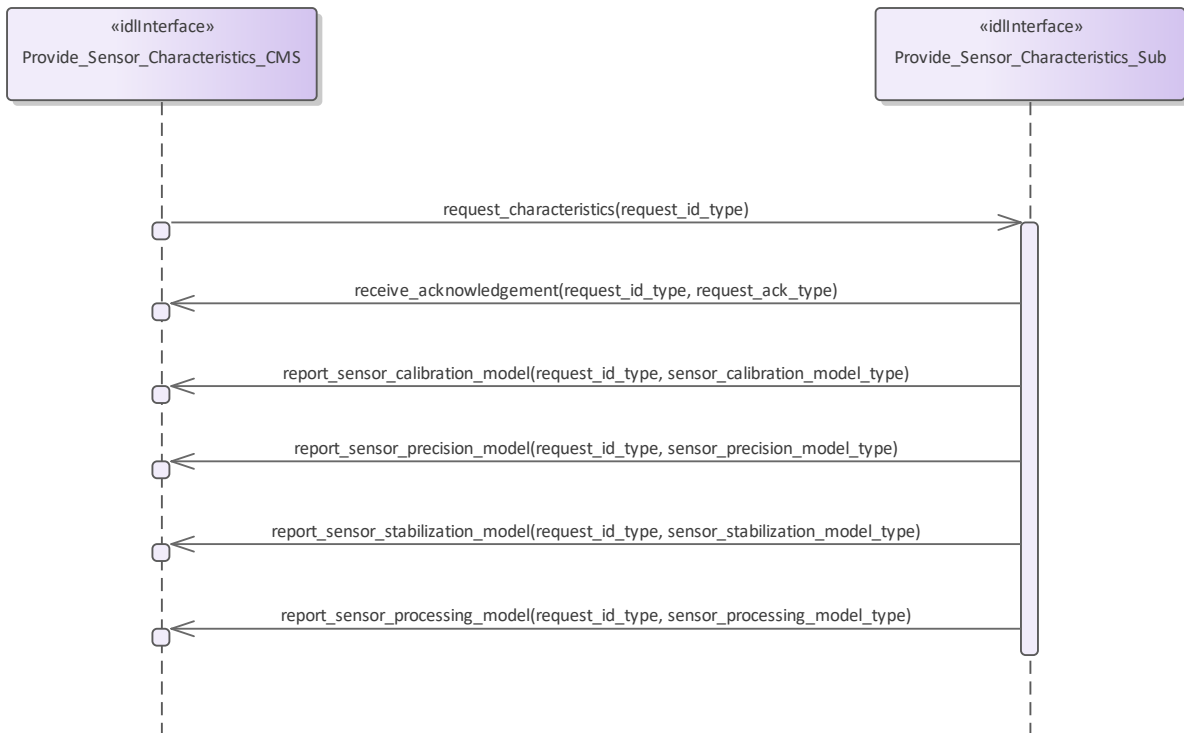
Figure 7.175 Basic Flow - Provide_Sensor_Characteristics on request (Interaction diagram)
