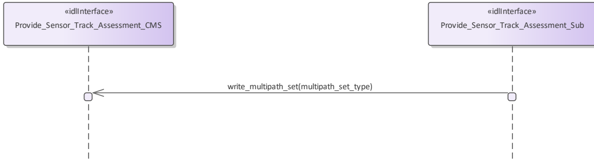
Figure 7.165 Assess_Sensor_Track - multipath (Interaction diagram)
