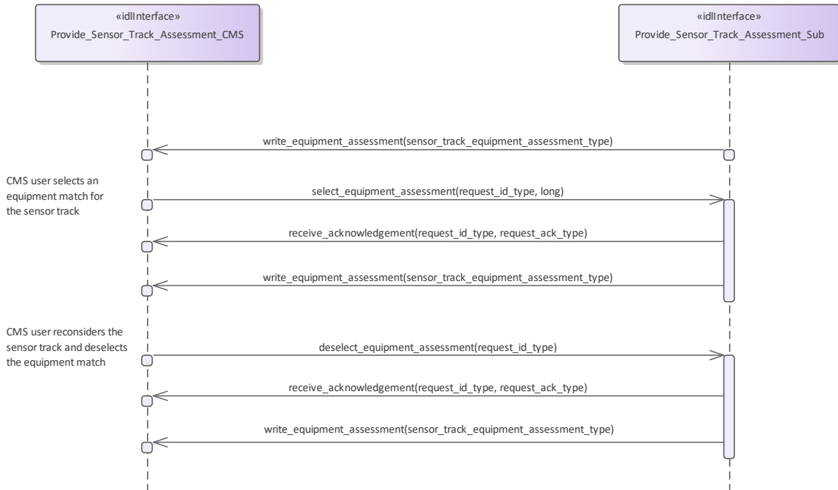
Figure 7.163 Assess_Sensor_Track - equipment deselection (Interaction diagram)
