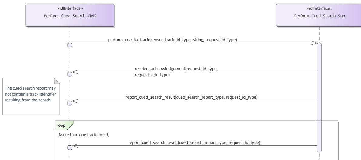
Figure 7.155 Alternative Flow - Sensor does not Perform Cued To Track (Interaction diagram)
