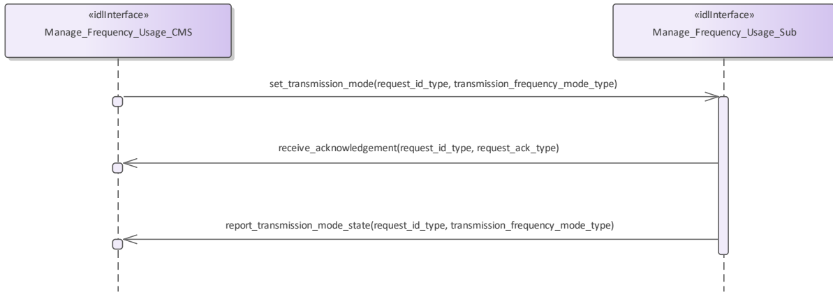
Figure 7.184 Basic Flow - Transmission Mode Selection (Interaction diagram)
