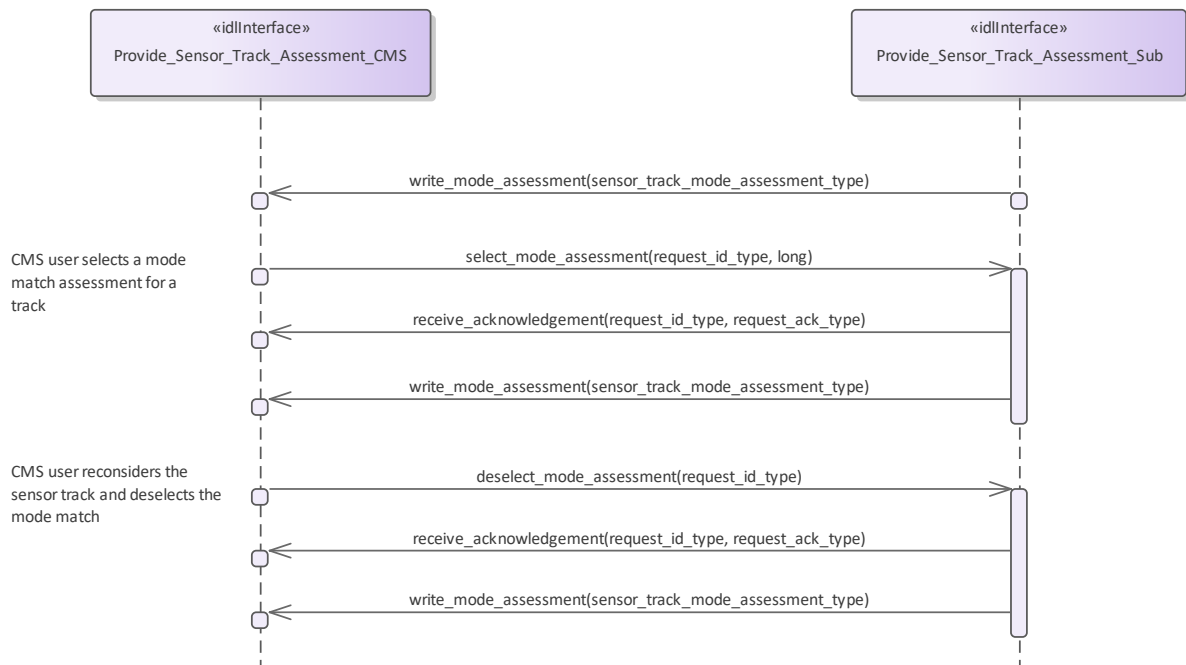
Figure 7.164 Assess_Sensor_Track - mode deselection (Interaction diagram)
