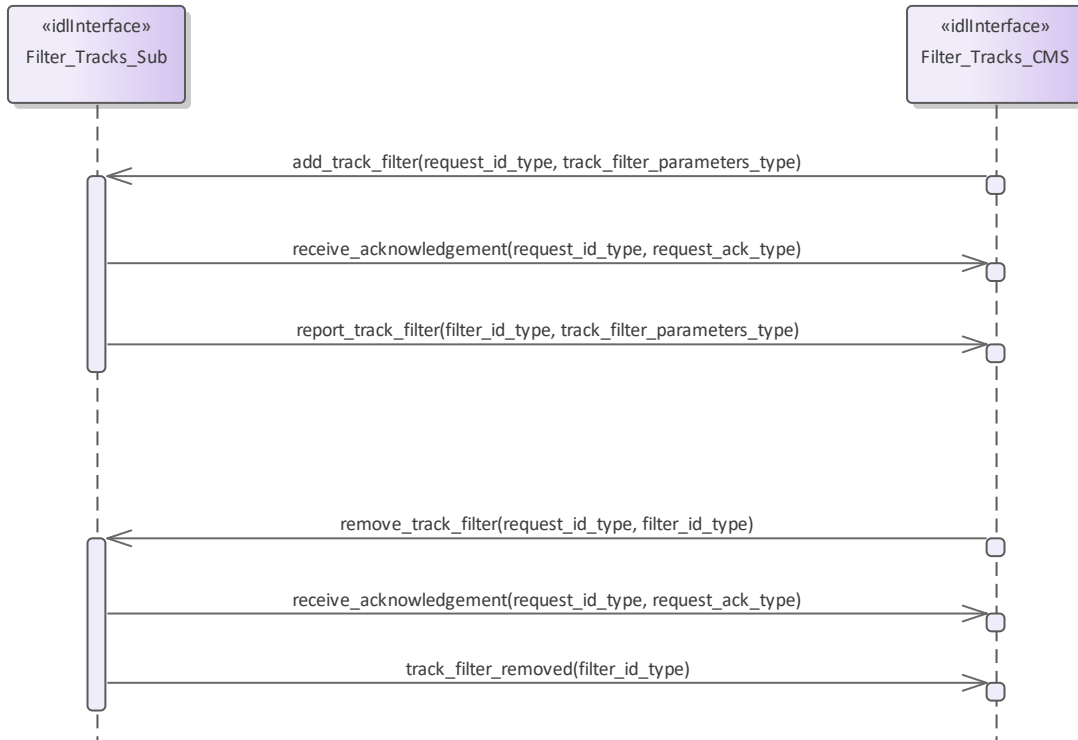
Figure 7.204 Basic Flow Filter_Tracks (Interaction diagram)
