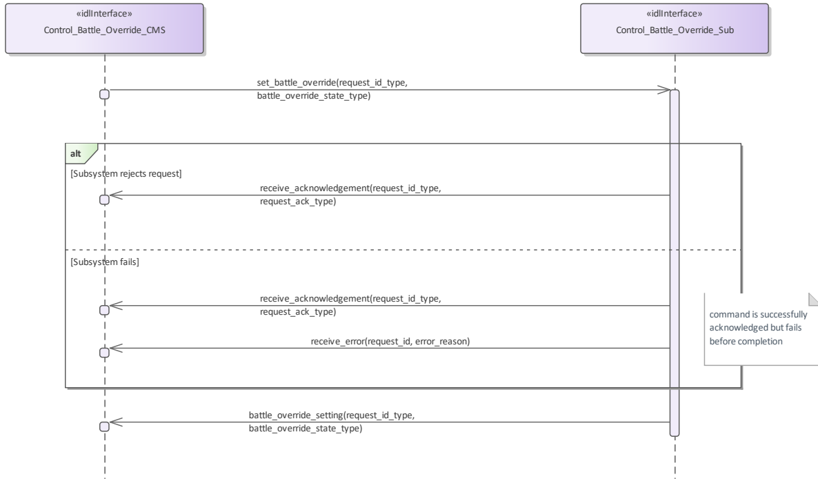
Figure 7.120 Alternative Flow - Control Battle Override - Set/Reset - loss of mastership (Interaction diagram)
