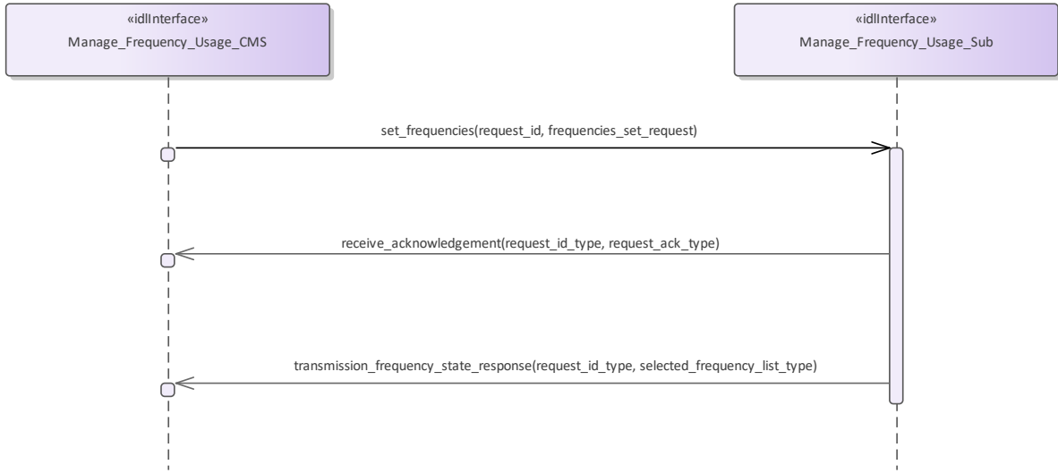
Figure 7.182 Basic Flow - Enable/Disable Frequency Usage (Interaction diagram)
