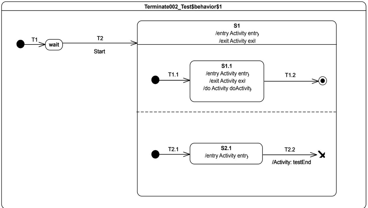
**Figure 9.79 - Terminate 002 Test Classifier Behavior**
