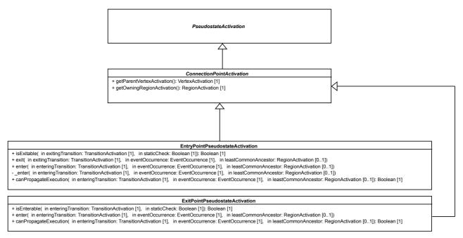
Figure 8.11 - EntryPointActivation and ExitPointActivation
