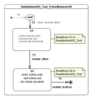
Figure 9.112 - Redefinition 005 Test Classifier Behavior - Runtime State Machine
