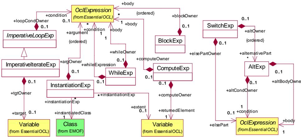
Figure 8.5 - Imperative OCL Package - Control and instantiation constructs
