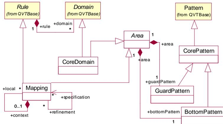
**Figure 9.2 - QVTCore Package - Mappings and Patterns**
