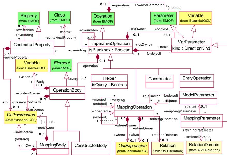
Figure 8.2 - QVT Operational Package - Defining Imperative Features
