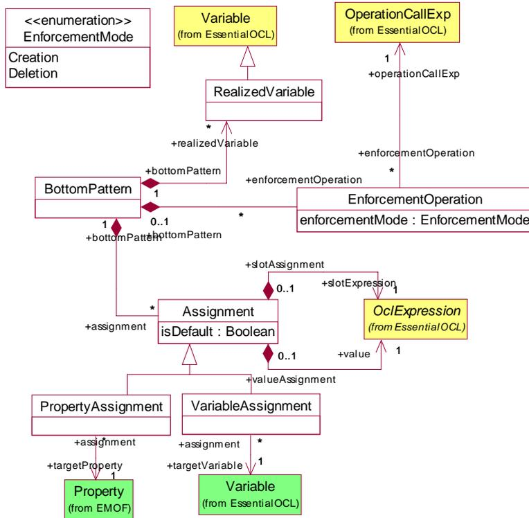
Figure 9.3 - QVT Core Package - Bottom patterns
