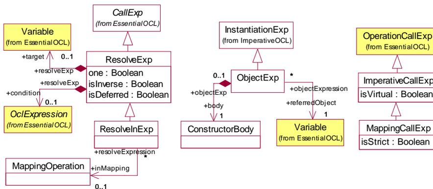
**Figure 8.3 - QVT Operational Package / Usage of Imperative Operations**
