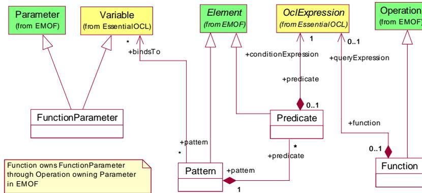
Figure 7.5 - QVTBase Package - Patterns and Functions
