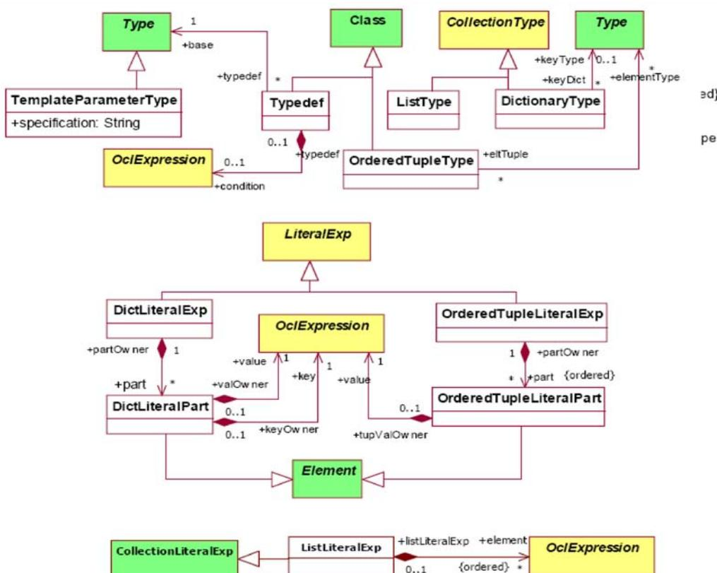
Figure 8.7 - Imperative OCL Package - Type extensions
