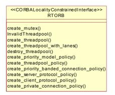
Figure B-7 The Real-Time ORB interface specification
