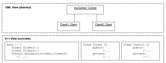
Figure 4-12 Example of refinement-type layering
