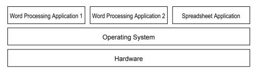
Figure 4-13 An example of realization layering
