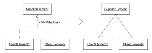
Figure 4-17 Substitution semantics of synchronous and asynchronous forms of deployment
