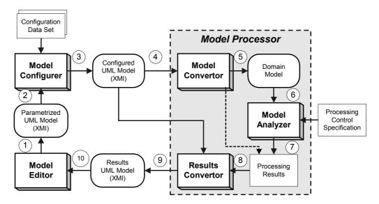
Figure 10-1 General model-processing framework
