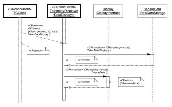
Figure 6-3 Concurrency Model - asynchronous case
