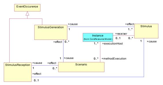
Figure 4-4 The basic causal loop model
