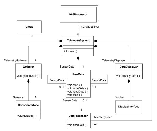
Figure 7-4 Example telemetry system specification
