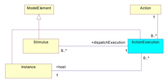
Figure 4-20 Proposed changes to the UML metamodel (ActionExecution)
