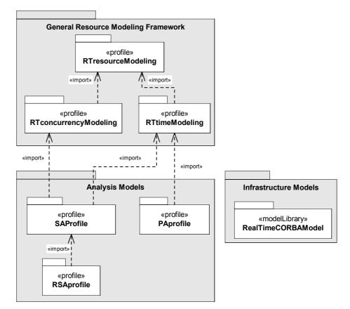
*Figure 3-3* The structure of the profile
