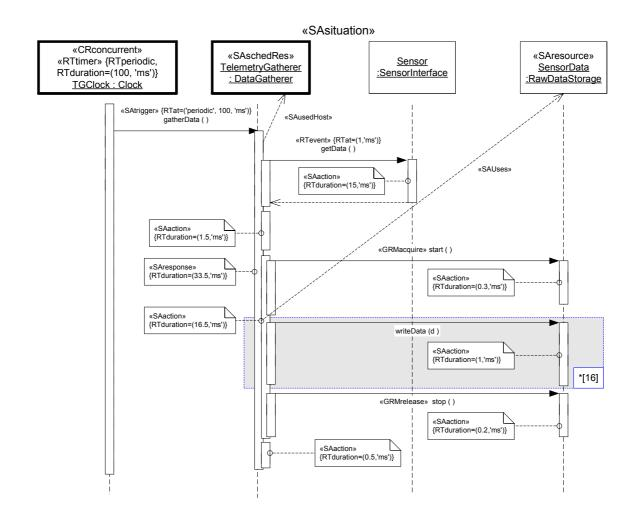
Figure 7-5 Showing a trigger and its response in a Sequence Diagram
