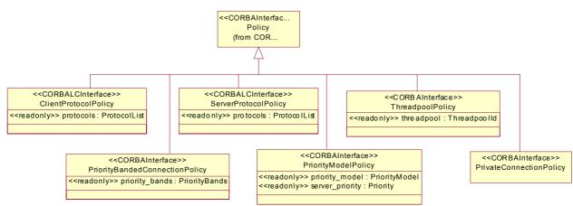
The remaining interfaces are for setting policies of various kinds that apply in RT CORBA (Figure B-8 and Figure B-9).
