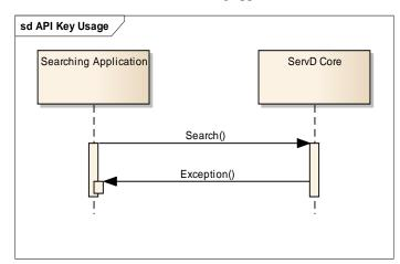
A Searching application makes a call to a ServD method (Search) using an API key that is not registered with the ServD Core.
