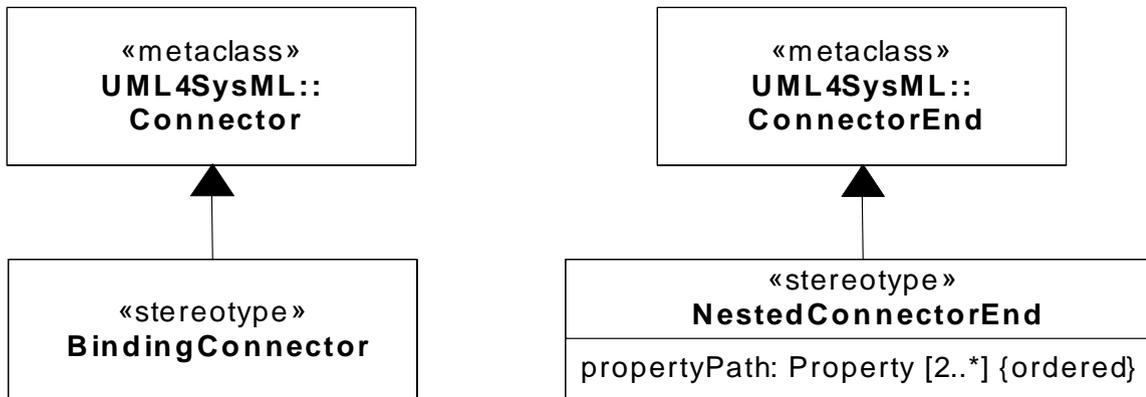
Figure 8.5 - Abstract syntax extensions for SysML connector ends
