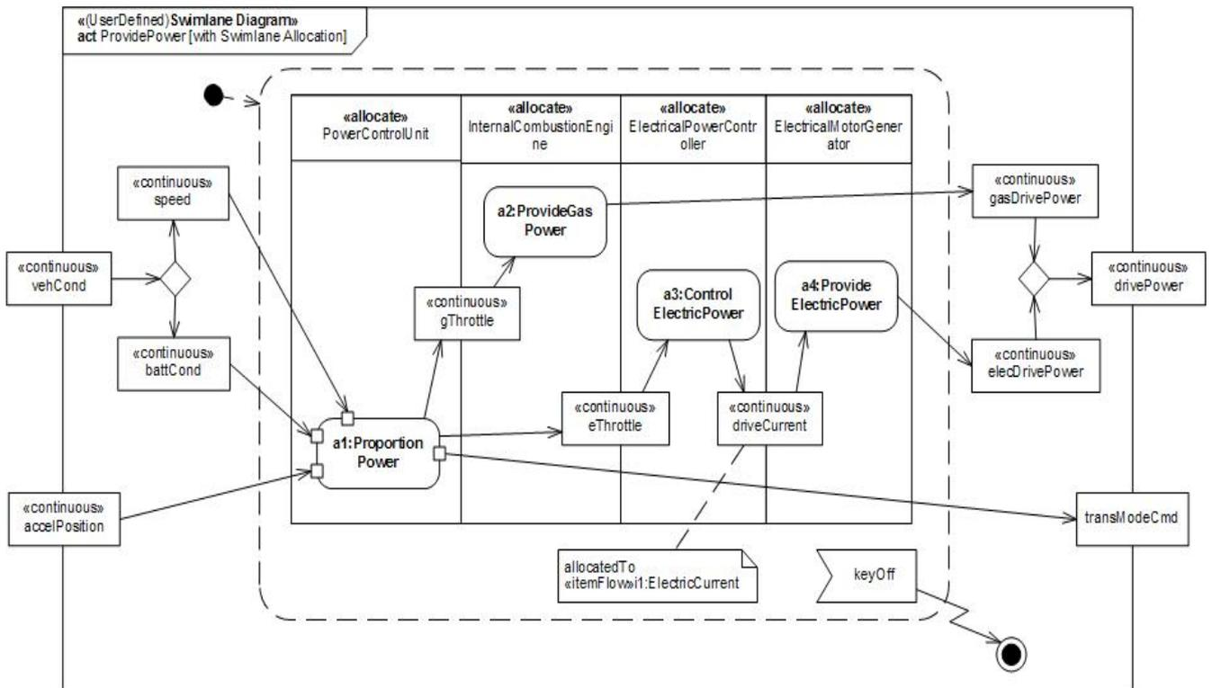
**Figure B.35 - Detailed Behavior Model for “Provide Power” (Activity Diagram)**
