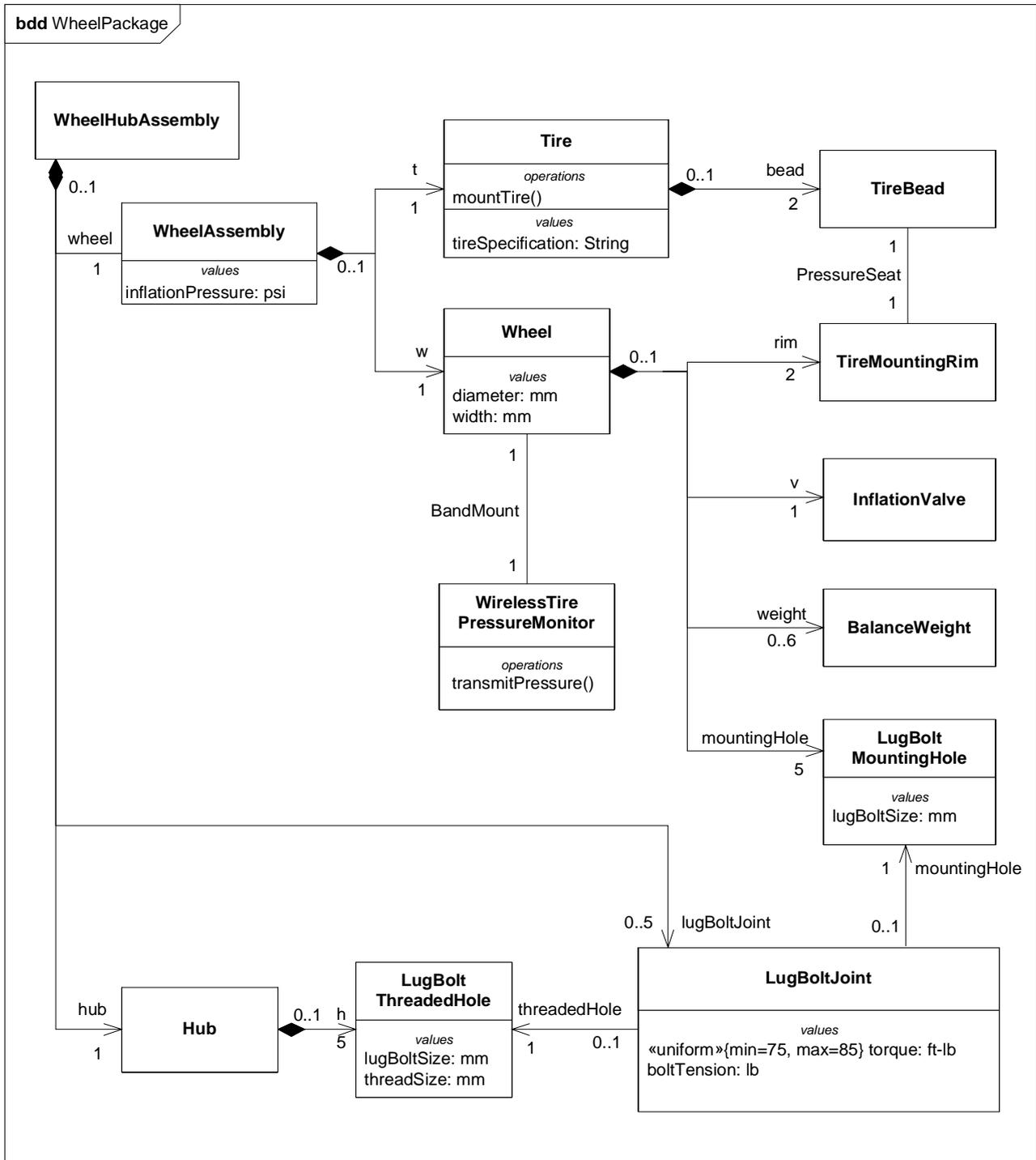
Figure 8.8 - Block diagram for the Wheel Package
