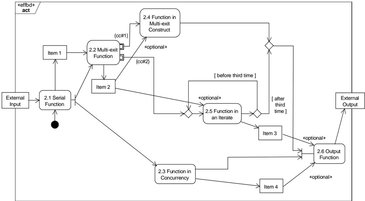
Figure C.1 - Example activity with «effbd» stereotype applied
