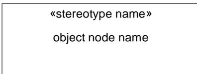
**Figure 11.7 - ObjectNode notation in activity diagrams**
