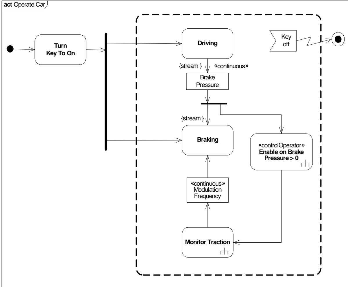
Figure 11.10 - Continuous system example 1.
