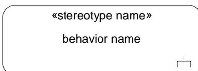
**Figure 11.2 - CallBehaviorAction notation with behavior stereotype**
