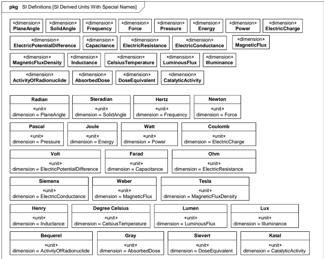
Figure C.7 - SI Derived Units With Special Names
