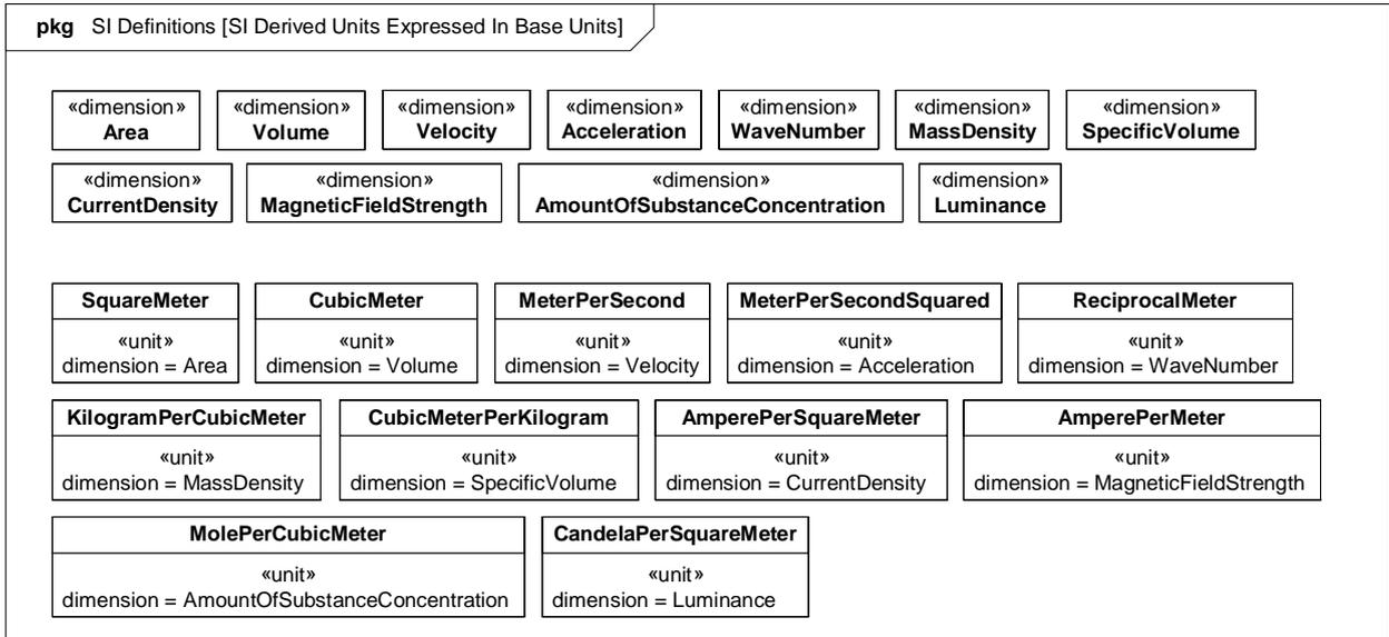
Figure C.6 - SI Derived Units Expressed In Base Units
