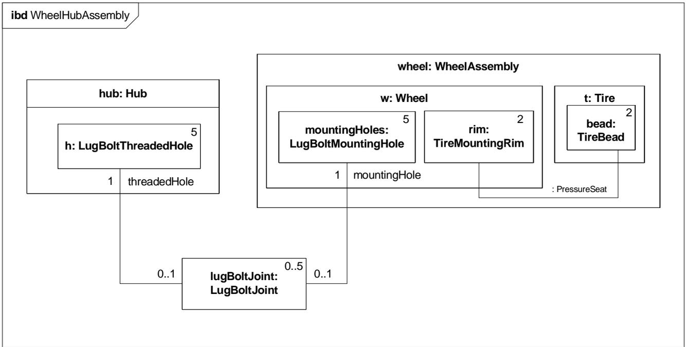
**Figure 8.9 - Internal Block Diagram for WheelHubAssembly**
