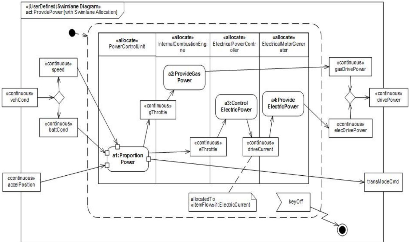
Figure 15.9 - AllocateActivityPartitions (Swimlanes) for HybridSUV Cellarette Example
