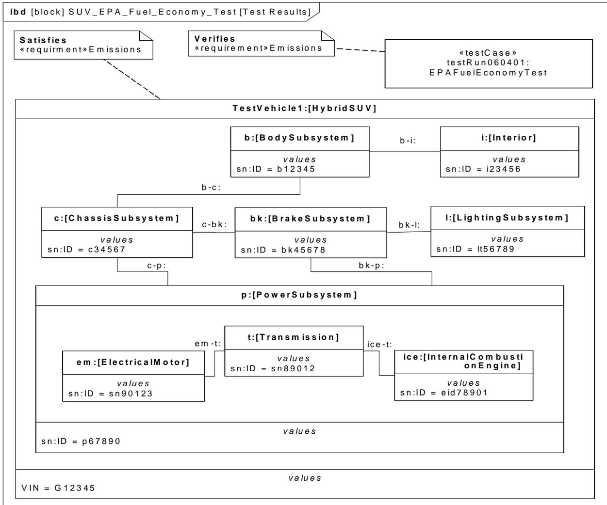
Figure B.38 - Special Case of Internal Block Diagram Showing Reference to Specific Properties (serial numbers)
