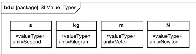
**Figure 8.10 - Defining Value Types with units and dimensions**
