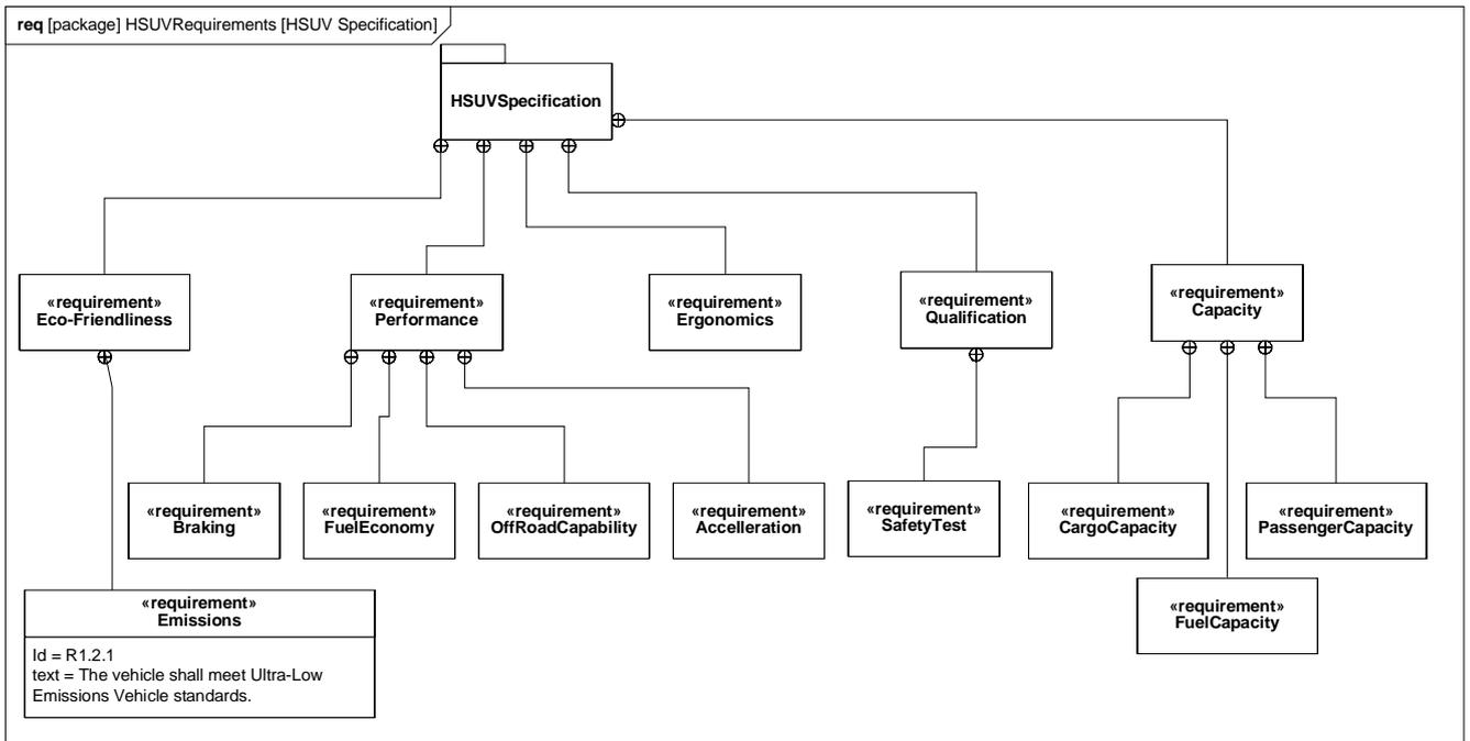
Figure B.11 - Establishing HSUV Requirements Hierarchy (containment) - (Requirements Diagram)
