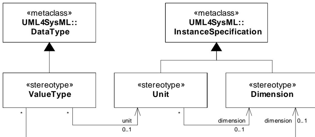
Figure 8.4 - Abstract syntax extensions for SysML value types
