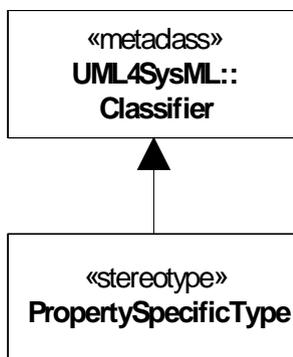
Figure 8.6 - Abstract syntax extensions for SysML property-specific types
