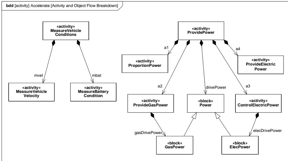
Figure B.34 - Decomposition of “Accelerate” Function (Block Definition diagram)
