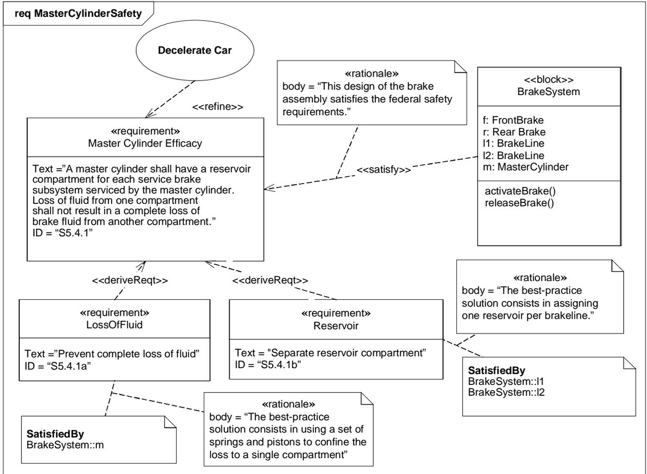
Figure 16.4 - Links between requirements and design
