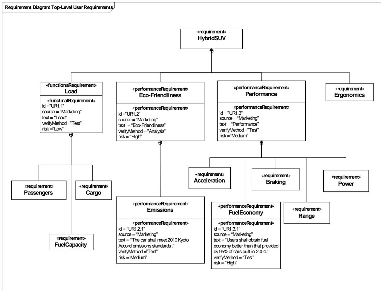
Figure C.3 - Example extensions to Requirement
