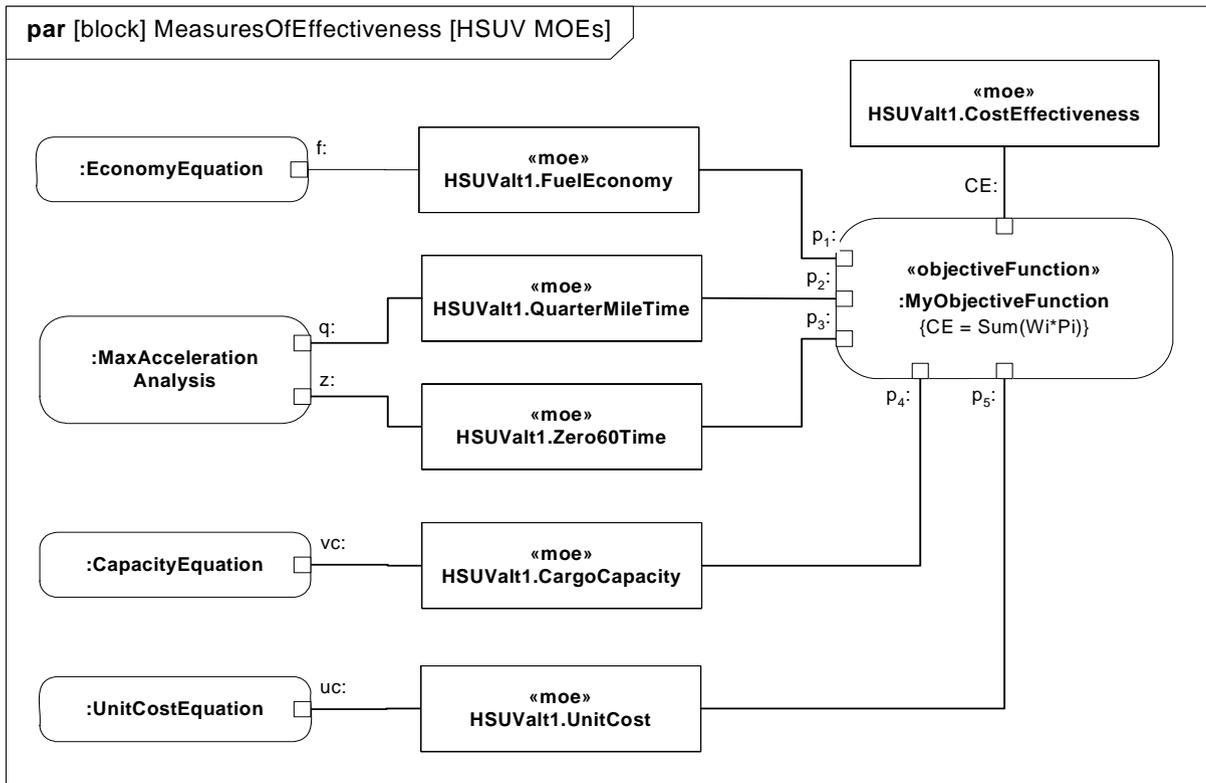
Figure B.28 - Defining Measures of Effectiveness and Key Relationships (Parametric Diagram)
