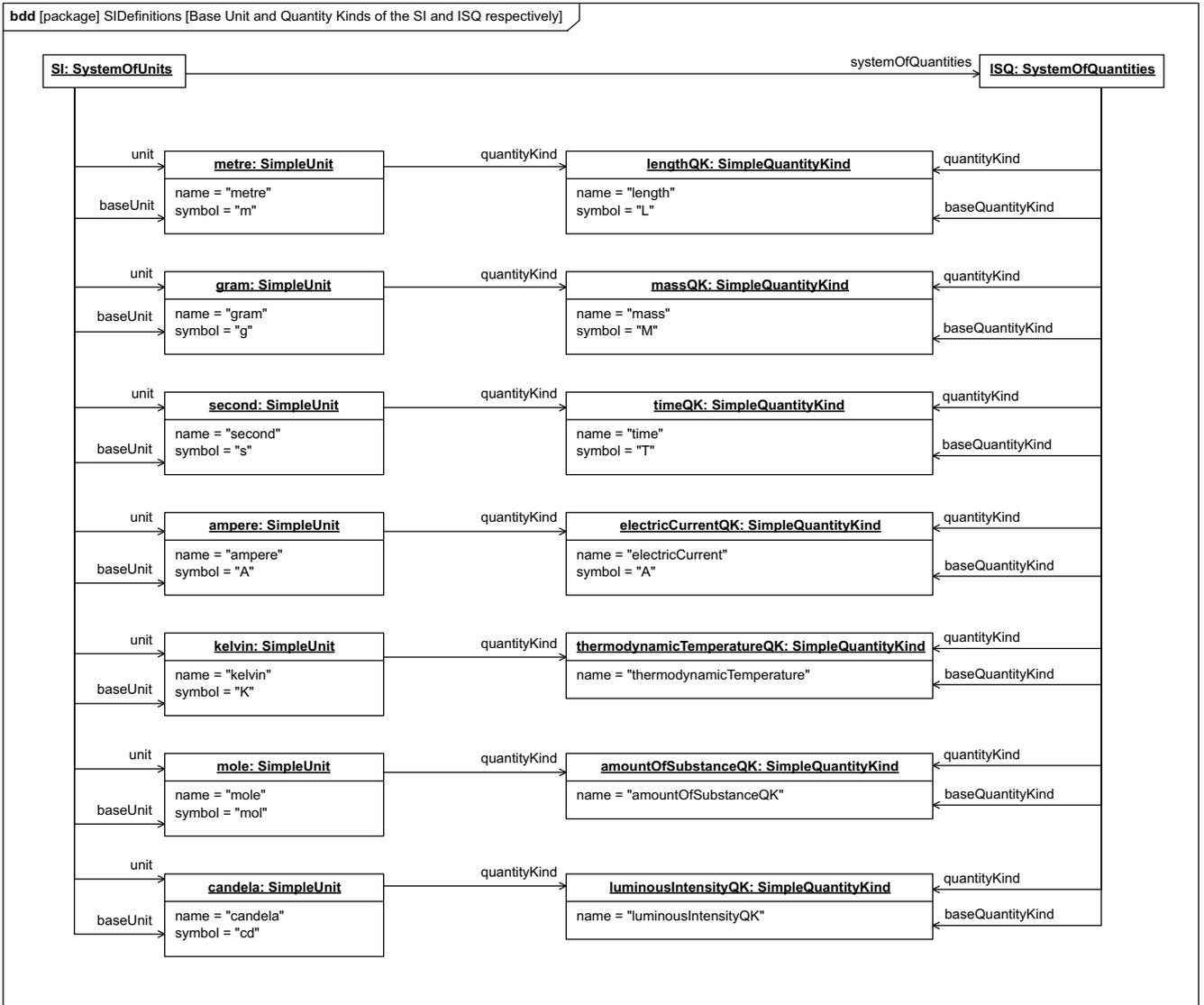
Figure C.11 - Base Unit and Quantity Kinds of the SI and ISQ respectively
