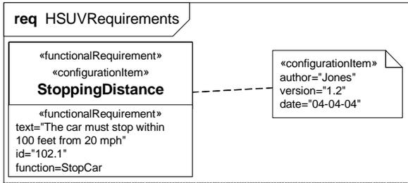
**Figure 17.9 - Using two stereotypes on a model element**
