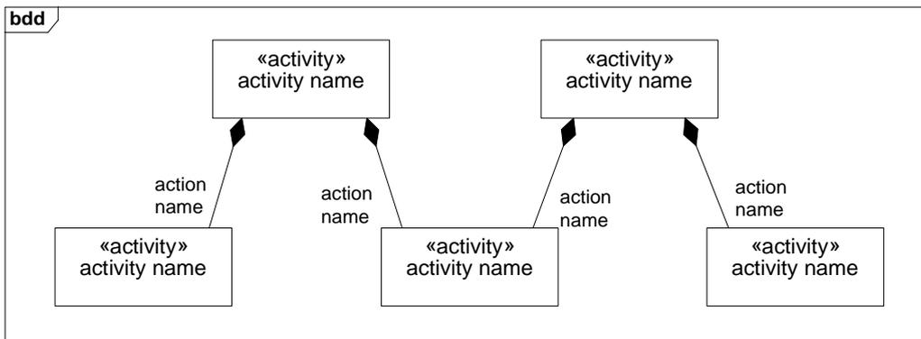
Figure 11.1 - Block definition diagram with activities as blocks
