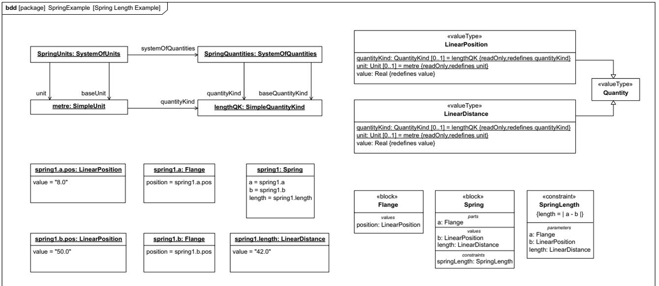
Figure C.13 - Spring Length Example
