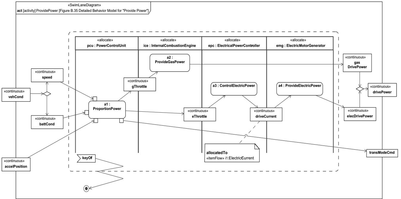
**Figure B.35 - Detailed Behavior Model for "Provide Power" (Activity Diagram)**
