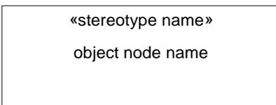
**Figure 11.7 - ObjectNode notation in activity diagrams**
