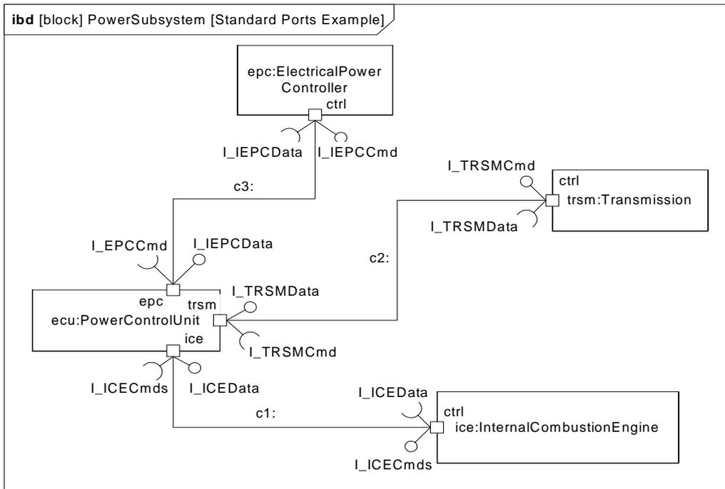
Figure 9.3 - Usage example of standard ports
