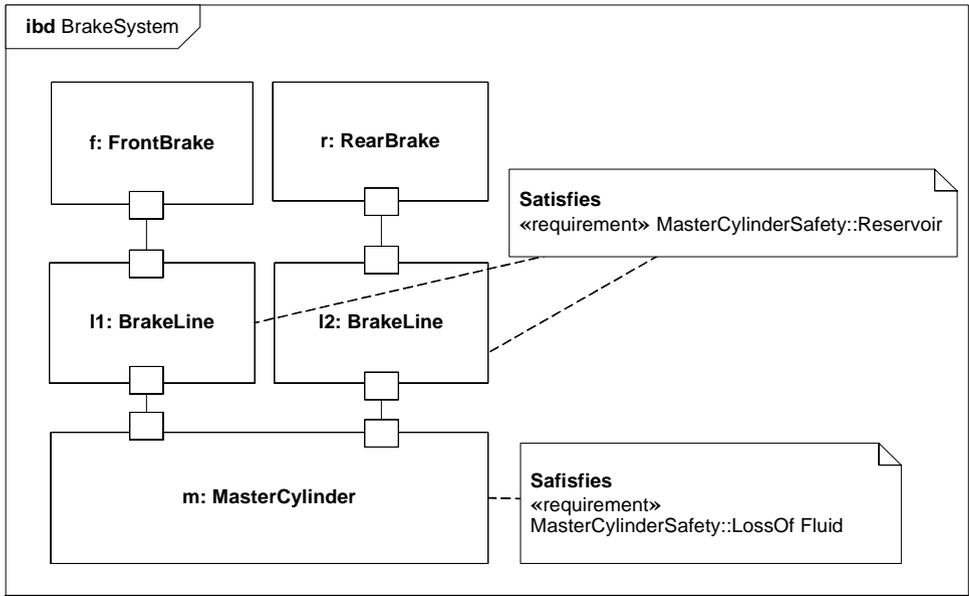
Figure 16.5 - Requirement satisfaction in an internal block diagram
