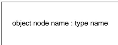
**Figure 11.6 - ObjectNode notation in activity diagrams**
