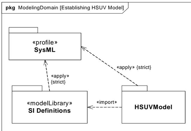
**Figure B.1 - Establishing the User Model by Importing and Applying SysML Profile & Model Library (Package Diagram)**
