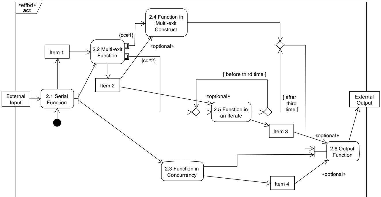
**Figure C.1- Example activity with «effbd» stereotype applied**
