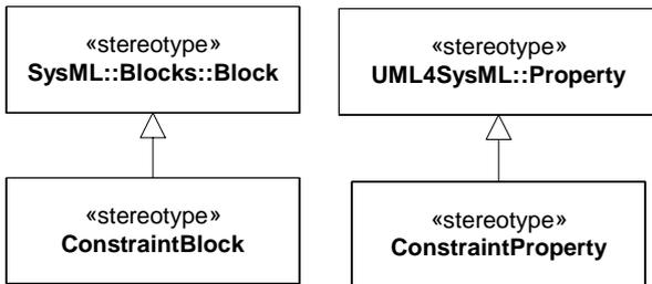
Figure 10.1 Stereotypes defined in SysML ConstraintBlocks package
