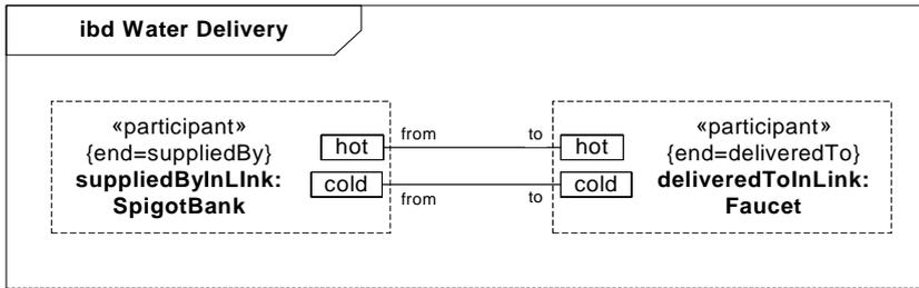
**Figure 8.12 - Internal structure of Water Delivery association block**
