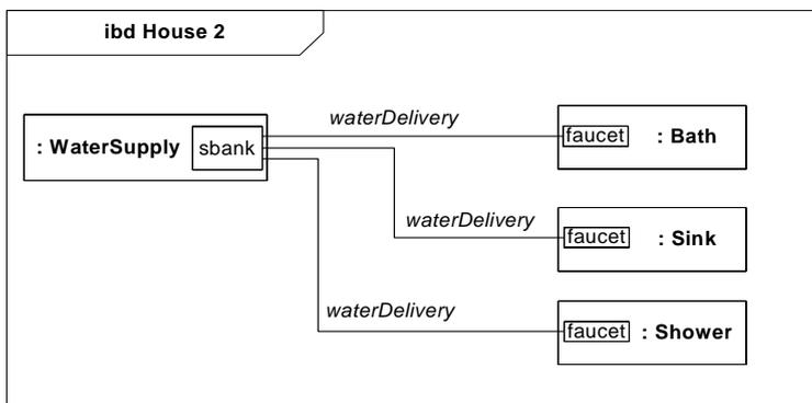
Figure 8.14 - Specializations of Water Client in house example
