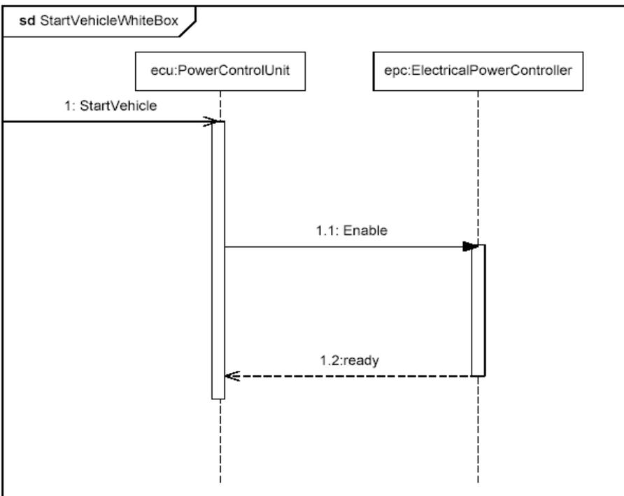
**Figure B.10 - White Box Interaction for “StartVehicle” (Sequence Diagram)**
