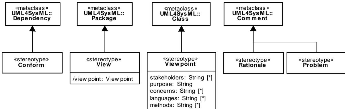
Figure 7.1 - Stereotypes defined in package ModelElements
