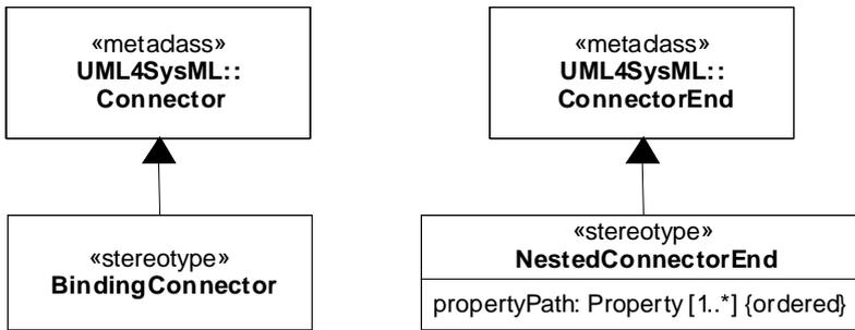
Figure 8.5 - Abstract syntax extensions for SysML connector ends
