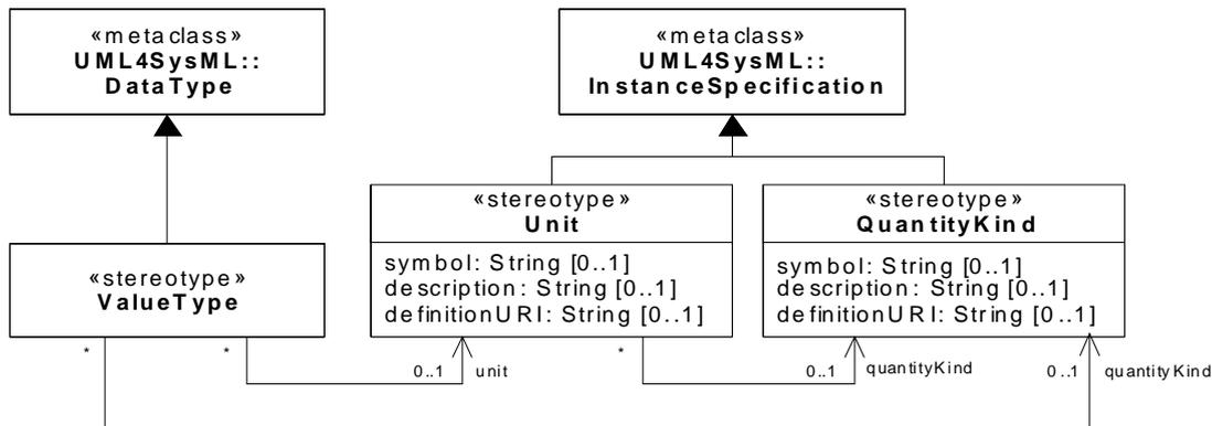
Figure 8.4 - Abstract syntax extensions for SysML value types
