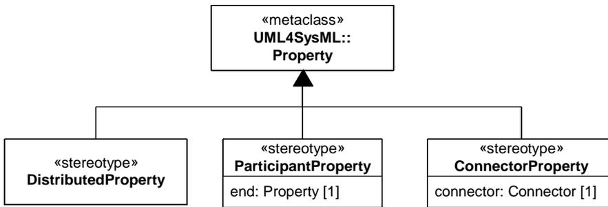
Figure 8.3 - Abstract syntax extensions for SysML properties
