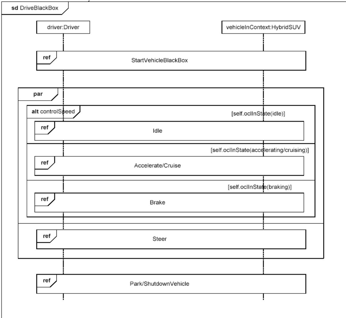
**Figure B.7 - Elaborating Black Box Behavior for the “Drive the Vehicle” Use Case (Sequence Diagram)**
