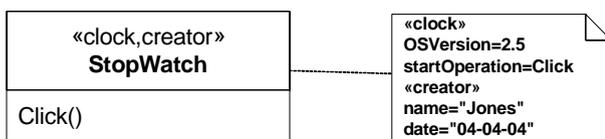
Figure 17.3 - Using stereotypes and showing values
