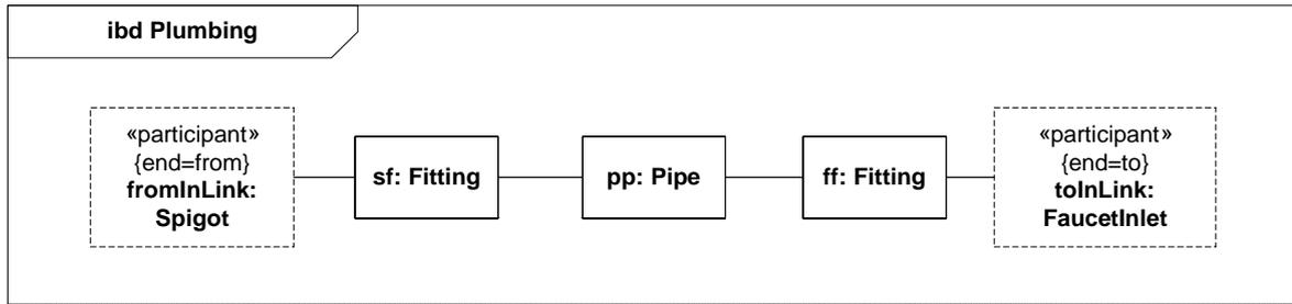
**Figure 8.16 - Internal structure of Plumbing association block**
