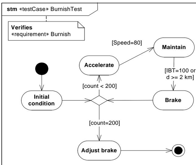
Figure 16.8 - Linkage of a Test Case to a requirement:
