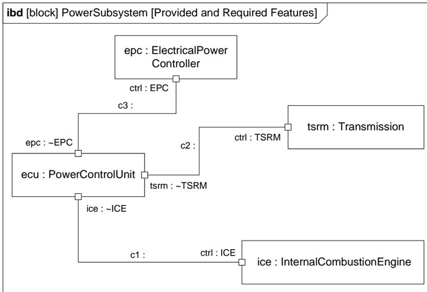
Figure 9.6 - Usage example of ports with provided and required features
