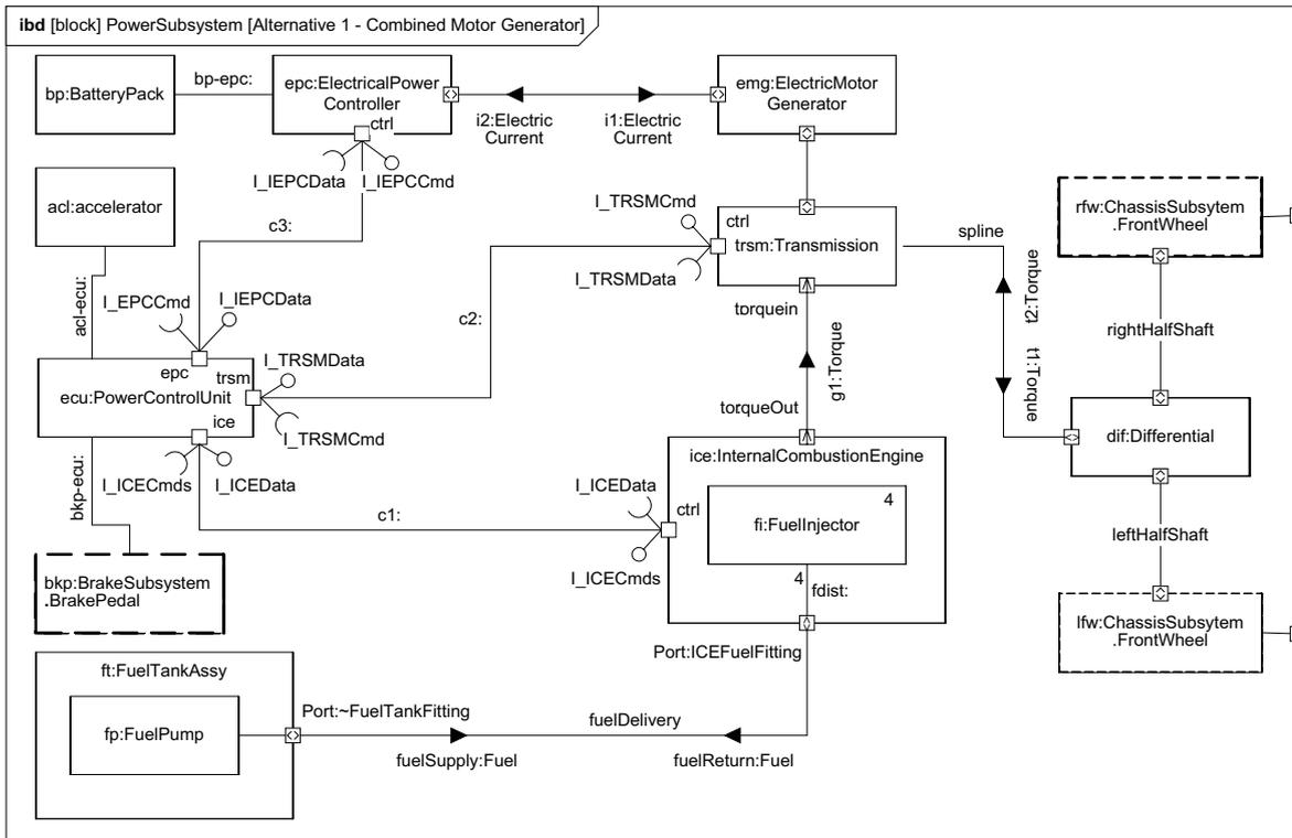
Figure C.19 - Internal Structure of the Power Subsystem (Internal Block Diagram)
