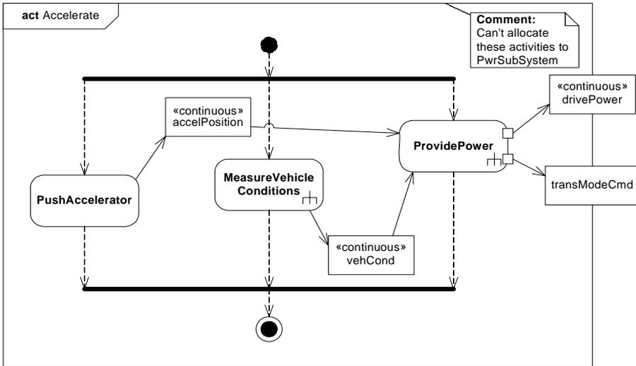
Figure C.33 - Behavior Model for “Accelerate” Function (Activity Diagram)
