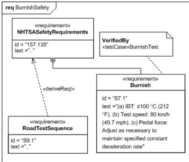
Figure 16.7 - Linkage of a Test Case to a requirement:
