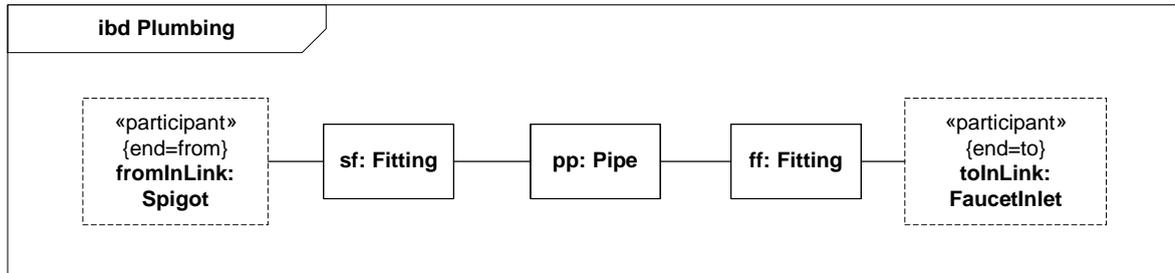
Figure 9.13 - Internal structure of Plumbing association block
