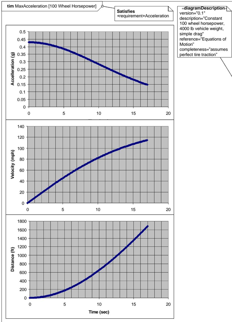
Figure C.32 - Results of Maximum Acceleration Analysis (Timing Diagram)
