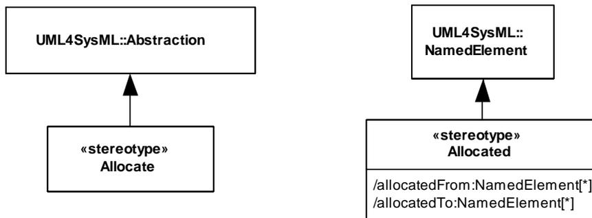
Figure 15.1 - Abstract syntax extensions for SysML Allocation
