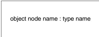
**Figure 11.6 - ObjectNode notation in activity diagrams**
