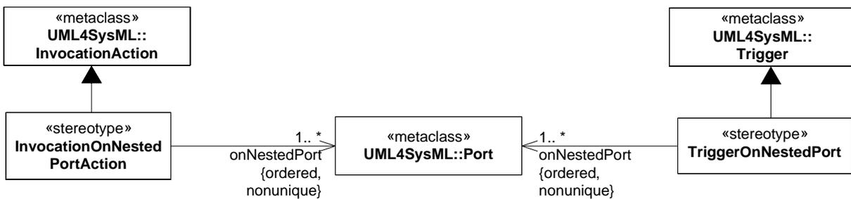
Figure 9.2 - Stereotypes for Actions on Nested Ports
