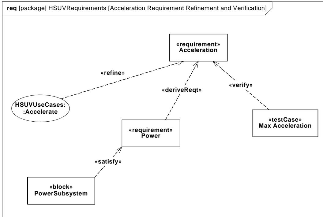
Figure C.13 - Acceleration Requirement Relationships (Requirements Diagram)
