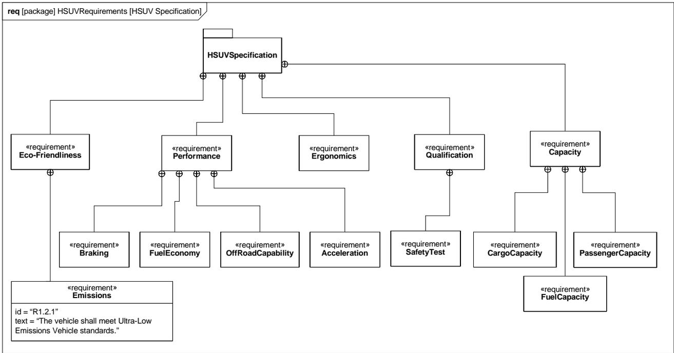
**Figure C.11 - Establishing HSUV Requirements Hierarchy (containment) - (Requirements Diagram)**
