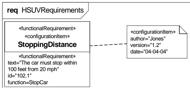
Figure 17.9 - Using two stereotypes on a model element
