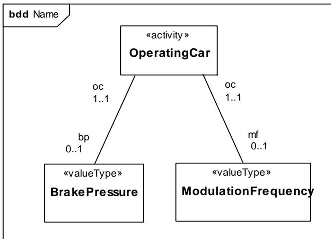
Figure 11.14 - Example block definition diagram for object node types
