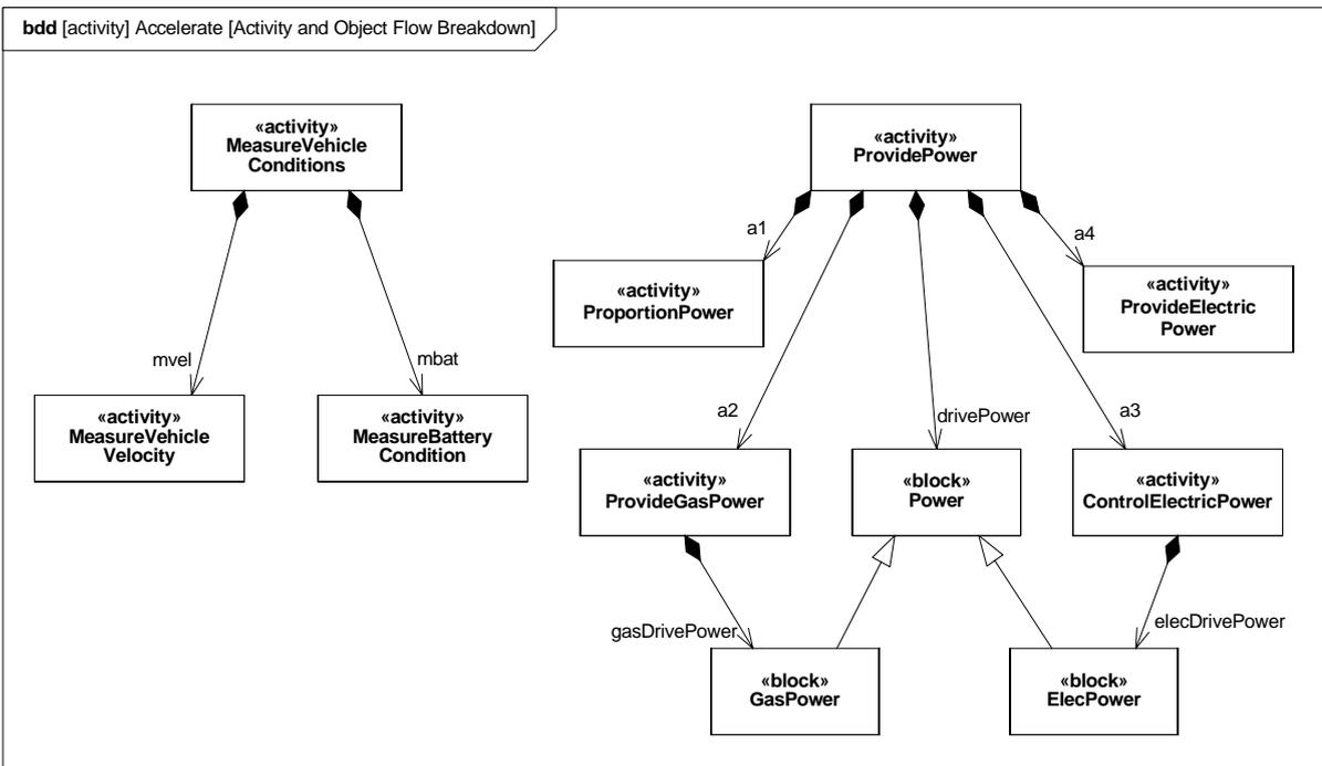
Figure C.34 - Decomposition of “Accelerate” Function (Block Definition diagram)
