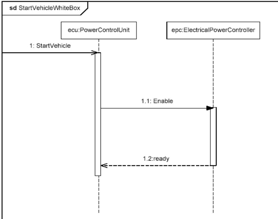
Figure C.10 - White Box Interaction for “StartVehicle” (Sequence Diagram)
