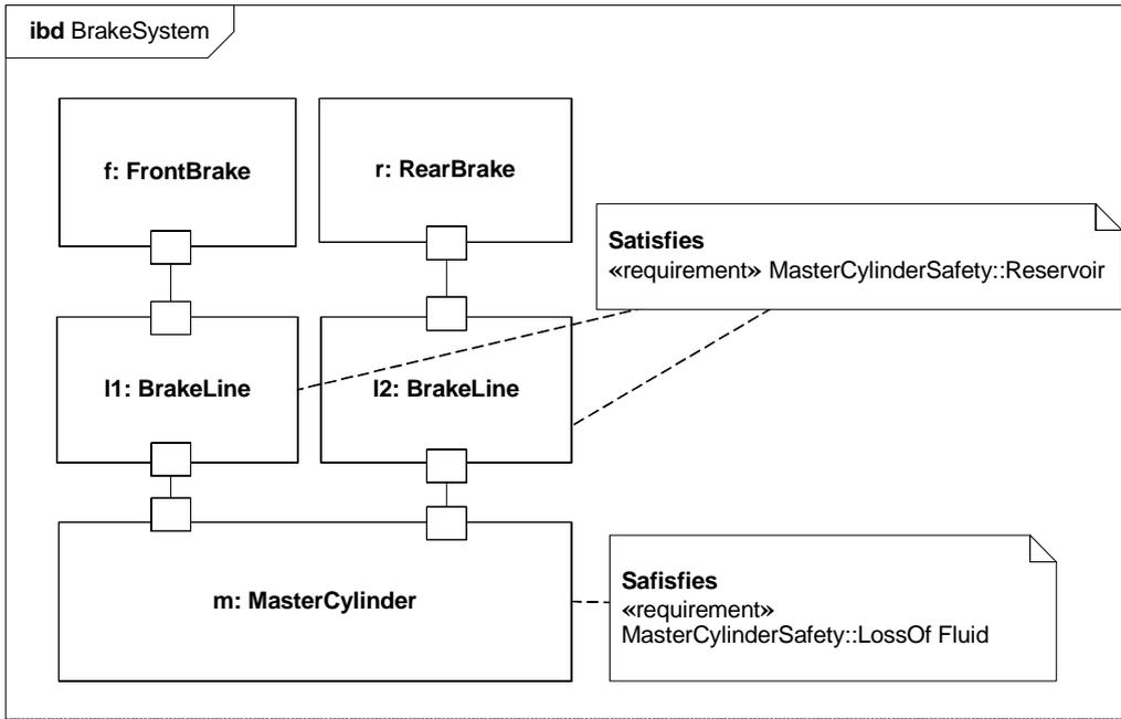
Figure 16.5 - Requirement satisfaction in an internal block diagram.
