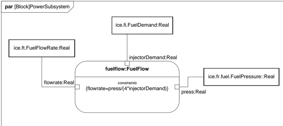
Figure C.24 - Defining Fuel Flow Constraints (Parametric Diagram)
