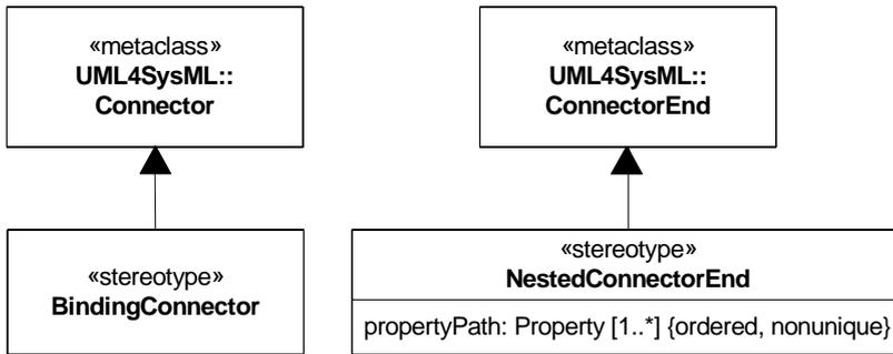
Figure 8.5 - Abstract syntax extensions for SysML connector ends
