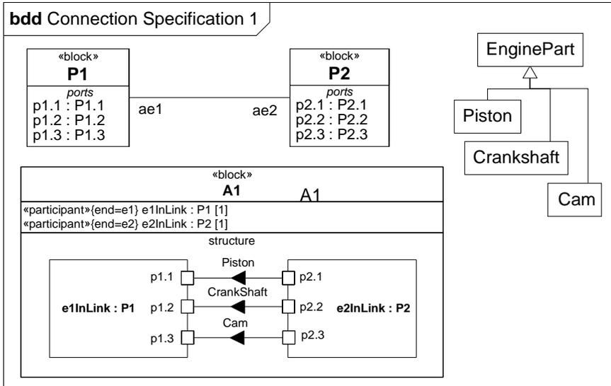
Figure 9.16 - Usage example of item flow decomposition
