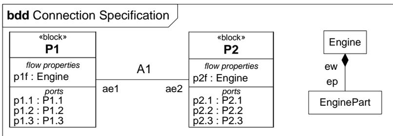
Figure 9.17 - Usage example of item flow decomposition
