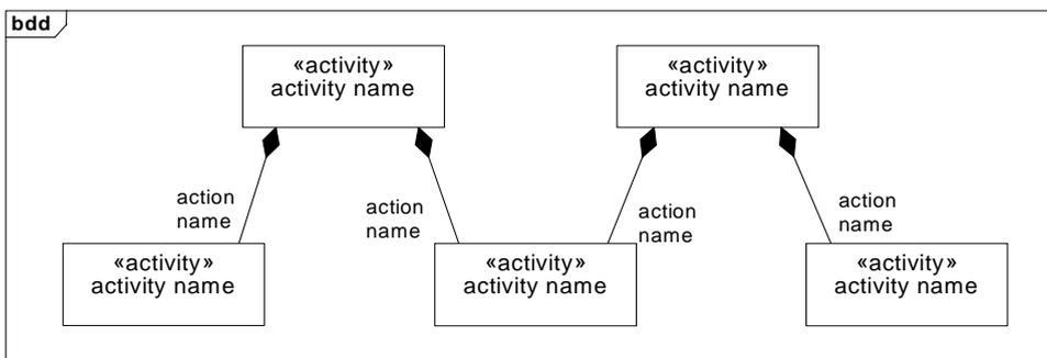
Figure 11.1 - Block definition diagram with activities as blocks
