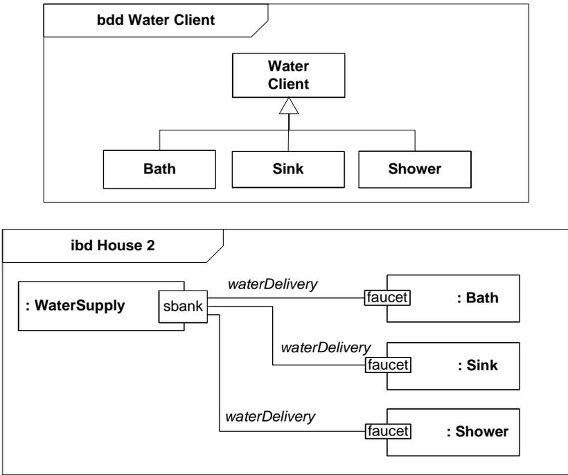
**Figure 9.11 - Specializations of Water Client in house example**
