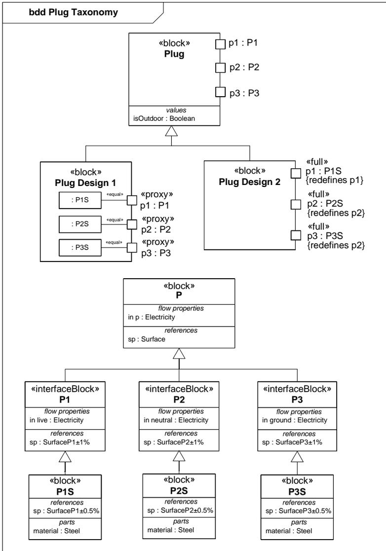
Figure 9.7 Usage example of proxy and full ports
