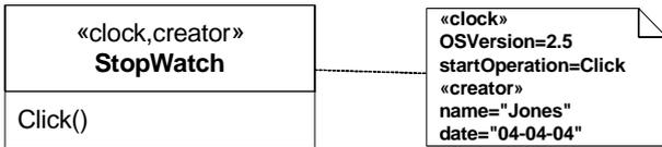
Figure 17.3 - Using stereotypes and showing values
