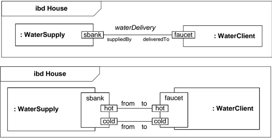
**Figure 9.10 - Two views of Water Delivery connector within House block**
