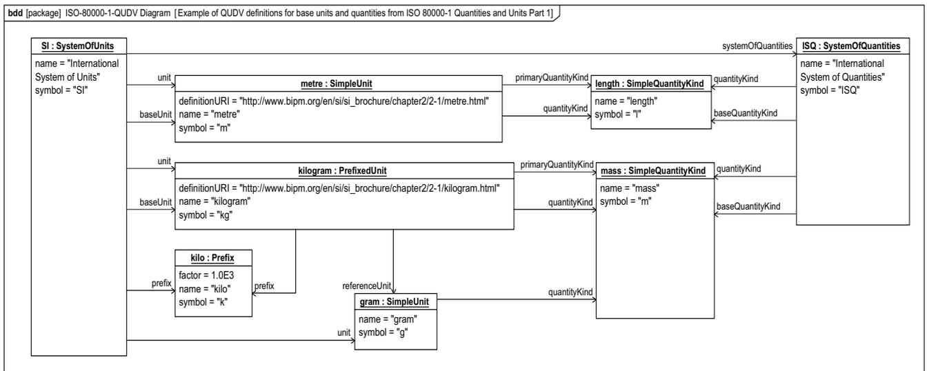
Figure D.11 - Base Unit and Quantity Kinds of the SI and ISQ respectively
