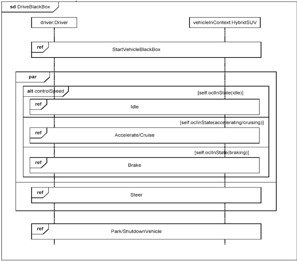
Figure C.7 - Elaborating Black Box Behavior for the “Drive the Vehicle” Use Case (Sequence Diagram)
