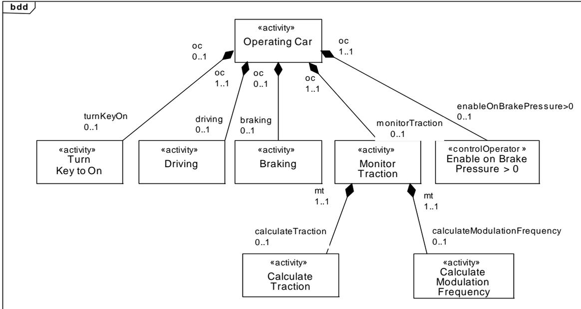
Figure 11.13 - Example block definition diagram for activity decomposition
