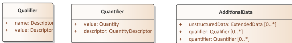
Figure 8.4 Structs (Class diagram)
