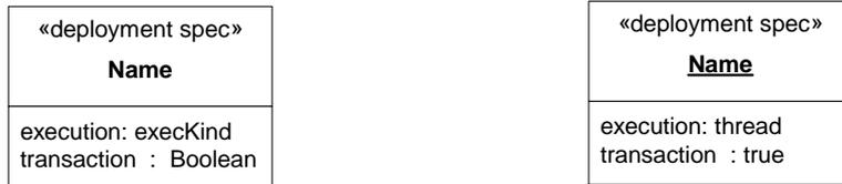
Figure 133 - A DeploymentSpecification for an artifact (specification and instance levels)
