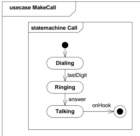
Figure 405 - Example of a use case with an associated state machine behavior
