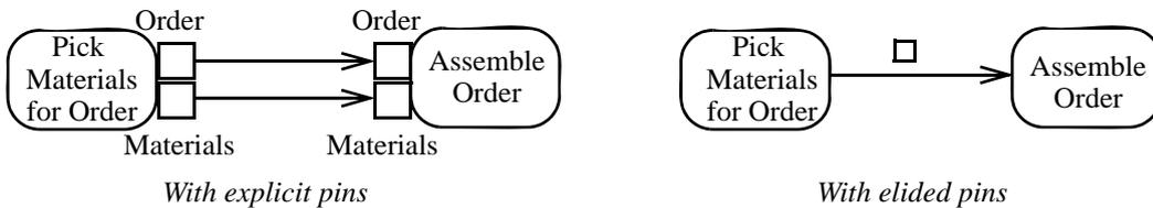
Figure 285 - Eliding objects flowing on the edge
