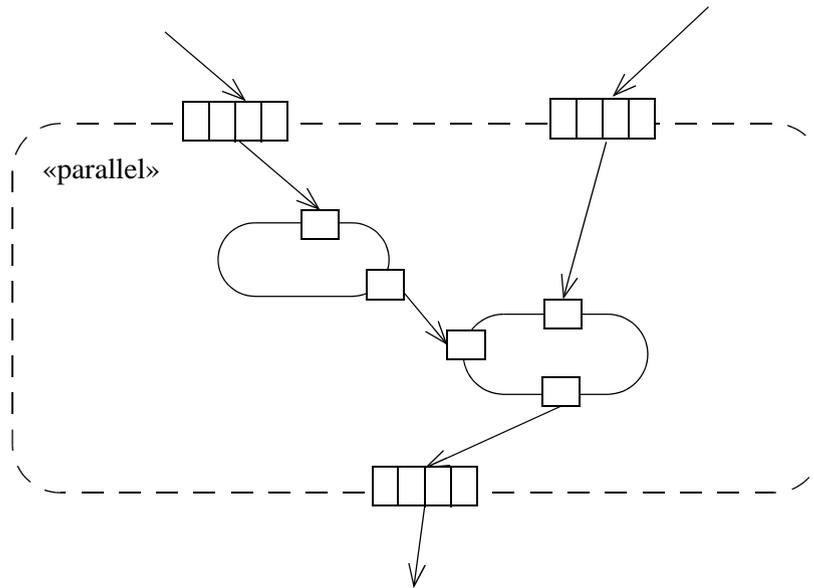
Figure 260 - Expansion region with 2 inputs and 1 output
