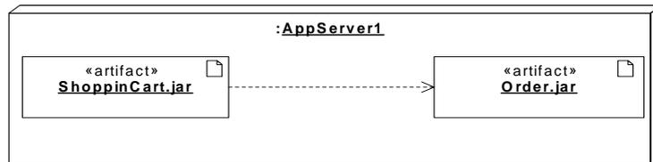
Figure 140 - A set of deployed component artifacts on a Node
