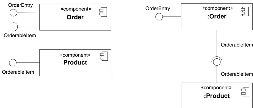
**Figure 92 - An assembly connector maps a required interface of a component to a provided interface of another component in a certain context (definition of components e.g. in a library on the left, an assembly of those components on the right).**
