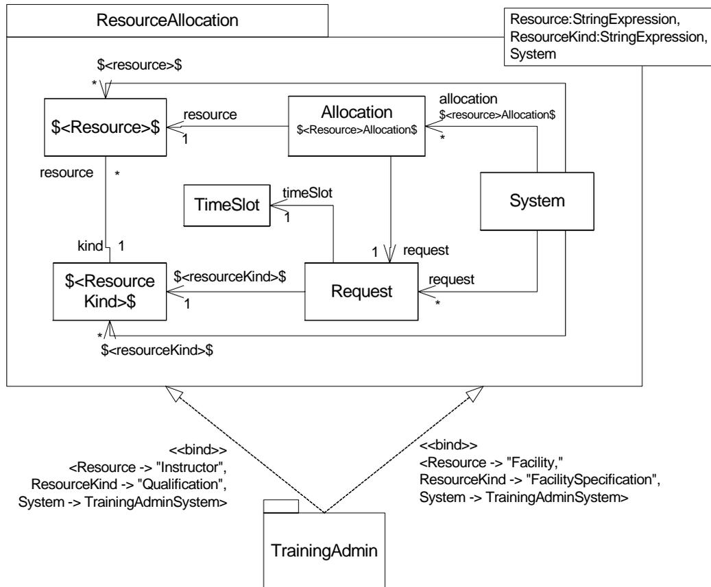
Figure 439 - Template Package with string parameters
