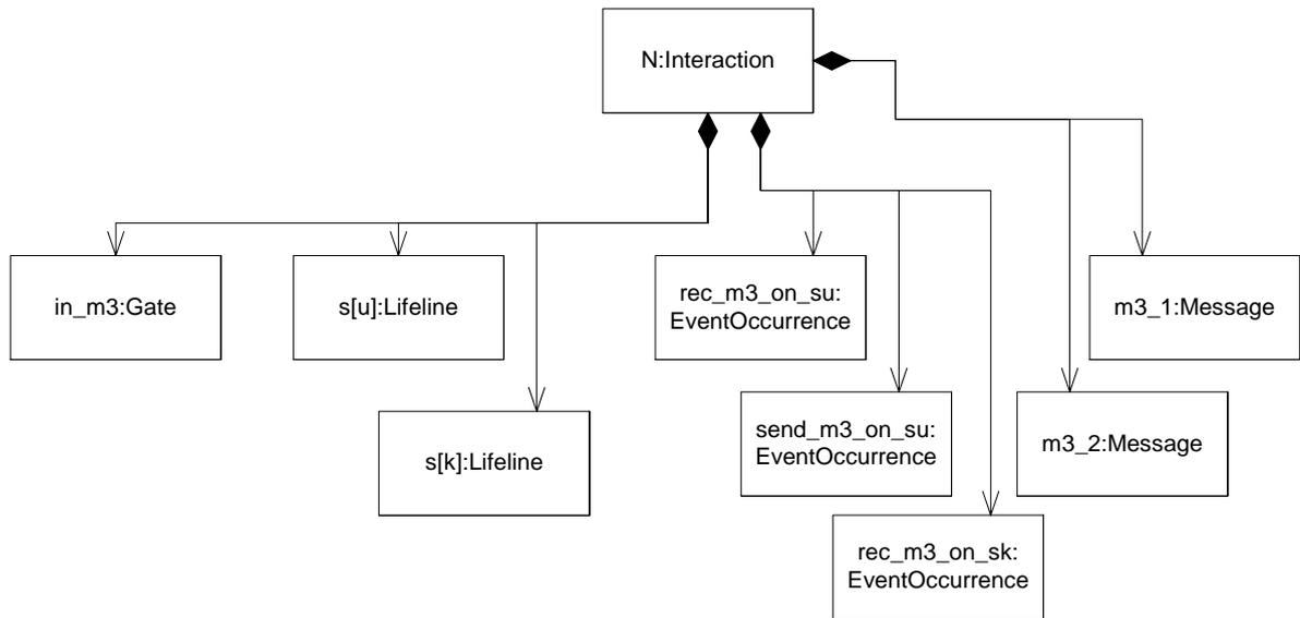
**Figure 347 - Metamodel elements of a sequence diagram**
