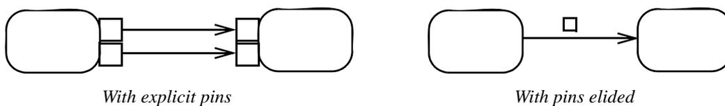
**Figure 283 - Eliding objects flowing on the edge**
