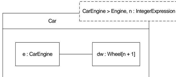
**Figure 432 - Template Class with a constrained class parameter**
