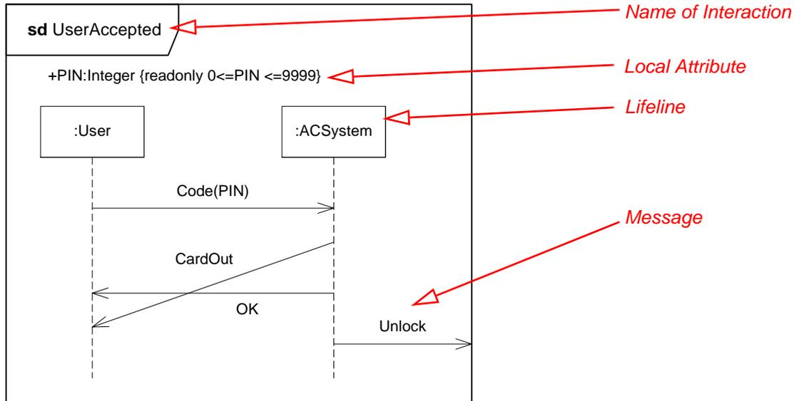
Figure 340 - An example of an Interaction in the form of a Sequence Diagram
