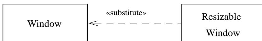
Figure 72 - An example of a substitute dependency
