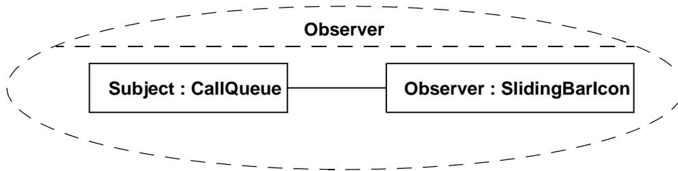
**Figure 104 - The internal structure of the Observer collaboration shown inside the collaboration icon (a connection is shown between the Subject and the Observer role).**
