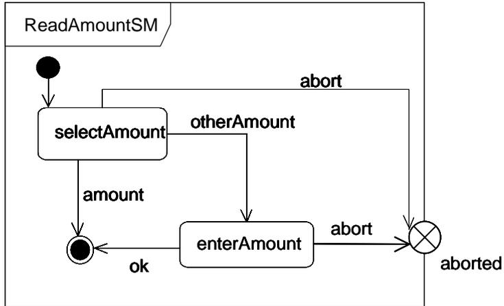
Figure 399 - State machine with exit point definition
