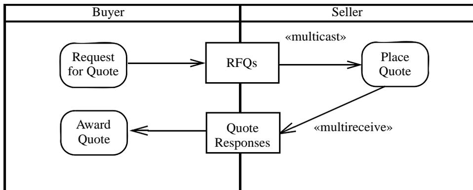
Figure 287 - Specifying multicast and multireceive on the edge
