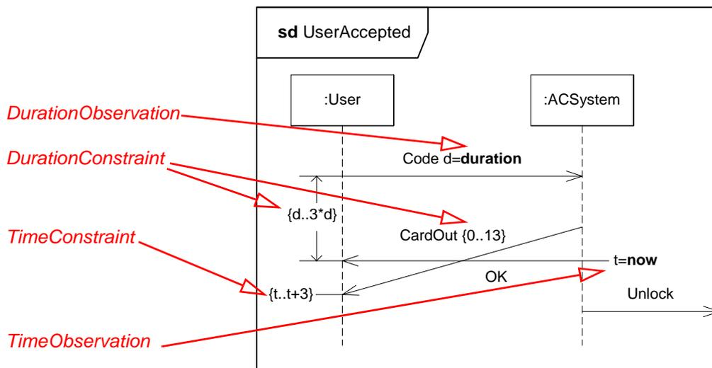
**Figure 350 - Sequence Diagram with time and timing concepts**
