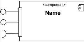
A rectangular box representing a component. Inside the box, the text «component» is at the top, followed by the word "Name" in bold. On the right side of the box is a small icon of a component. On the left side, there is a vertical bar representing a complex port, with three semi-circular shapes (two provided and one required) attached to it. | See “Port”.      |
