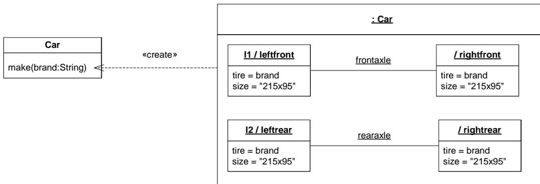
Figure 121 - A constructor for the Car class
