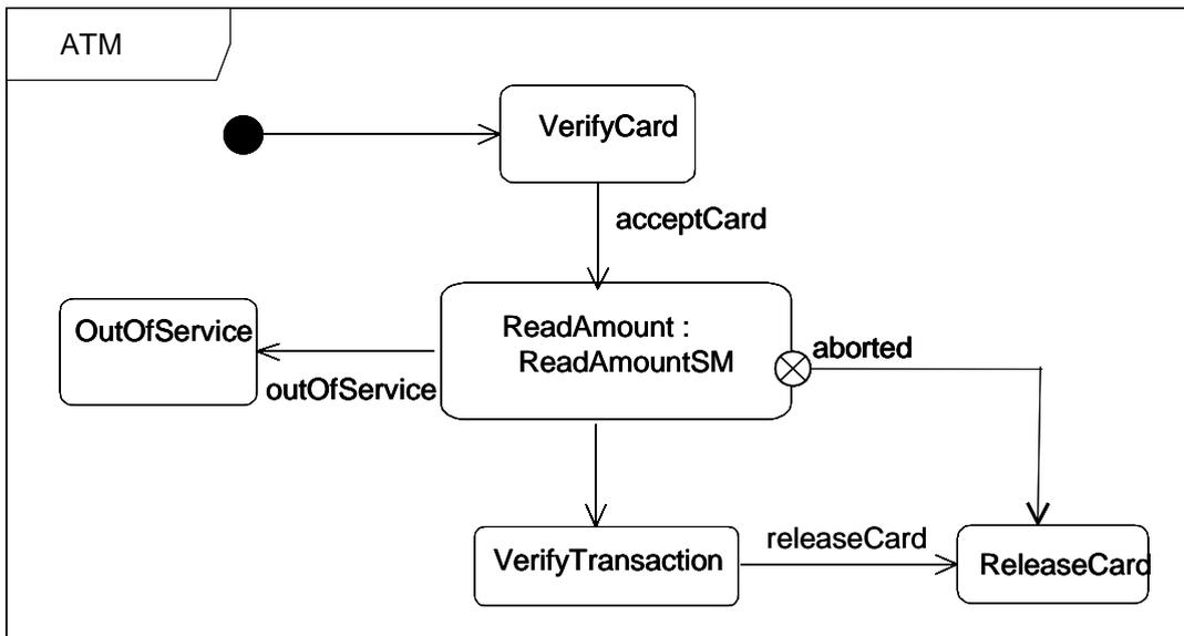
Figure 400 - SubmachineState with usage of exit point
