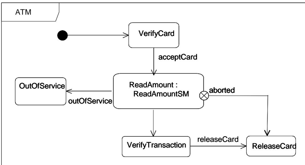
Figure 391 - SubmachineState with usage of exit point
