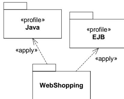
Figure 455 - Profiles applied to a package
