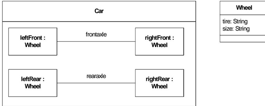
**Figure 118 - Connectors and parts in a structure diagram**
