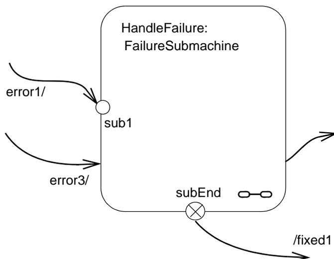
**Figure 388 - Submachine State**
