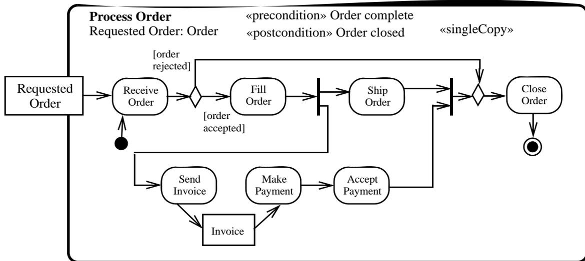
Figure 209 - Example of an activity with input parameter
