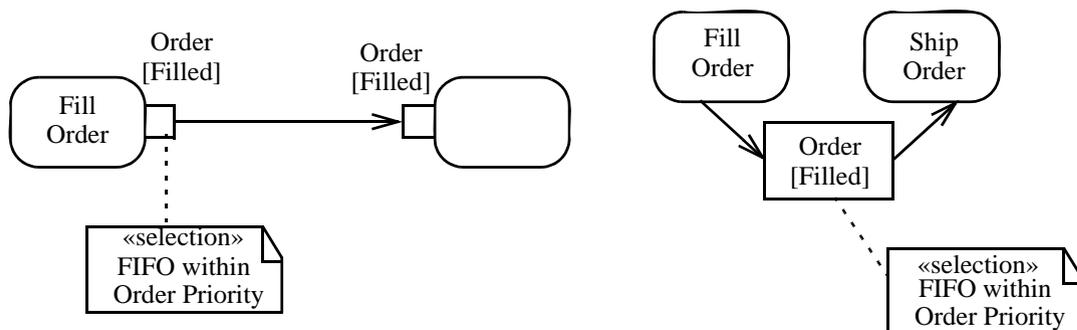
Figure 304 Specifying selection behavior on an ObjectFlow
