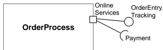
**Figure 112 - Port notation showing multiple provided interfaces**
