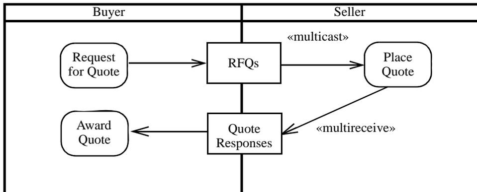
Figure 12.113 - Specifying multicast and multireceive on the edge
