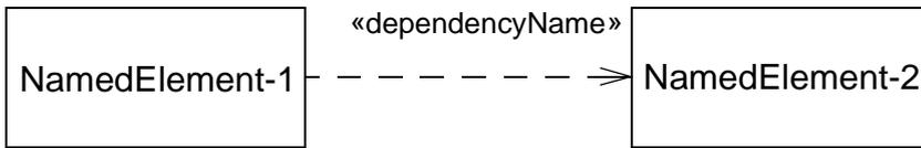
Figure 7.37 - Notation for a dependency between two elements
