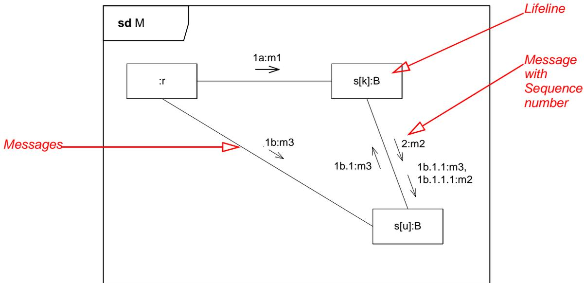
Figure 14.27 - Communication diagram
