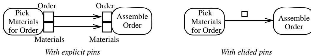
Figure 12.111 - Eliding objects flowing on the edge
