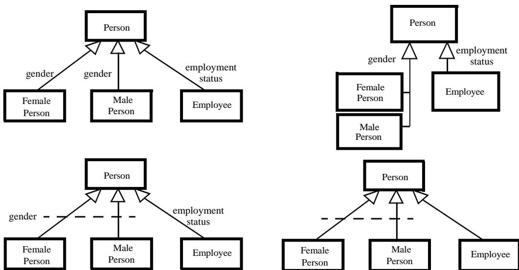
Figure 7.44 - Multiple subtype partitions (GeneralizationSets) example
