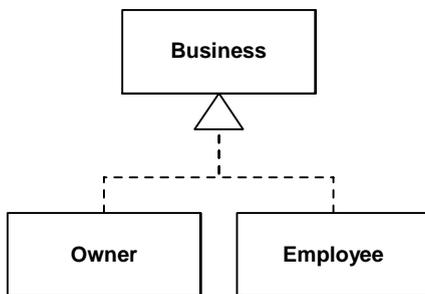
Figure 7.73 - An example of a realization dependency
