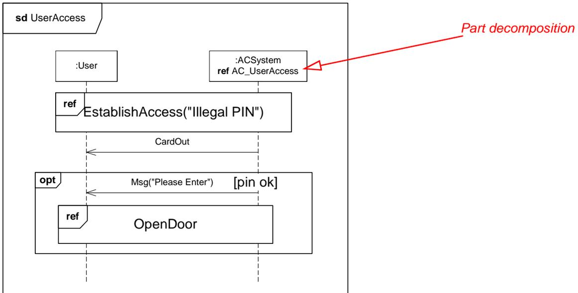
**Figure 14.20 - Part Decomposition - the decomposed part**
