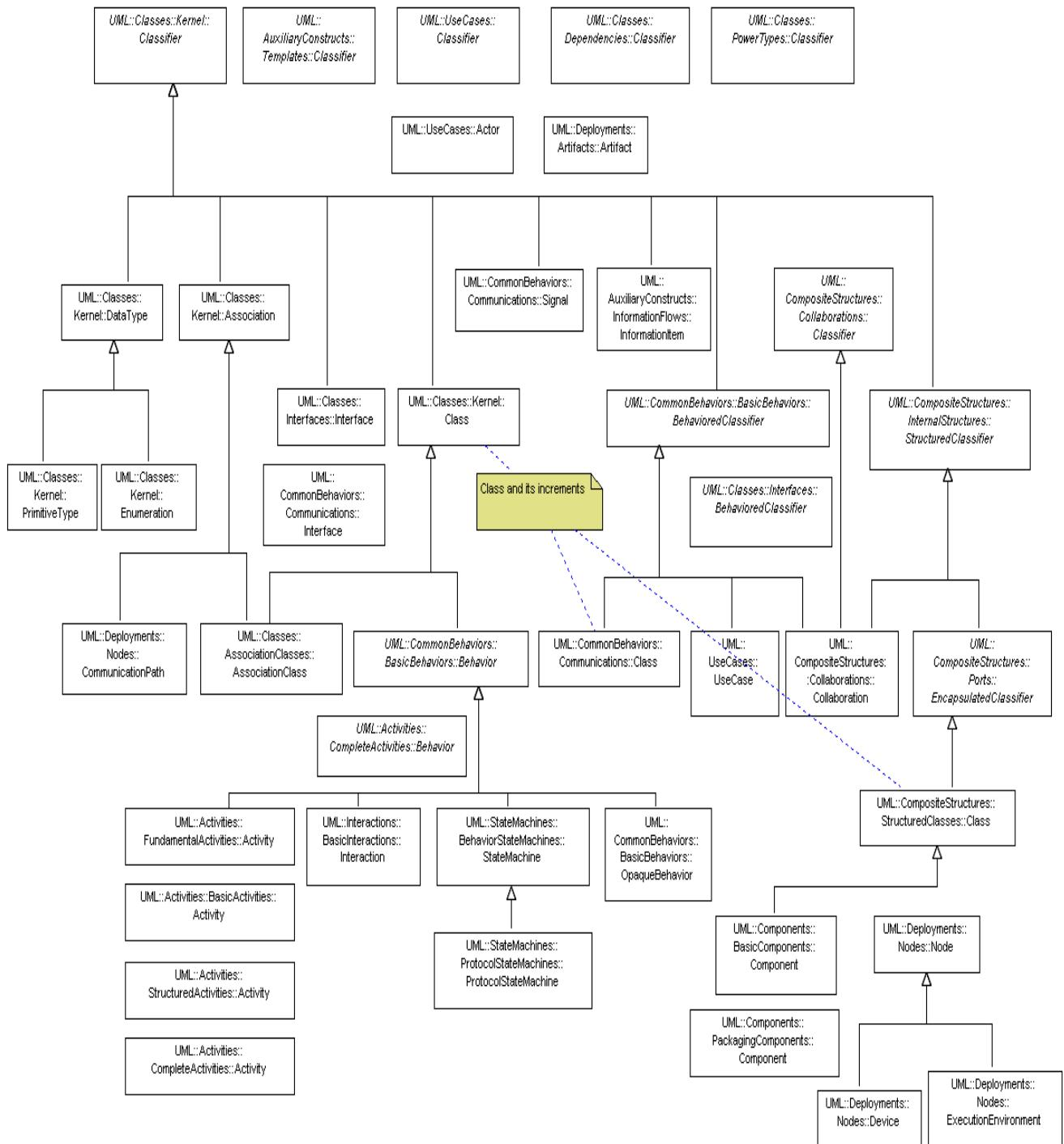
**Figure F.1 - Classifier hierarchy for UML 2.0 Superstructure**
