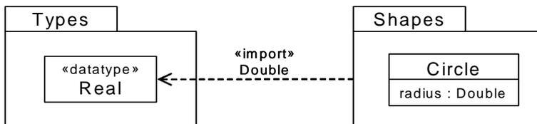
Figure 7.40 - Example of element import with aliasing
