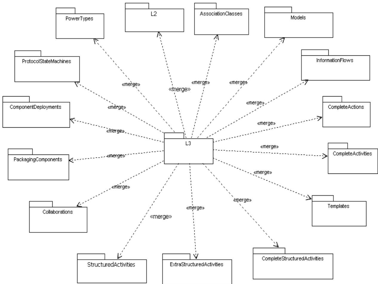
Figure 2.4 - Level 3 top-level package merges
