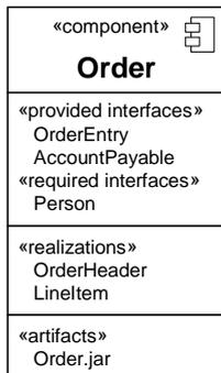
**Figure 8.9 - A white-box representation of a component**
