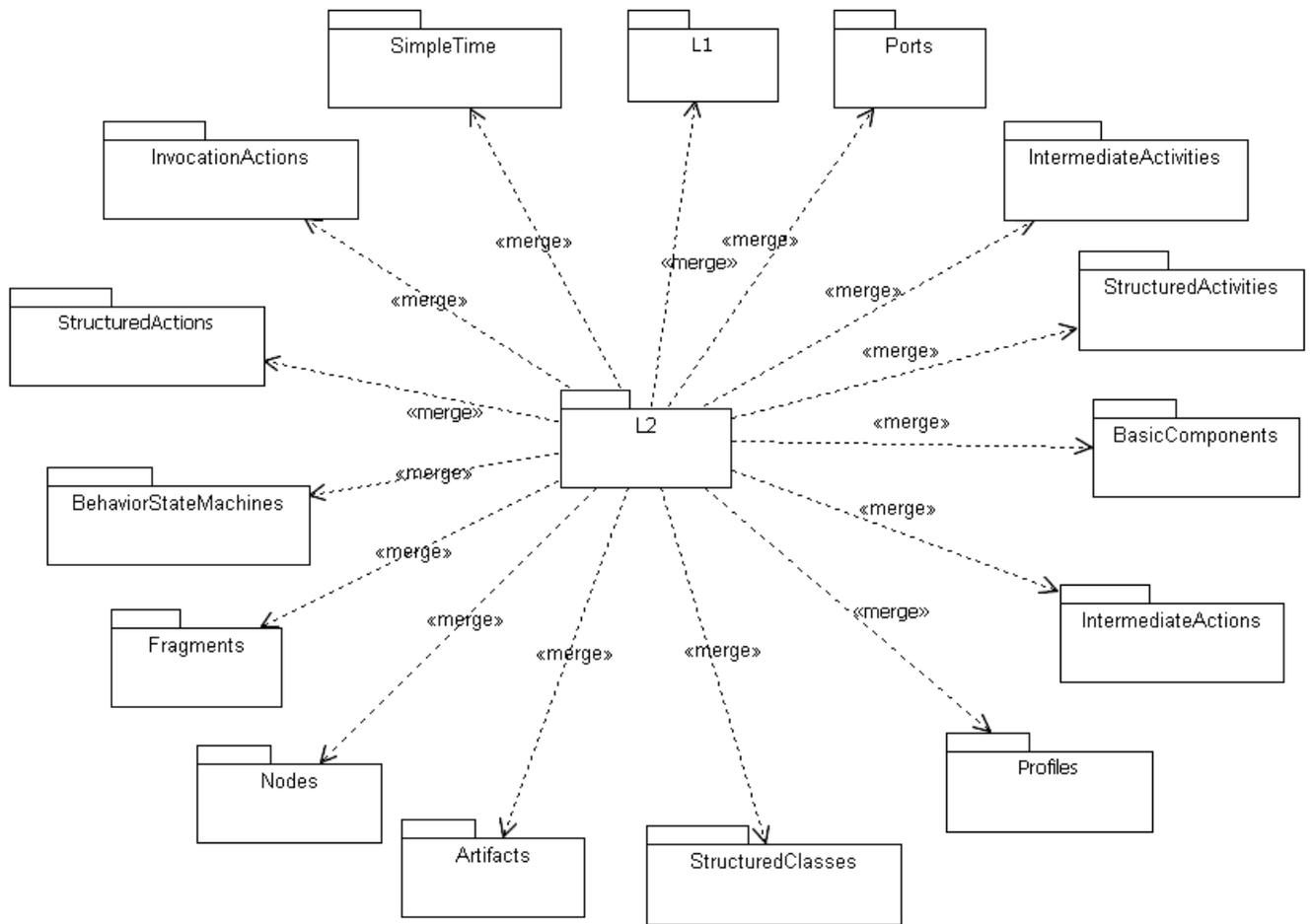
**Figure 2.3 - Level 2 top-level package merges**
