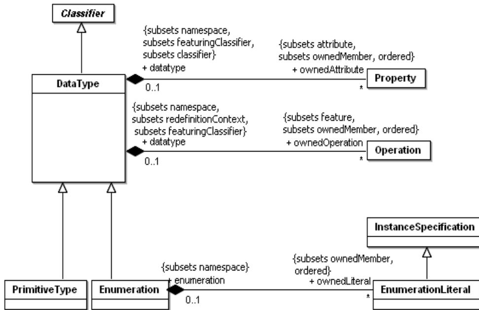
Figure 7.13 - DataTypes diagram of the Kernel package
