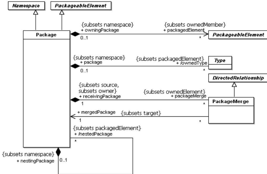
Figure 7.14 - The Packages diagram of the Kernel package
