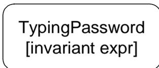
**Figure 15.40 - State with invariant - notation**
