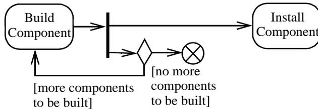
**Figure 12.93 - Flow final example without merge edge**
