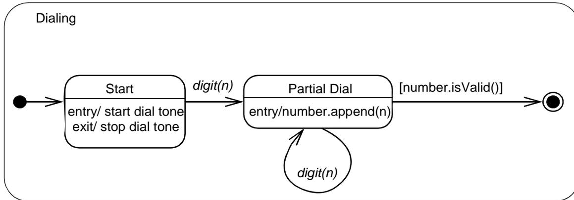
Figure 15.33 - Composite state with two states
