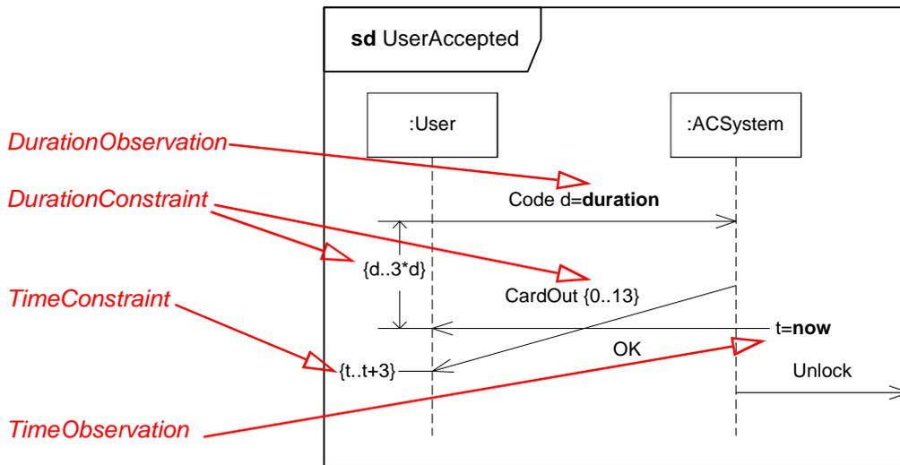
**Figure 14.26 - Sequence Diagram with time and timing concepts**
