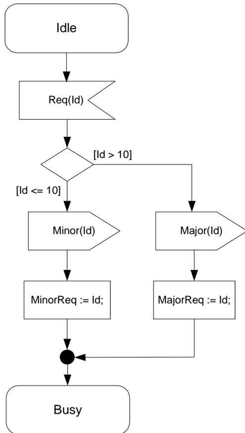
**Figure 15.44 - Symbols for Signal Receipt, Sending and Actions on transition**
