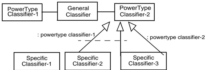
(b) Power type specification using dashed-line notation
