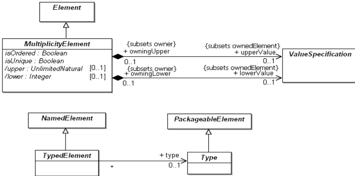
Figure 7.5 - Multiplicities diagram of the Kernel package
