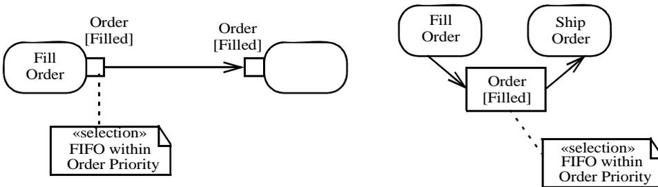
**Figure 12.130 - Specifying selection behavior on an ObjectFlow**
