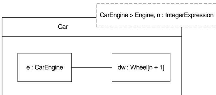
**Figure 17.21 - Template Class with a constrained class parameter**
