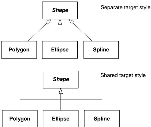
Figure 7.43 - Examples of generalizations between classes
