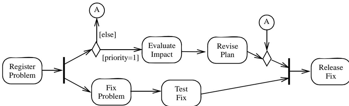
Figure 12.43 - Connector example
