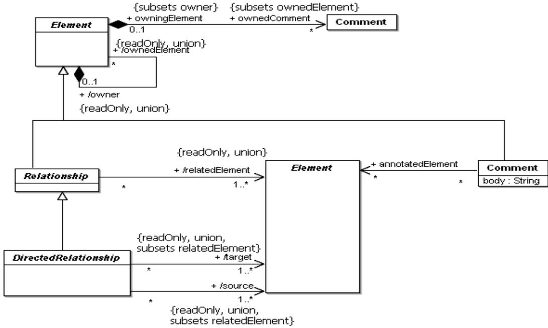
Figure 7.3 - Root diagram of the Kernel package
