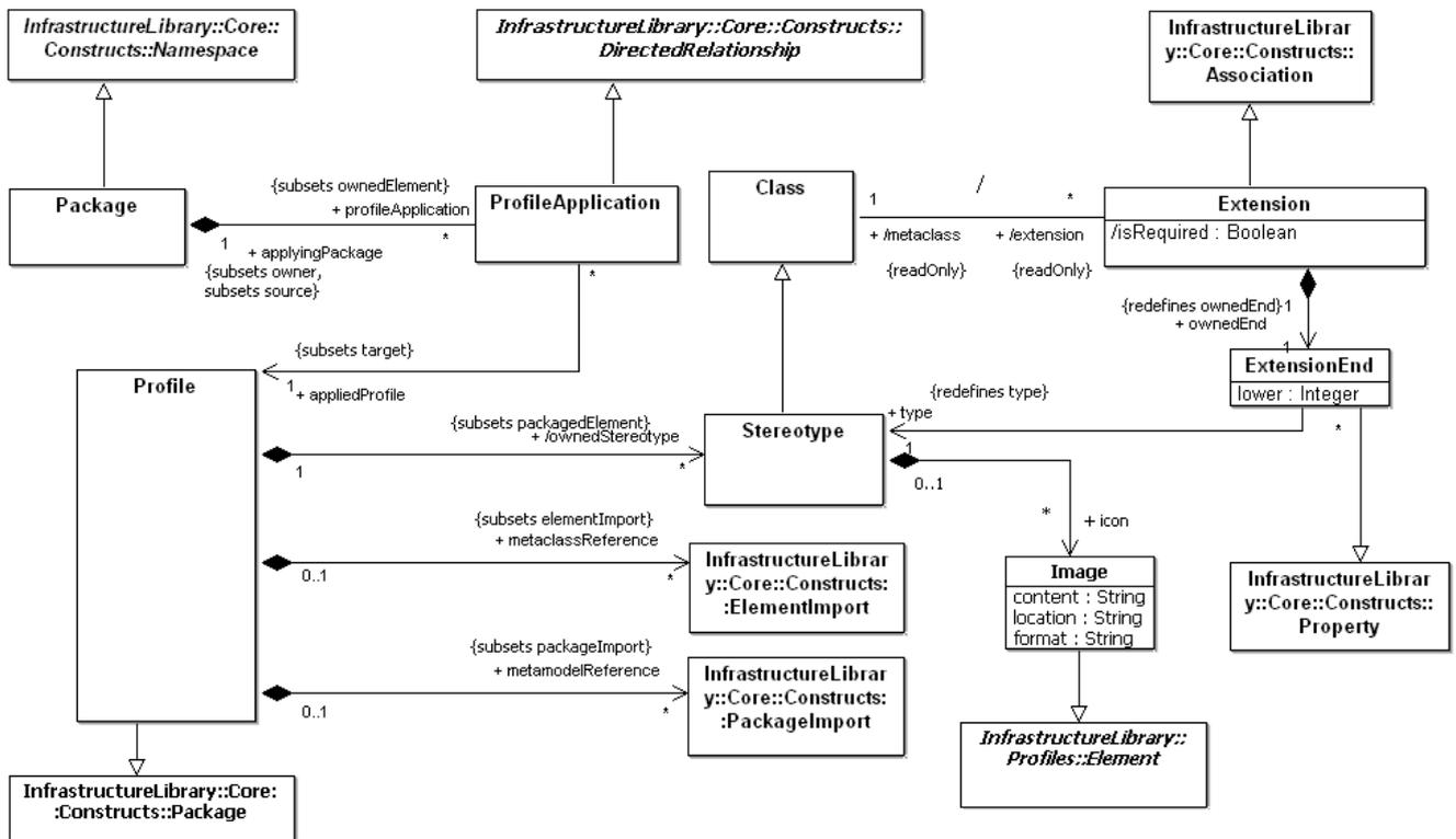
Figure 18.2 - The elements defined in the Profiles package
