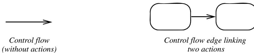
Figure 12.70 - Control flow notation
