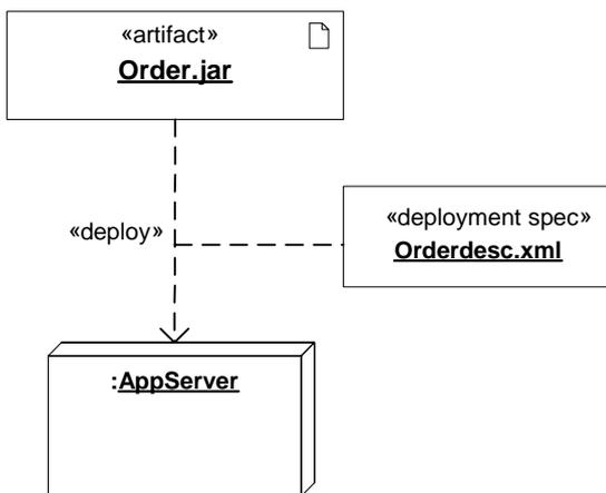
Figure 10.13 - A DeploymentSpecification for an artifact
