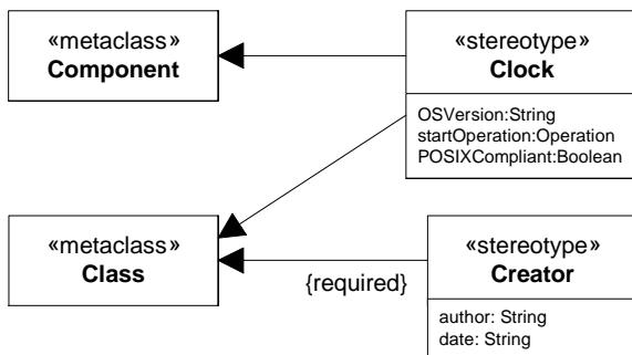
**Figure 18.16 - Defining multiple stereotypes on multiple stereotypes**
