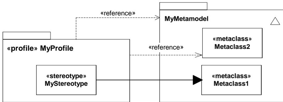
**Figure 18.8 - Specification of an accessible metaclass**
