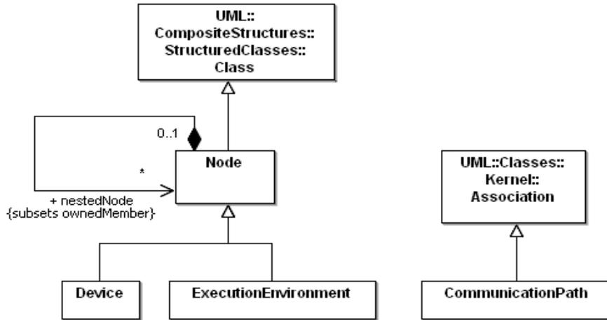
Figure 10.3 - The definition of the Node concept
