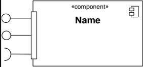
A rectangular box representing a component. Inside the box, the text «component» is at the top, followed by the word <b>Name</b> . On the left side, there are three semi-circular shapes representing required ports. On the right side, there is a small square with a vertical line extending upwards, representing a provided interface.       | See “Port”       |
