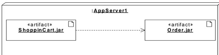
**Figure 10.18 - A set of deployed component artifacts on a Node**
