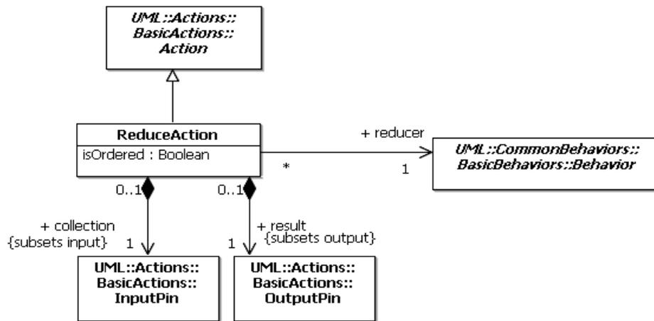
Figure 11.17 - ReduceAction (CompleteActions)
