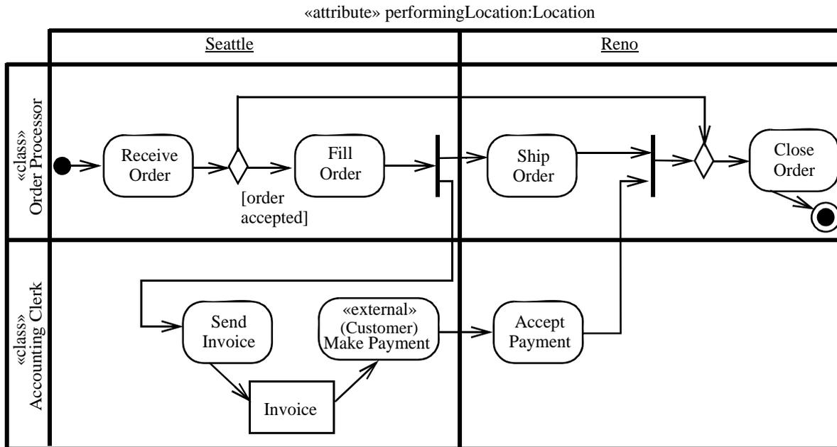
Figure 12.61 - Activity partition using multidimensional swimlane example
