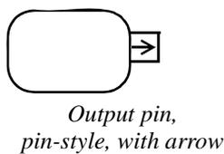
**Figure 12.124 - Pin notations, with arrows**
