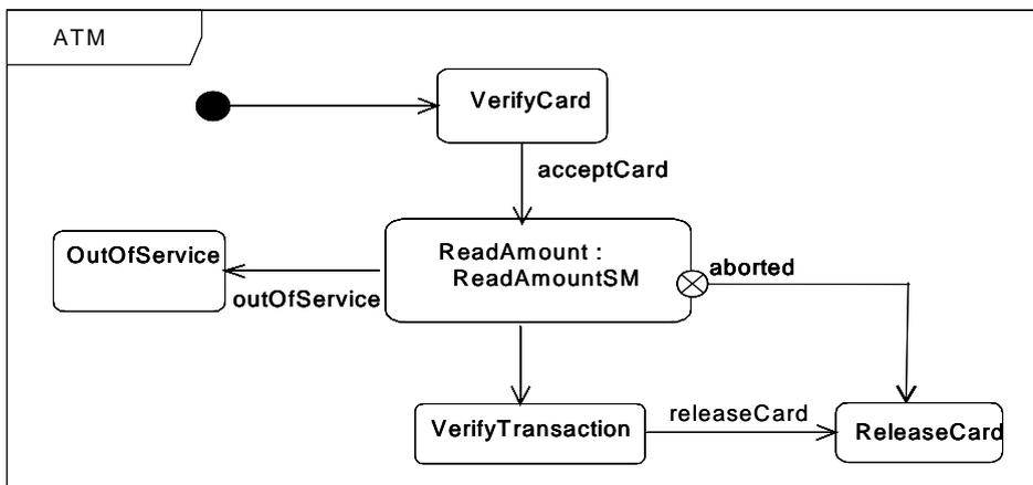
Figure 15.48 - SubmachineState with usage of exit point
