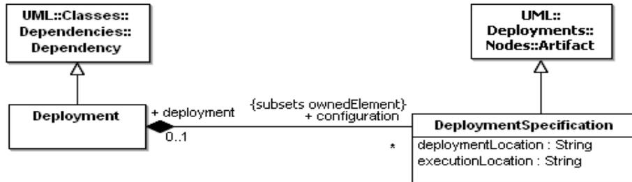
Figure 10.5 - Metaclasses that define component Deployment
