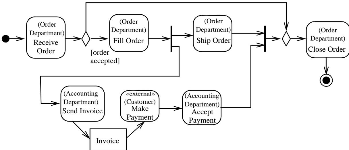
Figure 12.60 - Activity partition using annotation example
