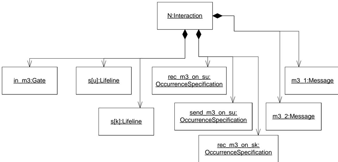
Figure 14.23 - Metamodel elements of a sequence diagrams
