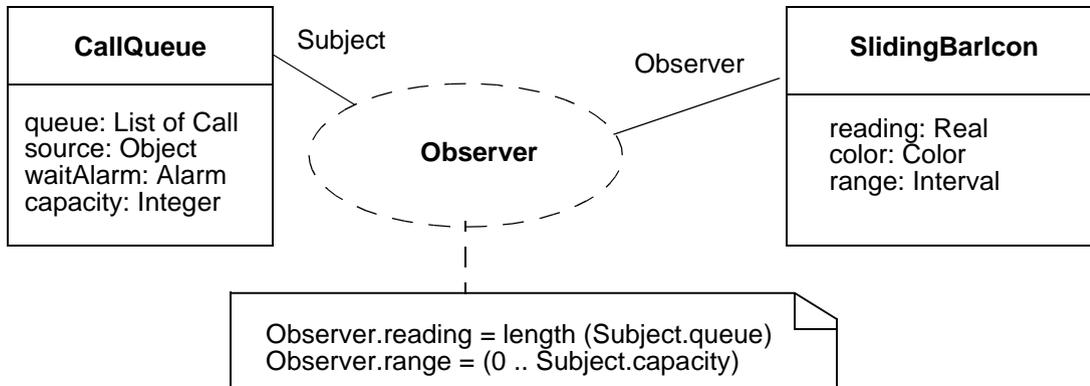
**Figure 9.12 - In the Observer collaboration two roles, a Subject and an Observer, collaborate to produce the desired behavior. Any instance playing the Subject role must possess the properties specified by CallQueue, and similarly for the Observer role.**
