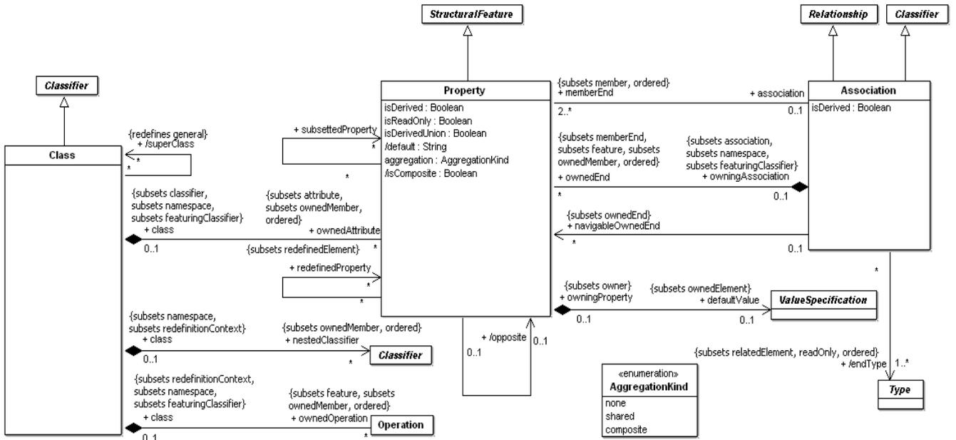
Figure 7.12 - Classes diagram of the Kernel package
