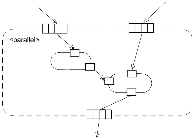
**Figure 12.86 - Expansion region with 2 inputs and 1 output**
