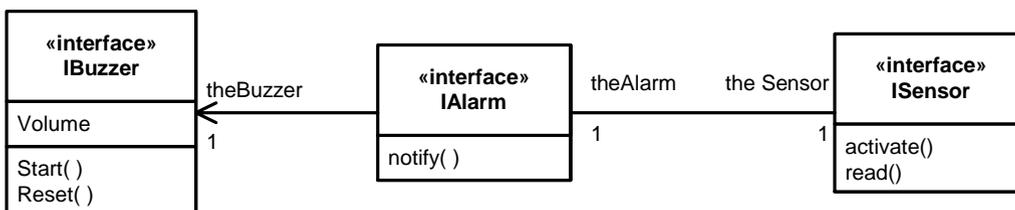
Figure 7.59 - A set of collaborating interfaces
