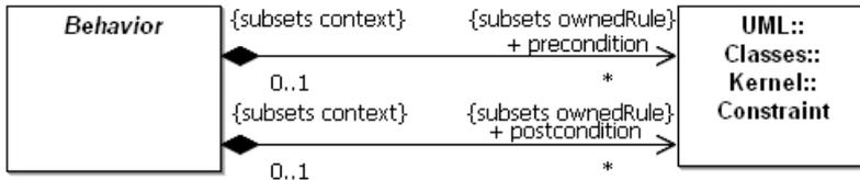
Figure 13.8 - Precondition and postcondition constraints for behavior
