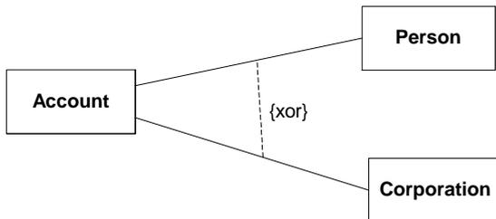
Figure 7.34 - {xor} constraint
