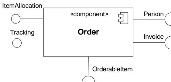
**Figure 8.6 - A Component with two provided and three required interfaces**
