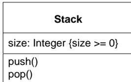
Figure 7.33 - Constraint attached to an attribute
