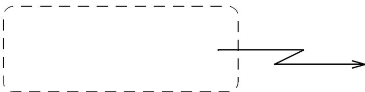
Figure 12.98 - `InterruptibleActivityRegion` notation with interrupting edge
