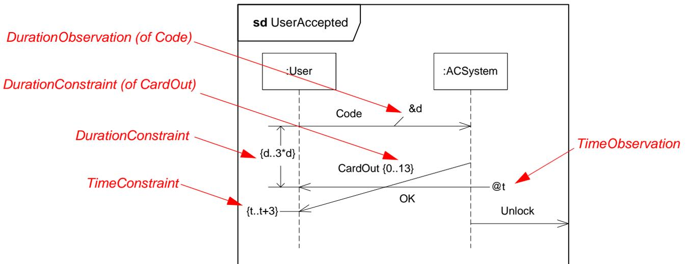
Figure 13.15 - DurationConstraint and other time-related concepts
