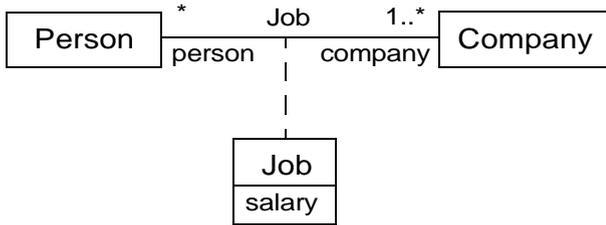
**Figure 7.27 - An AssociationClass is depicted by an association symbol (a line) and a class symbol (a box) connected with a dashed line. The diagram shows the association class Job, which is defined between the two classes Person and Company.**
