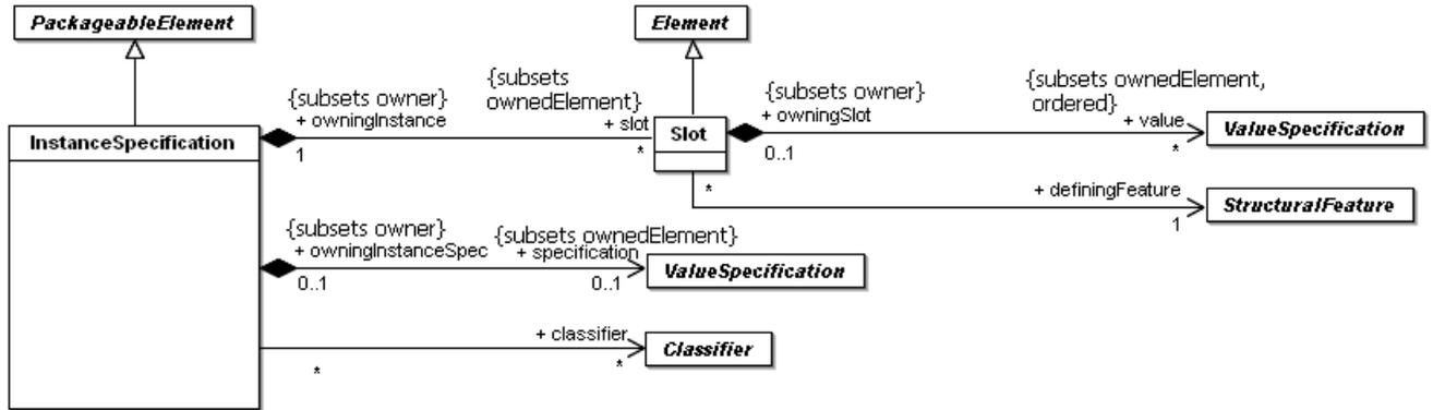
Figure 7.8 - Instances diagram of the Kernel package
