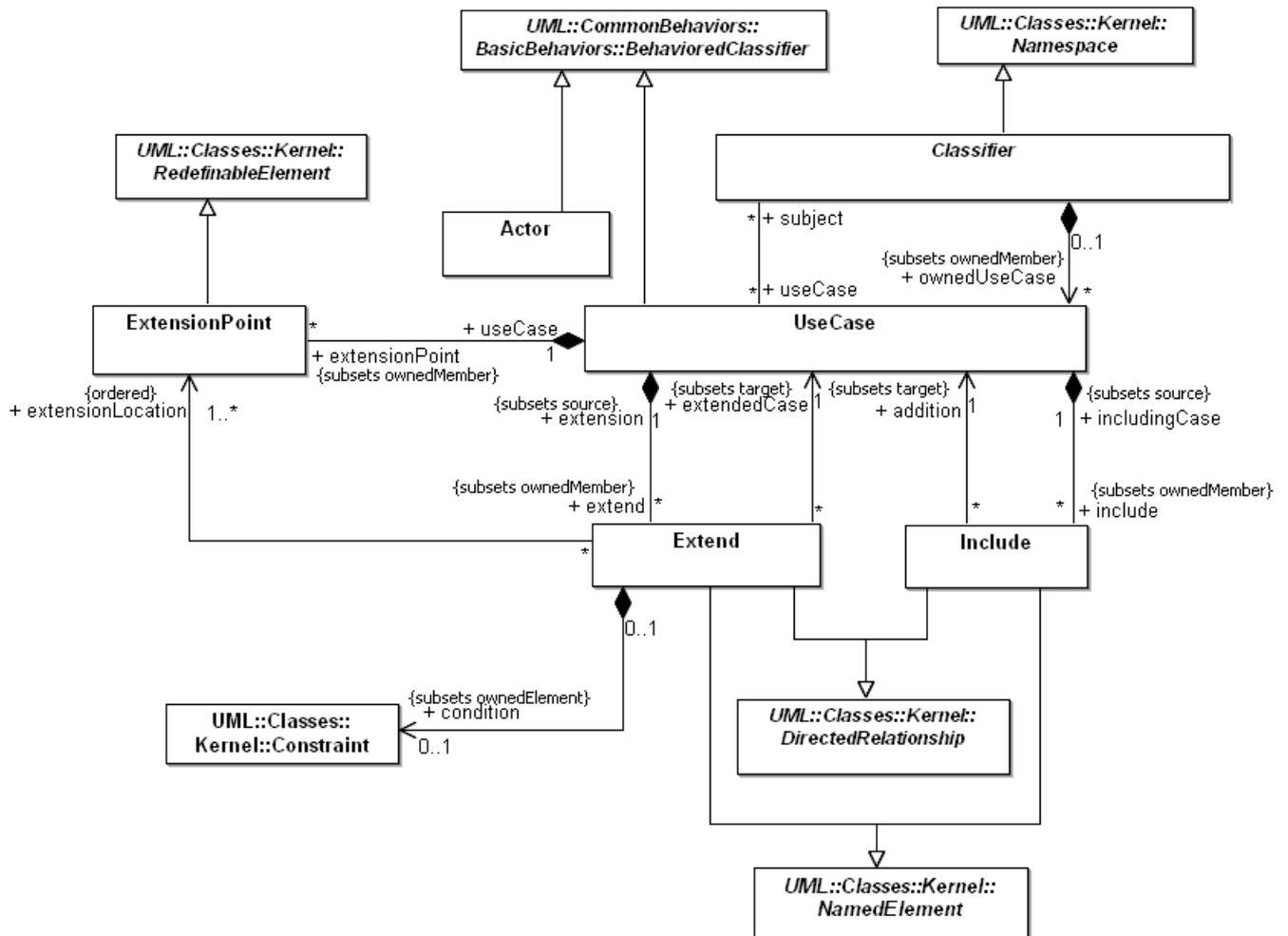
Figure 16.2 - The concepts used for modeling use cases
