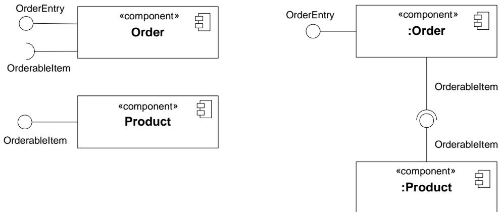
**Figure 8.17 - An assembly connector maps a required interface of a component to a provided interface of another component in a certain context (definition of components, e.g., in a library on the left, an assembly of those components on the right).**
