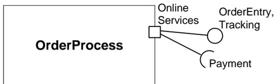
**Figure 9.18 - Port notation showing multiple provided interfaces**
