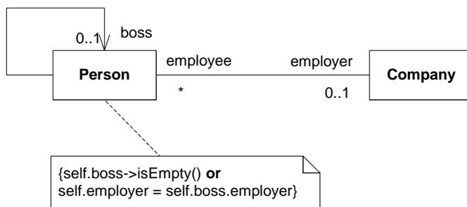
Figure 7.35 - Constraint in a note symbol
