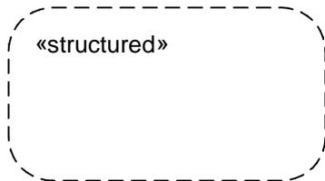
**Figure 12.133 Notation for structured nodes**
