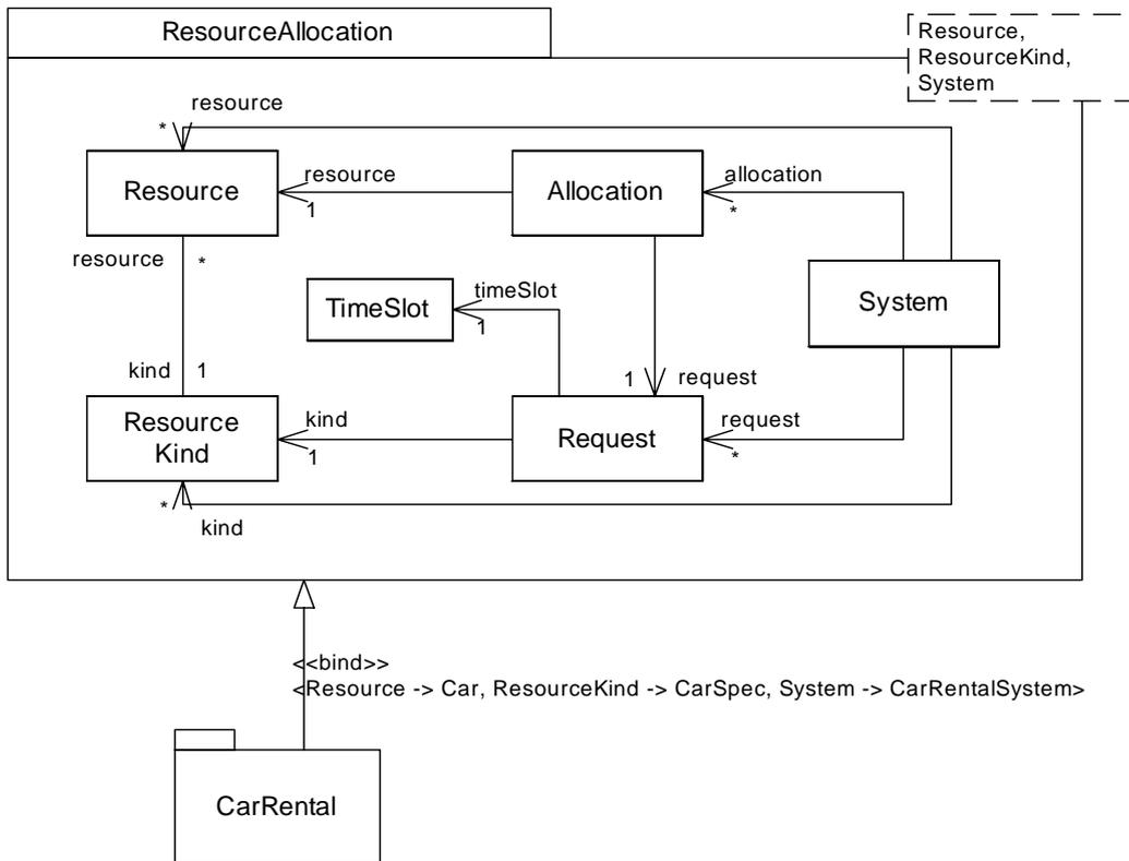
Figure 17.26 - Template Package and Bound Package
