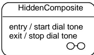
Figure 15.34 - Composite State with hidden decomposition indicator icon
