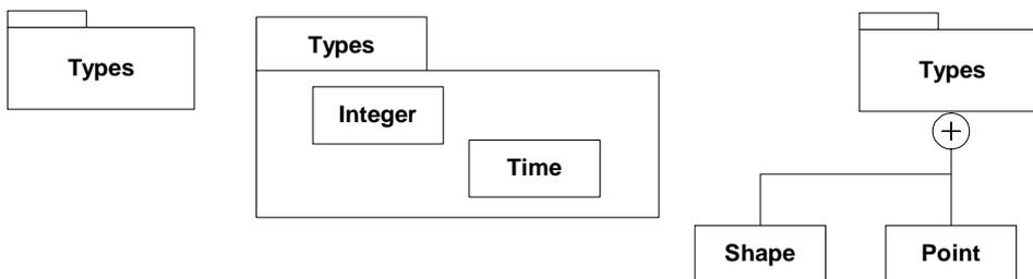
Figure 7.63 - Examples of a package with members
