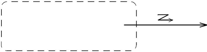
Figure 12.99 - InterruptibleActivityRegion notation with interrupting edge
