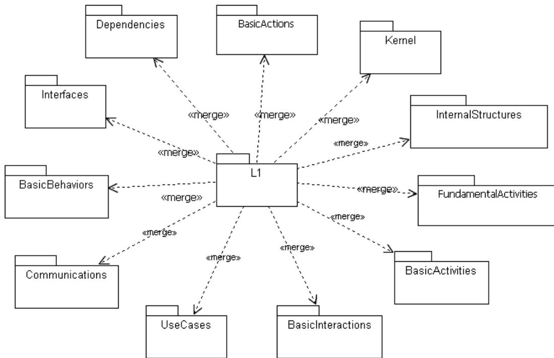
**Figure 2.2 - Level 1 top-level package merges**
