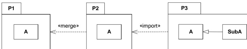
**Figure 7.65 - Illustration of the meaning of package merge**
