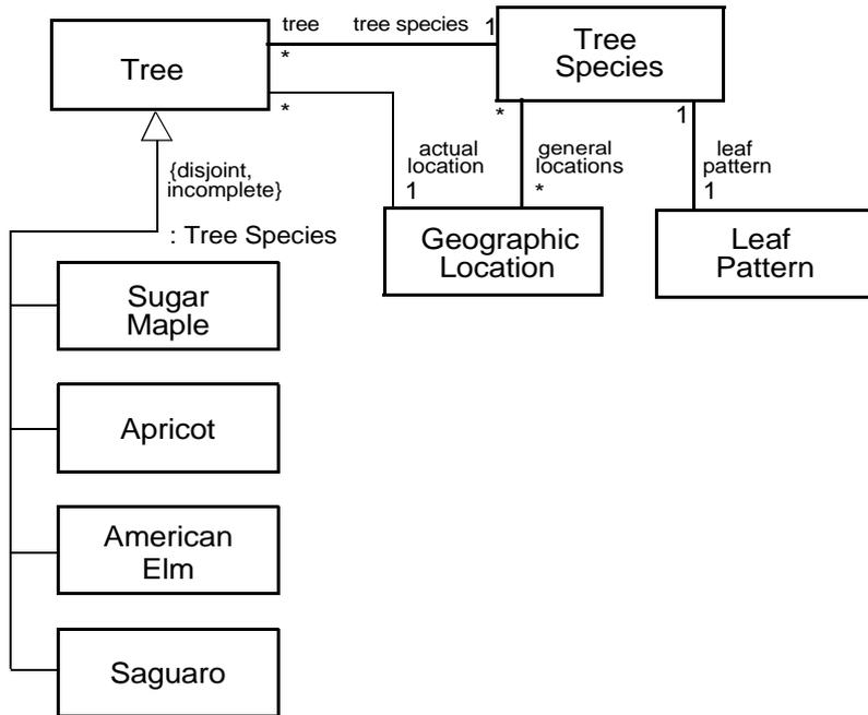
**Figure 7.49 - Power type example and notation**
