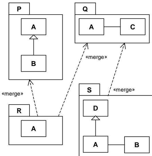
Figure 7.68 - Simple example of package merges
