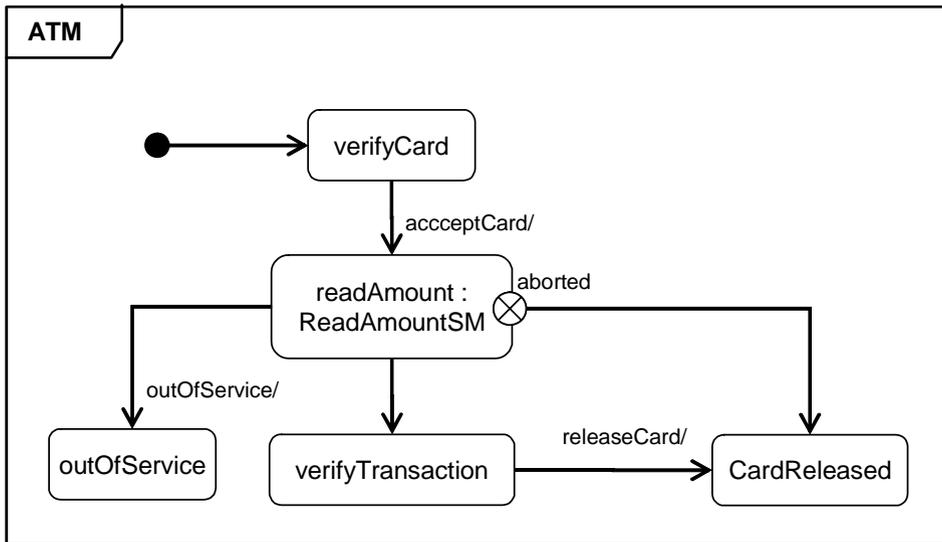
**Figure 15.39 - SubmachineState with usage of exit point**
