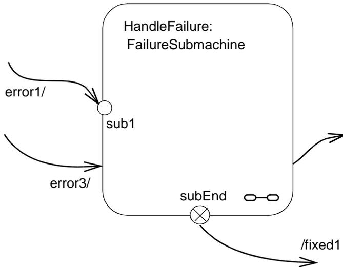
**Figure 15.36 - Submachine State**
