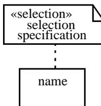
**Figure 12.116 - Specifying selection behavior on an Object node**
