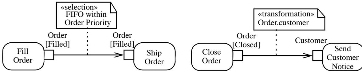
Figure 12.112 - Specifying selection behavior on an Object flow
