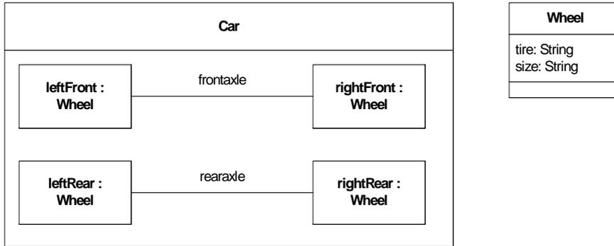
**Figure 9.24 - Connectors and parts in a structure diagram**
