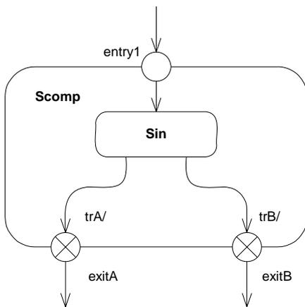
**Figure 15.21 - Entry and exit points on composite states**
