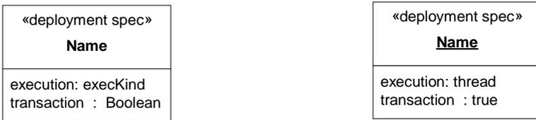
Figure 10.11 - DeploymentSpecification for an artifact (specification and instance levels)
