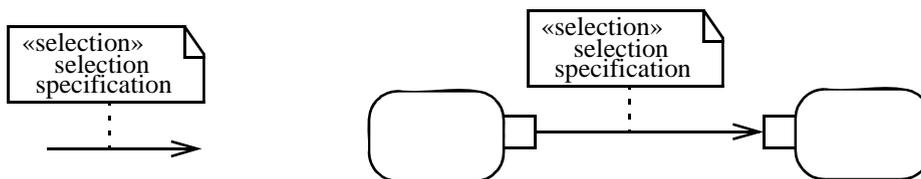
**Figure 12.108 - Specifying selection behavior on an Object flow**
