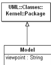
Figure 17.8 - The contents of the Models package
