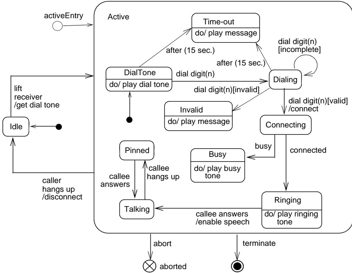
Figure 15.41 - State machine diagram representing a state machine
