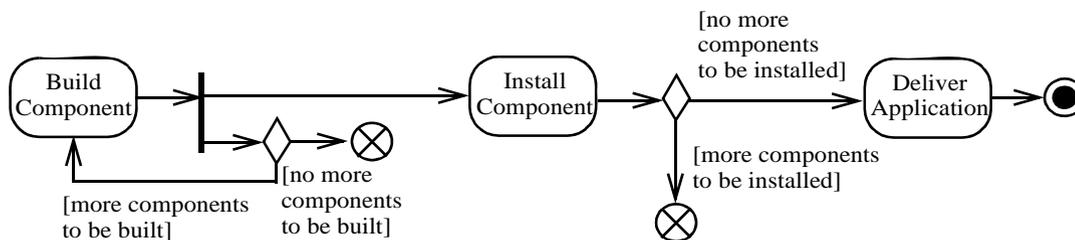
Figure 12.91 - Flow final and activity final example
