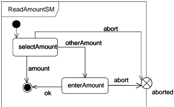
Figure 15.47 - State machine with exit point definition
