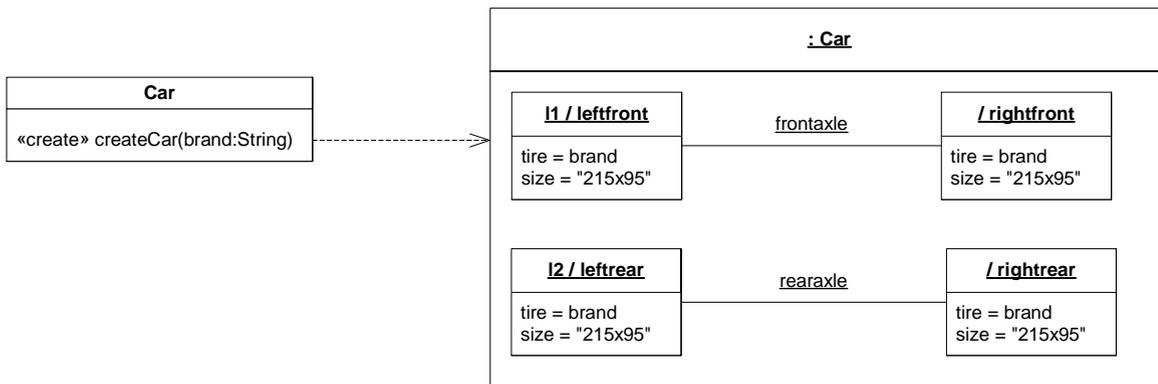
Figure 9.27 - A constructor for the Car class
