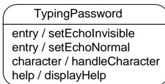
**Figure 15.32 - State with compartments**
