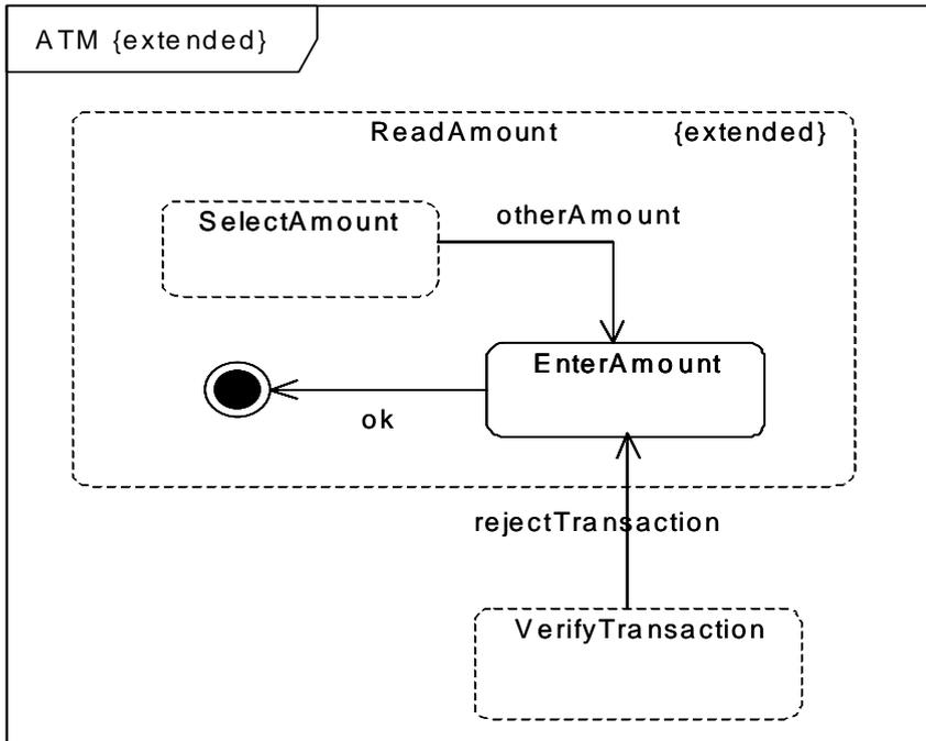
Figure 15.43 - An extended state machine
