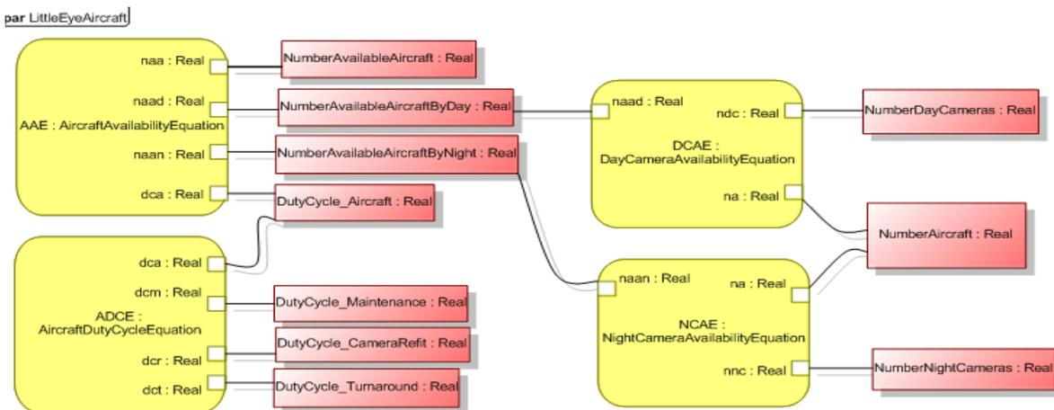
Figure D.51 - Aircraft System Parametric
