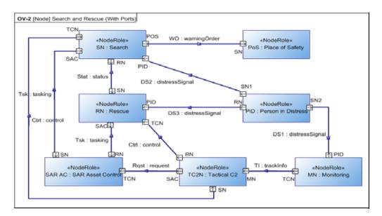
Figure D.17 - Alternate OV-2 with SysML Flow Ports
