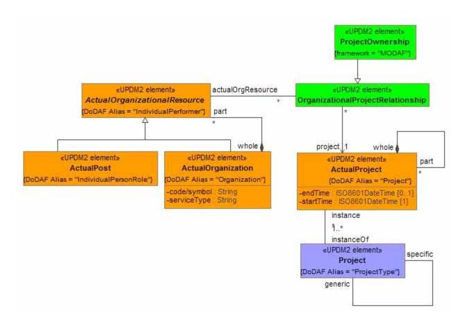
Figure A.1 - AcV-1/PV-1 - DMM
