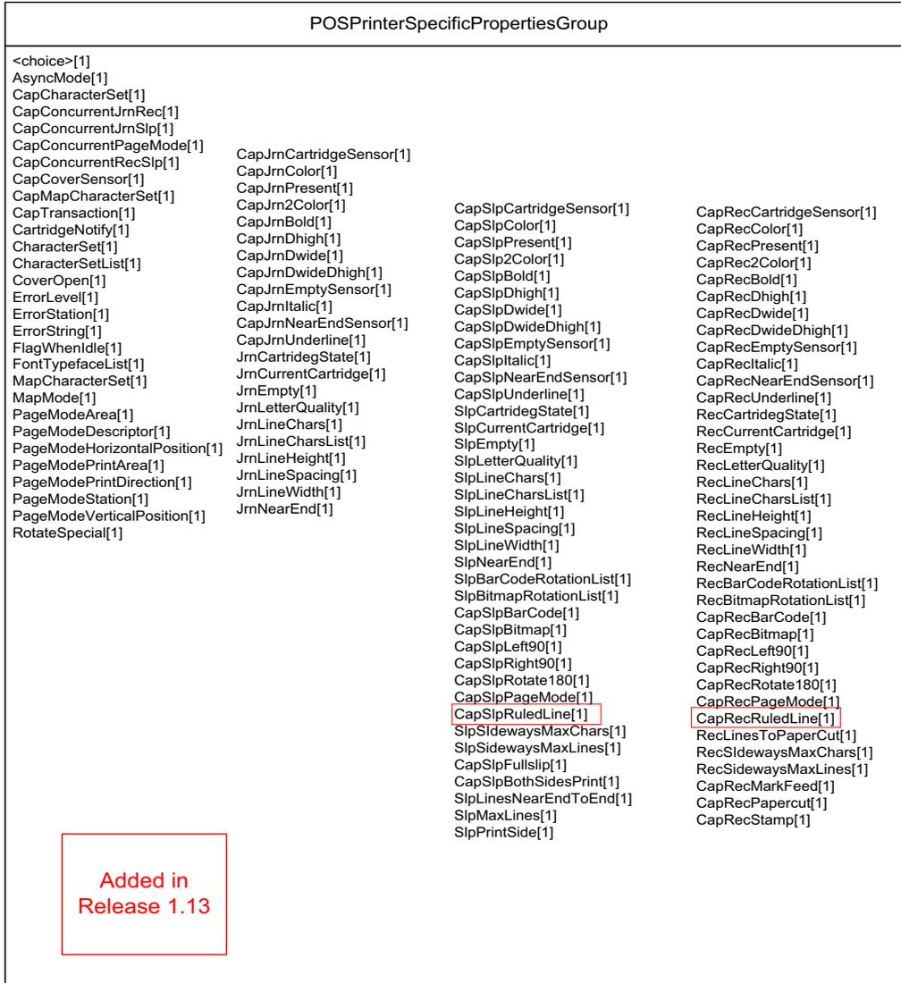
Figure 124: POS Printer Properties Domain View
