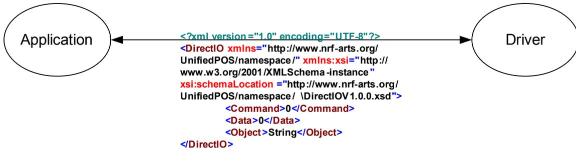
**Figure 1: Synchronous Communications**
