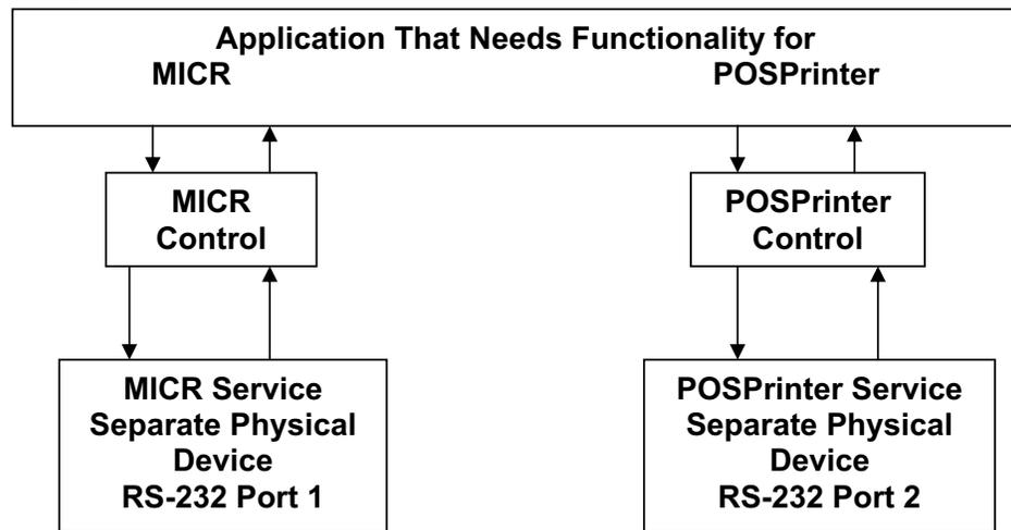
Note that in this case the application running the MICR and the POSPrinter consumes two separate ports but as far as the Application is concerned it interfaces to the MICR and POSPrinter functionality without regard to the fact that the two ports are used.
