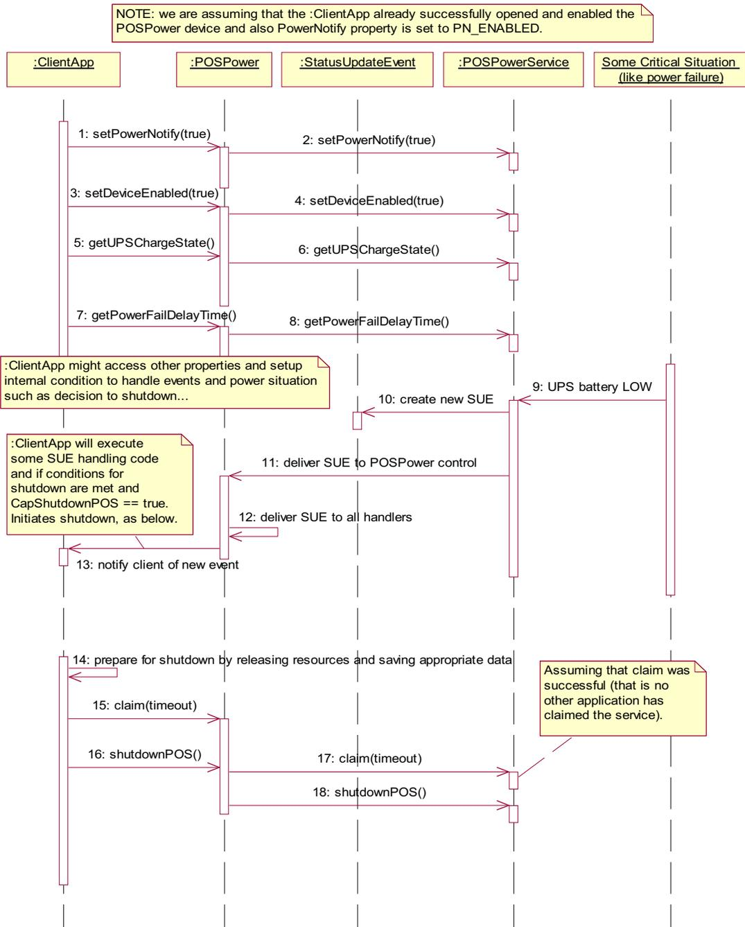
**POSPower Standby Sequence Diagram** *Added in Release 1.9*
