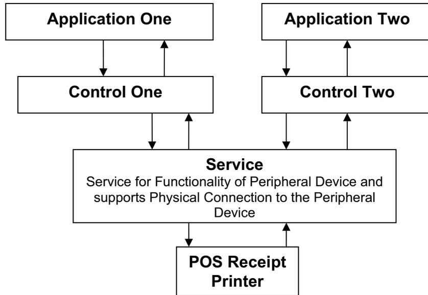
Note, that as far as each application is concerned, it is connected to the peripheral device and only one physical connection to the device is required... via the RS-232 serial connection in this example. This served the needs of device sharing where cooperating applications were utilized.
