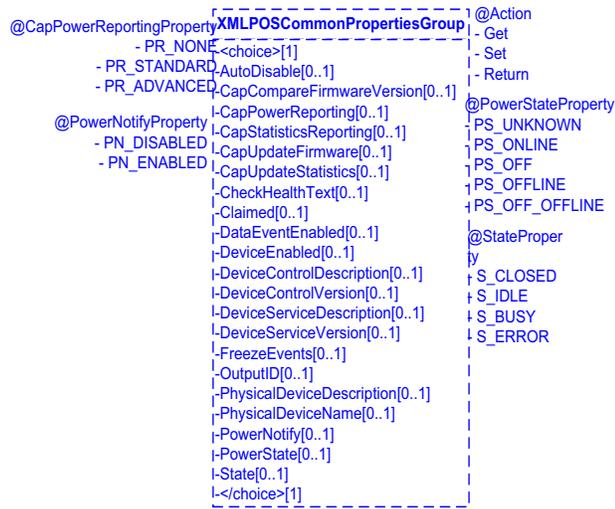
Figure 2: XML Common Properties Schema Architecture Sample
