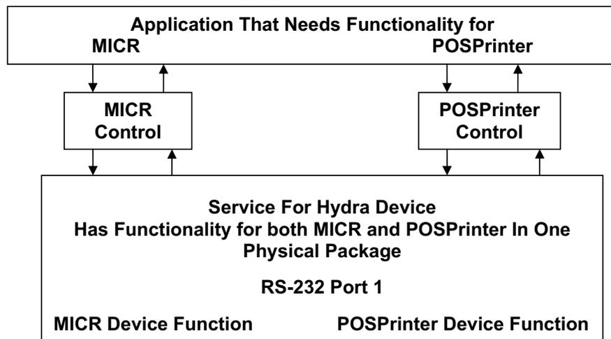
Note that in this case the application running the MICR and POSPrinter consumes only one port but as far as the application is concerned it interfaces to the MICR and POSPrinter functionality without regard to the fact that only one port is used. It is up to the Hydra Service to control the port and route the functionality to and from the proper interface.
