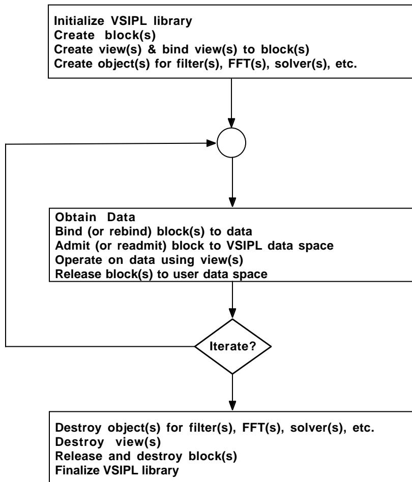
A VSIPL program must initialize the VSIPL library with a call to `vsip_init` before calling any other VSIPL function. Any program that uses VSIPL and that terminates must call `vsip_finalize` before terminating. See the Support chapter for additional conditions and restrictions on these functions.
