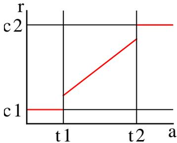
$$r_j = \begin{cases} c_1 & \text{if } a_j \leq t_1 \\ a_j & \text{if } a_j = t_2 \text{ for } j = 0, 1, \dots, N-1 \\ c_2 & \text{otherwise} \end{cases}$$
